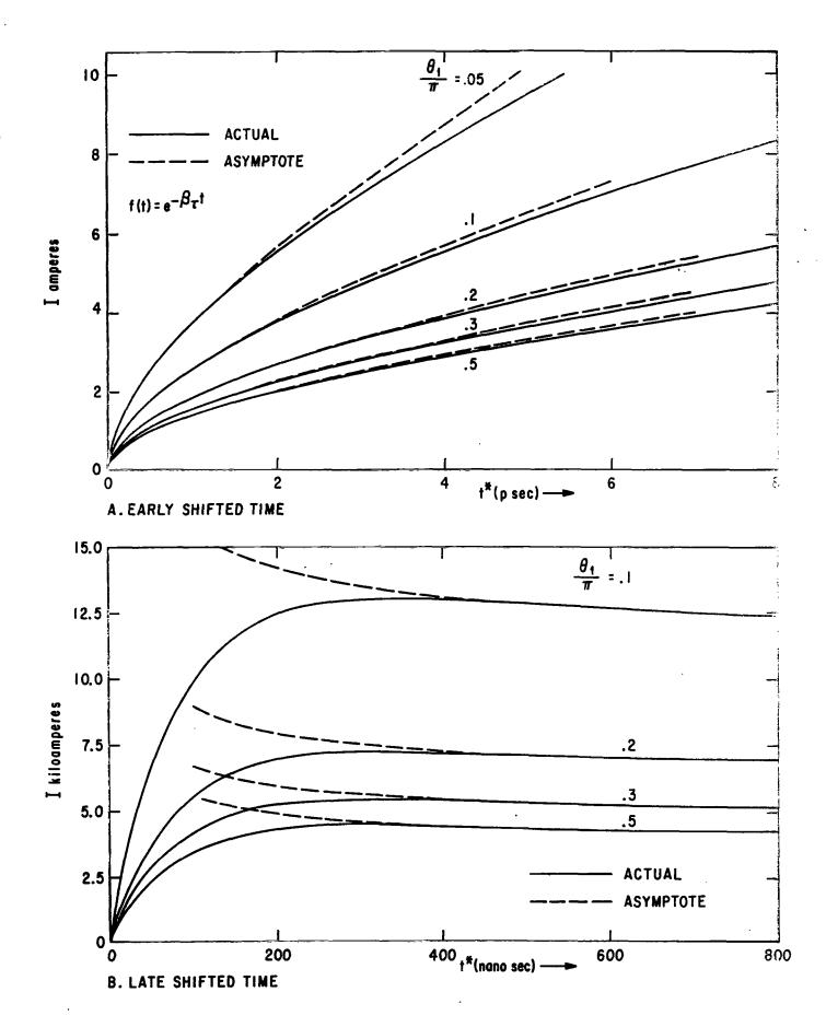
FIGURE 8. AXIAL CURRENT RESPONSE WITH  $\beta_{\tau} = 10^7 \text{sec.}^{-1}$ ,  $Z = 120\pi\Omega$ ,  $\alpha = 3\times10^{-3}\text{m}$ ,  $E_0 = 10^5$  VOLTS PER METER, AND  $\theta_1$  AS A PARAMETER.
