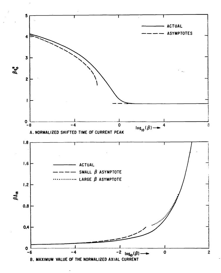
FIGURE 7. NORMALIZED PEAK AXIAL CURRENT RESPONSE TO AN EXPONENTIALLY DECAYING PLANE WAVE.
