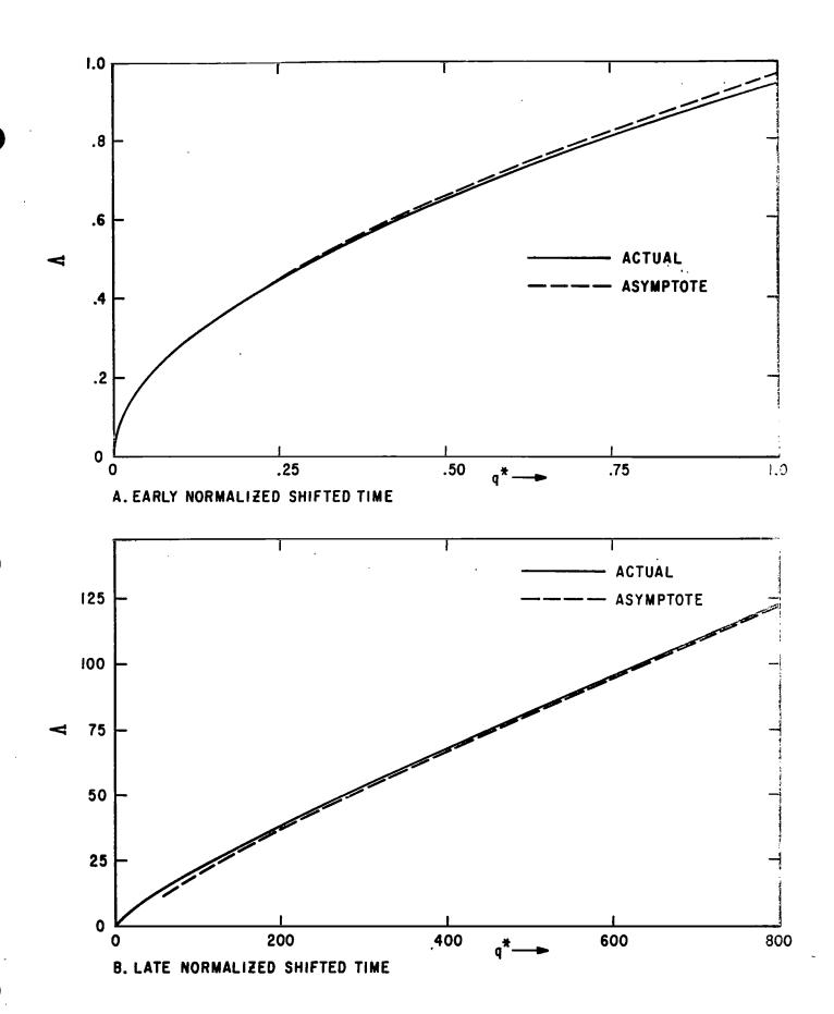
FIGURE 5. NORMALIZED AXIAL CURRENT RESPONSE TO AN INCIDENT PLANE WAVE WITH A STEP-FUNCTION TIME HISTORY.
