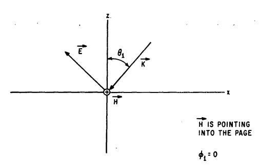
B. MAGNETIC FIELD POLARIZED PERPENDICULAR TO THE z-AXIS
