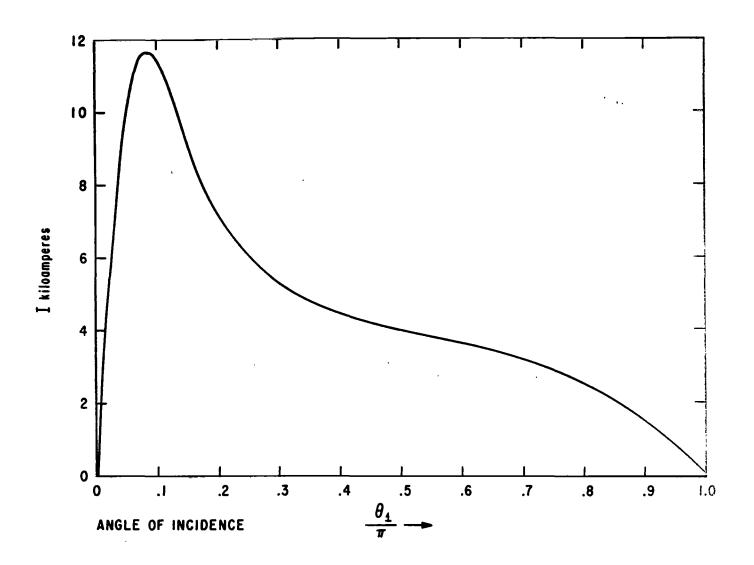
FIGURE 10. AXIAL CURRENT RESPONSE AT  $t^* = t_a^*$  WITH  $\beta_{\tau} = 10^7 \text{sec.}^{-1}$ ,  $a = 3 \times 10^{-3} \text{m}$ ,  $\frac{a_1}{c} = 3 \times 10^{-6} \text{s}$ ,  $\frac{a_2}{c} = 1.5 \times 10^{-7} \text{s}$ ,  $E_0 = 10^5 \text{ V/m}$ , AND  $Z = 120 \pi \Omega$ .
