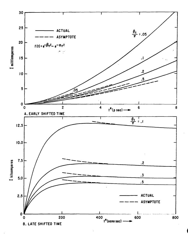
FIGURE 9. AXIAL CURRENT RESPONSE WITH  $\beta_{\tau}$ = 10<sup>7</sup> sec. , Z = 120 $\pi\Omega$ , a = 3 x 10<sup>-3</sup> m,  $\alpha_{\tau}$ = 5 x 10<sup>8</sup> sec. , E<sub>0</sub>= 10<sup>5</sup> V/m, AND  $\underline{\theta_{1}}$  AS A PARAMETER.
