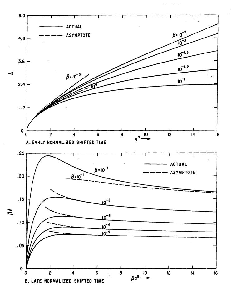
FIGURE 6. NORMALIZED AXIAL CURRENT RESPONSE TO AN EXPONENTIALLY DECAYING PLANE WAVE WITH  $oldsymbol{eta}$  AS A PARAMETER.
