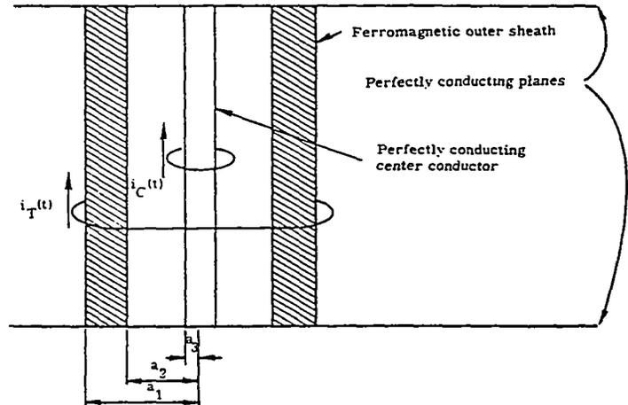
Fig. 1. Model coaxial cable.
