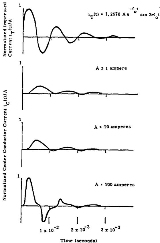
Fig. 3. Normalized center conductor current for a damped sine wave impressed current  $f_0 = 1$  kHz.
