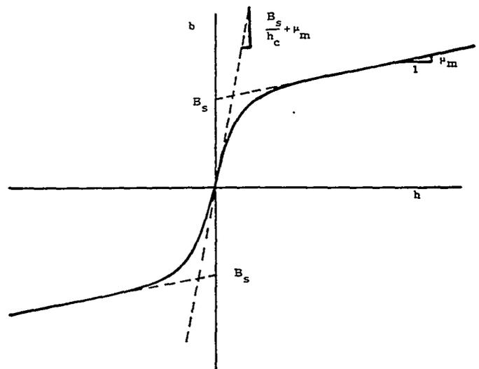
Fig. 2. Magnetic characteristics of ferromagnetic material.
