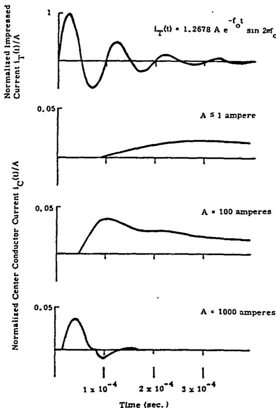
Fig. 4. Normalized center conductor current for a damped sine wave impressed current  $f_0 = 10$  kHz.
