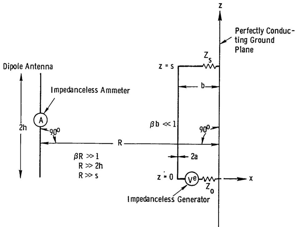
Figure 5. Single Conductor with Terminating Impedances Grounded to a Perfectly Conducting Plane as a Transmitting Antenna
