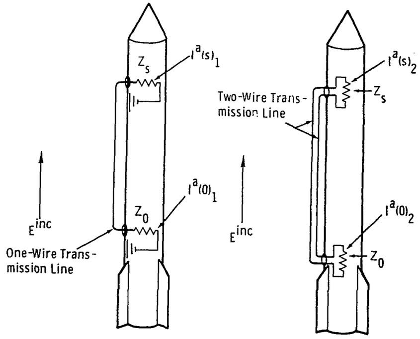
Figure 1. Rockets with External Cables
