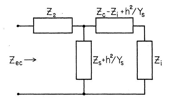
Figure 2. Network representation of the external coupling impedance per unit length
