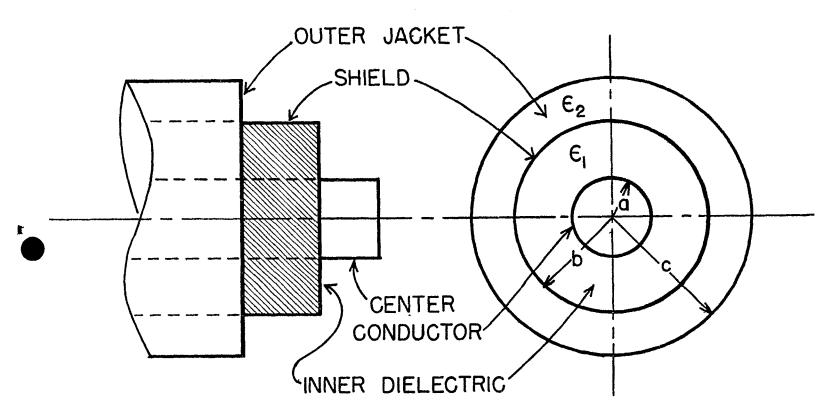
Figure 1. Geometry of the general coaxial cable model
