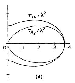
Fig. 6. Transmission cross sections for a square aperture of side length L, excited by a plane wave with H in the xz plane and incident at an angle  $\theta$  from the normal direction in the H plane. (a)  $L = \lambda/4$ ,  $\theta = 0$ . (b)  $L = \lambda/4$ ,  $\theta = 45^{\circ}$ . (c)  $L = \lambda/2$ ,  $\theta = 0$ . (d)  $L = \lambda/2$ ,  $\theta = 45^{\circ}$ .
