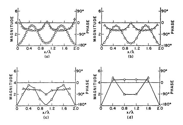
Fig. 5. Magnitude and phase of |M/F<sup>i</sup>|, where M is the x-directed magnetic current and E<sup>i</sup> is the incident electric field, when the number of expansion functions is (a) 39, (b) 19, (c) 9, and (d) 4. Circles denote magnitude, triangles denote phase. Computations are for the same slot as for Fig. 4.
