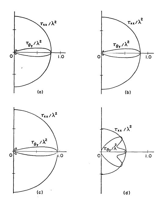
Fig. 4. Transmission cross section when the number of expansion functions is (a) 39, (b) 19, (c) 9, and (d) 4. Computations are for a slot of length  $2\lambda$  in the x direction and width  $\lambda/10$  in the y direction. Excitation is by a plane wave normally incident on the conducting plane with magnetic field in the x direction.
