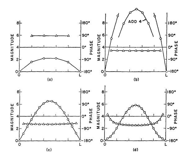
Fig. 3. Magnitude and phase of  $|M/E^i|$ , where M is the x-directed magnetic current and  $E^i$  is the incident electric field, for the same slots as for Fig. 2. (a)  $L = \lambda/4$ , (b)  $L = \lambda/2$ , (c)  $L = 3\lambda/4$ , (d)  $L = \lambda$ . Circles denote magnitude, triangles denote phase.
