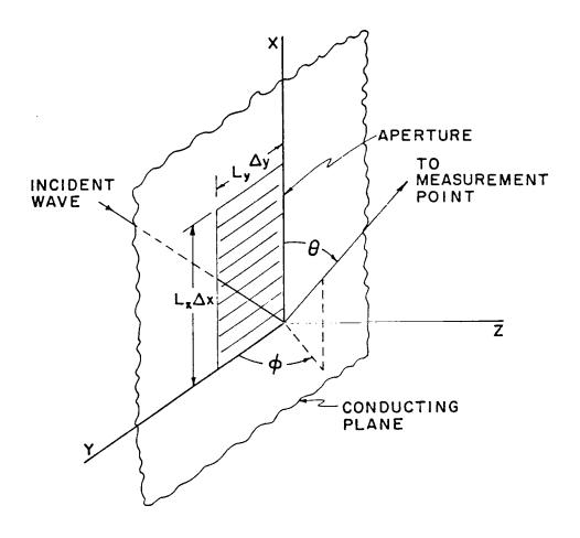
Fig. 1. Rectangular aperture in a conducting plane.
