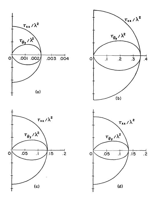
Fig. 2. Transmission cross section for slots of length L in the x direction and width  $\lambda/20$  in the y direction. (a) L =  $\lambda/4$ , (b) L =  $\lambda/2$ , (c) L =  $3\lambda/4$ , (d) L =  $\lambda$ . Excitation is by a plane wave normally incident on the conducting plane with magnetic field in the x direction.
