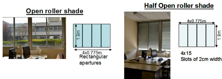
Figure 11 - Office-room windows and roller shade configurations
