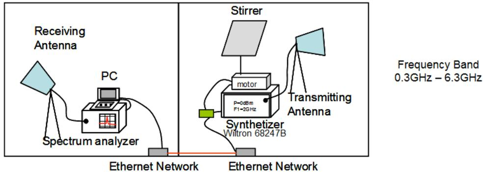
Figure 4 - Test set-up for transfer function measurements in a building
