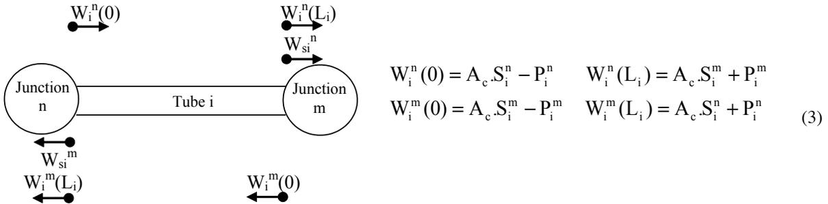
Figure 15 – Definition of waves on a tube in EMT/PWB formalism
