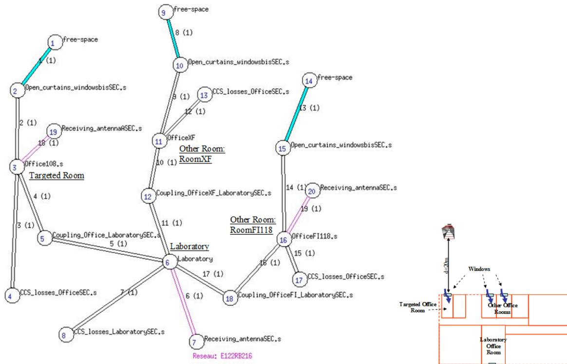
Figure 16 - EMT/PWB network model of the illumination configuration of ONERA's targeted building
