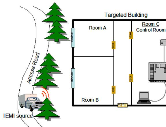
Figure 1 – IEMI/NNEMP attack of a building from outside
