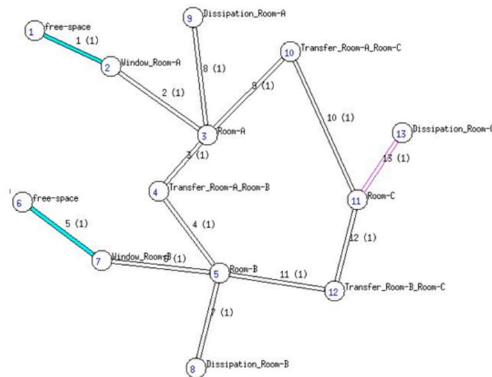
Figure 14: EMT/PWB network of the simple building
