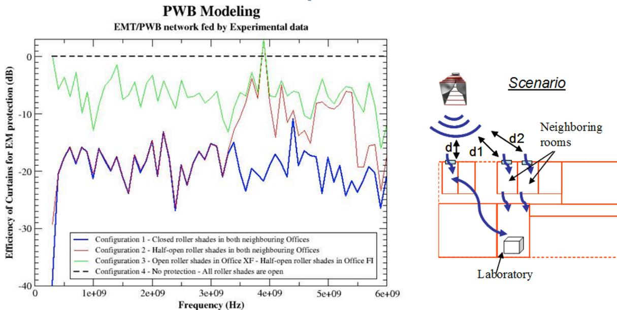
Figure 20 – Attenuation brought in the laboratory room by other rooms metallic roller shades
