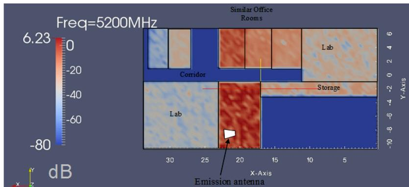
Figure 9 - Attenuation between an emission room and other neighbouring rooms in the targeted building (blue zones correspond to zones for which no measurement is available)
