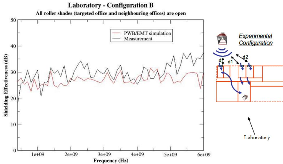
Figure 19 - Shielding effectiveness of the laboratory room – configuration B
