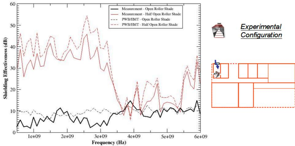
Figure 17 - Shielding effectiveness of targeted office – simulation and measurement – Horizontal polarization
