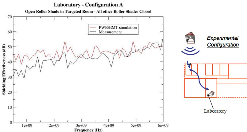
Figure 18 - Shielding effectiveness of laboratory room – configuration A
