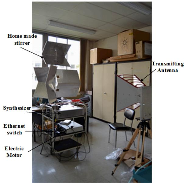
Figure 5 - Transmitting equipment in building room at emission side
