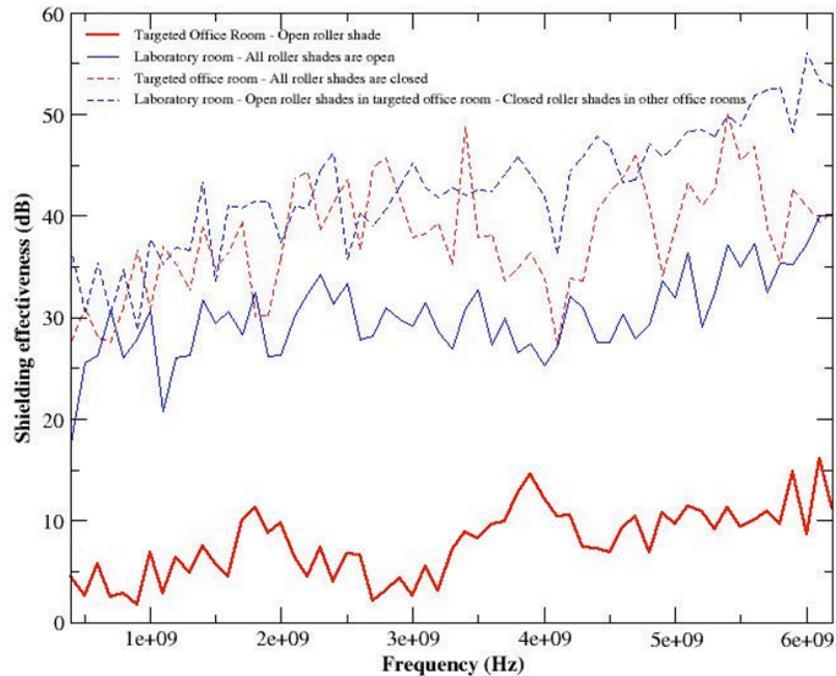
Figure 13 - Shielding effectiveness of targeted office and laboratory rooms for several open-closed configurations of office windows
