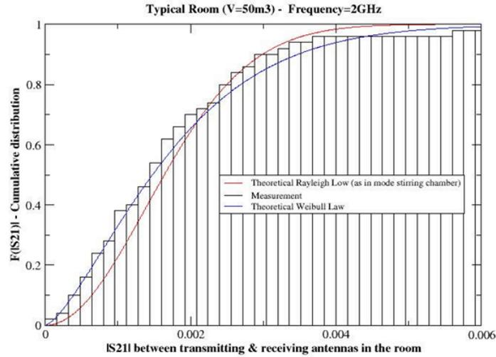
Figure 7 - Example of cumulative distribution obtained from “Intra” configuration measurements in a typical room of ONERA’s building
