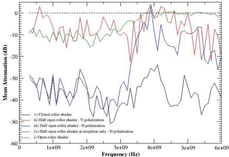
Figure 12 - Effects of metallic roller shades onto building attenuation in the targeted building room
