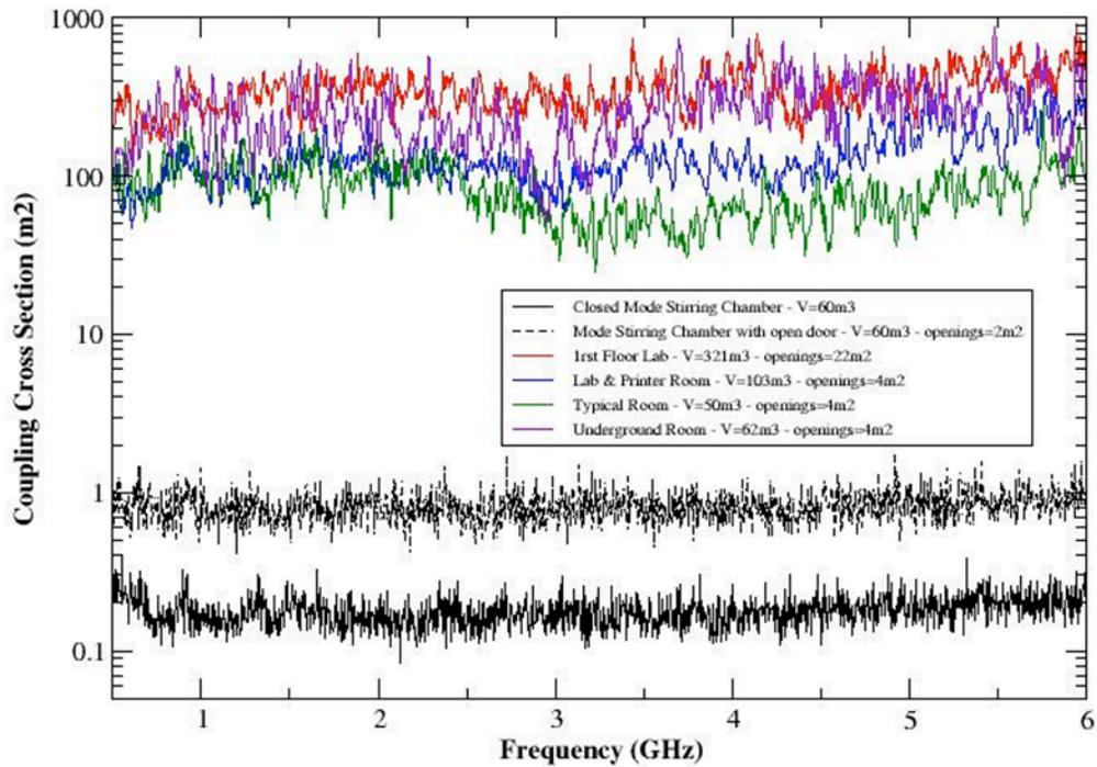
Figure 8 - Equivalent mean Coupling Cross-Sections of different rooms in the targeted building
