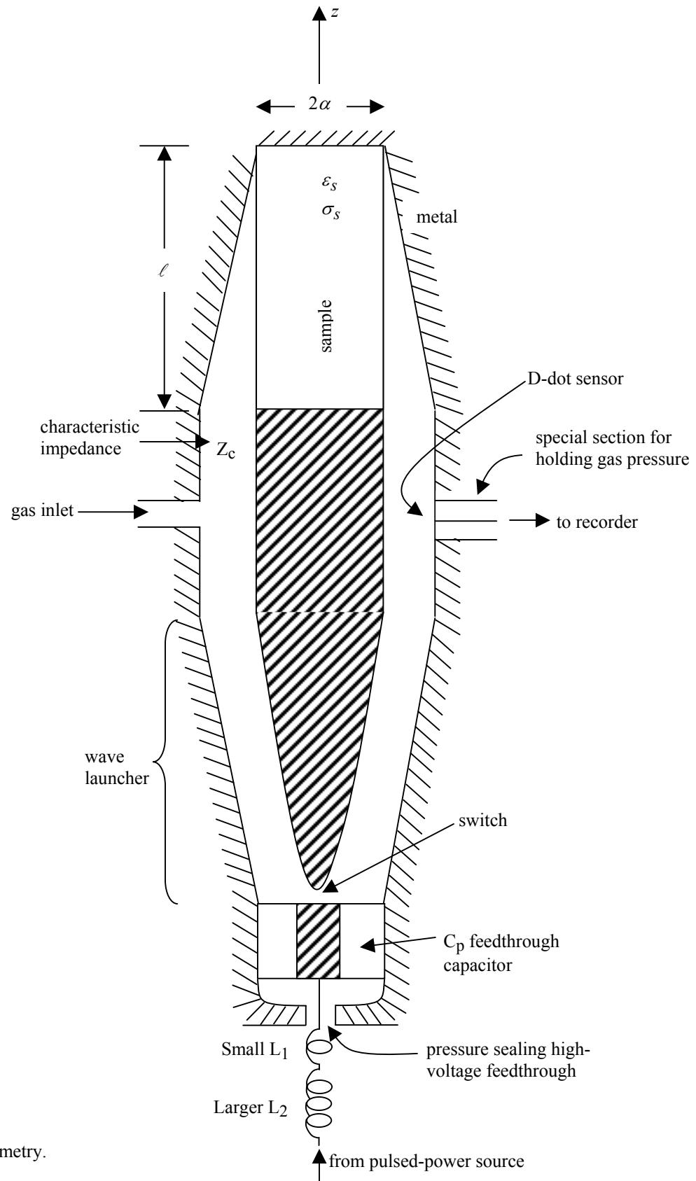
Fig. 2.1 Test-Cell Geometry.
