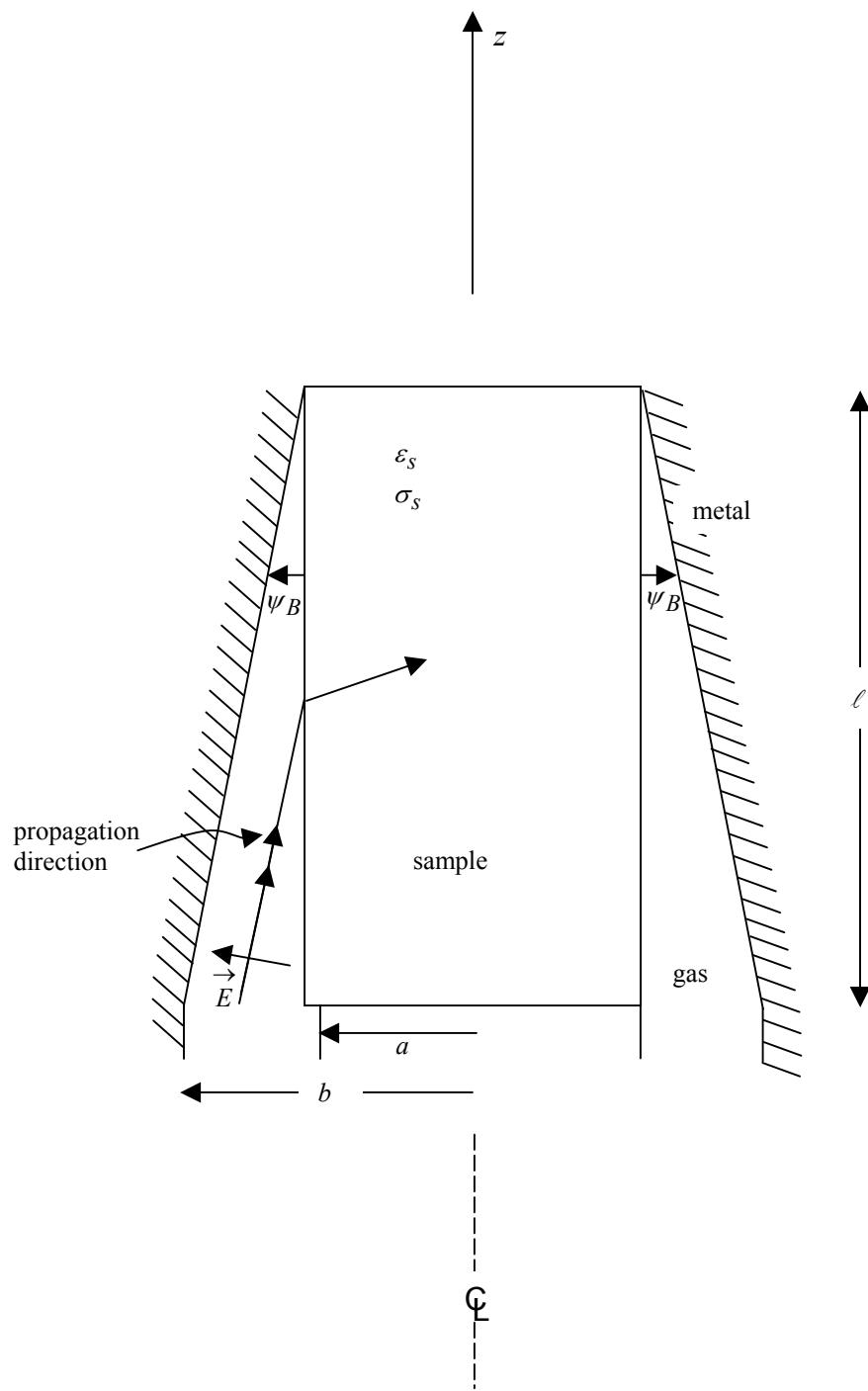
Fig. 3.1 Brewster-Angle Matching of Wave Into Test Sample
