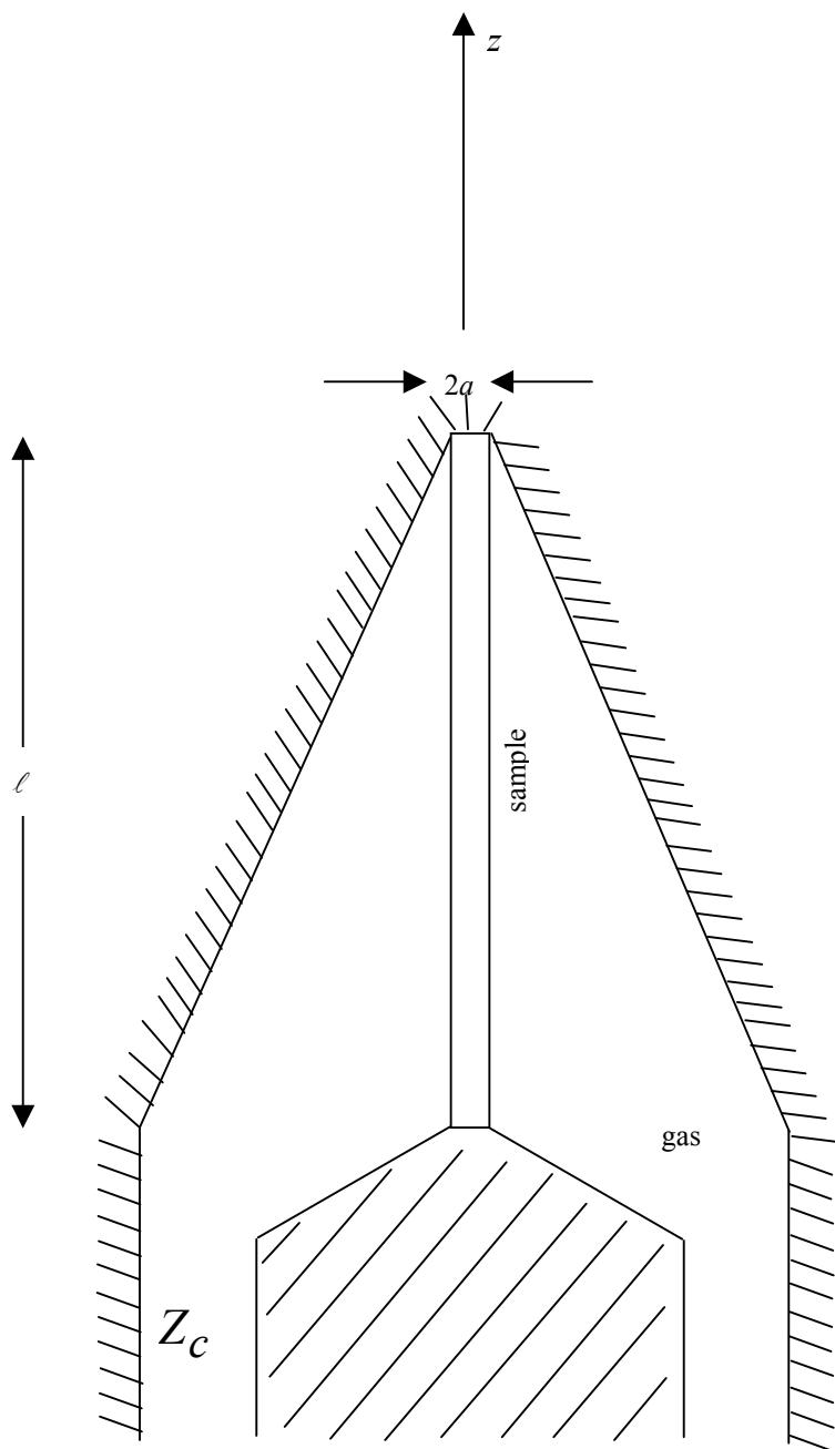
Fig. 3.2 Test-Sample Configuration for Small Sample Radius.
