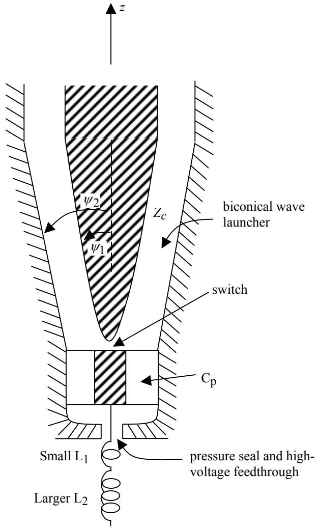
Fig. 4.1 Launching Wave Toward Test Sample
