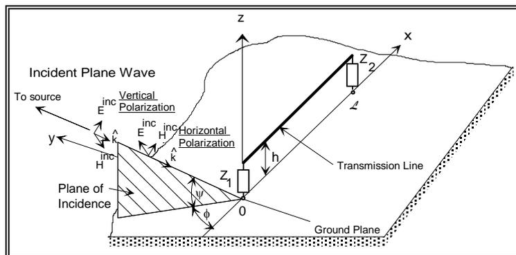
Figure B-2. A single-wire line over a perfectly conducting ground excited by an incident plane wave.
