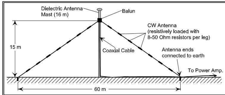
a. Horizontally polarized antenna (EMTECH)
