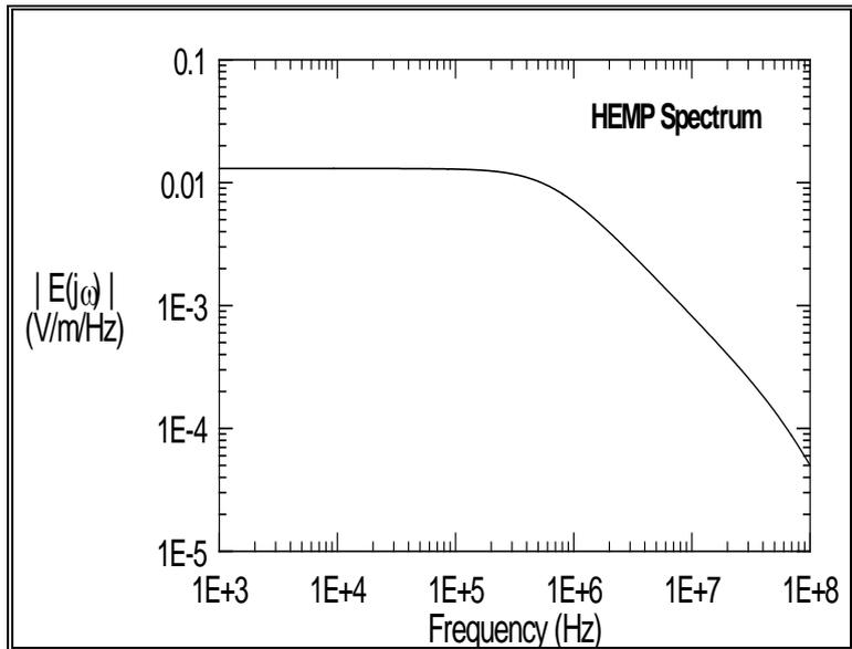
Figure 3. Frequency response of HEMP waveform.
