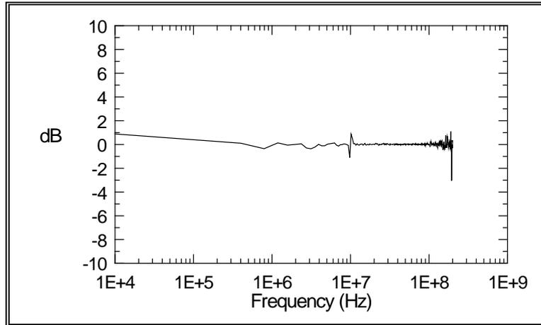
Figure 24. Measured transfer function, corrected by calibration file.
