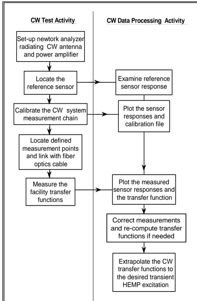
Figure 19. Test and analysis procedures for conducting a CW test.
