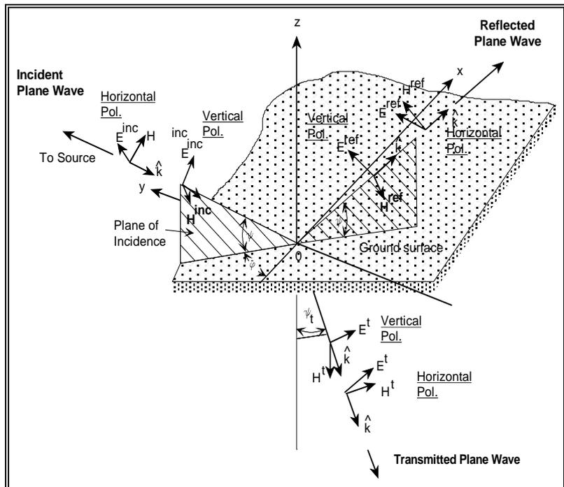
Figure 4. Incident, reflected and transmitted plane waves for  $E_1$ .
