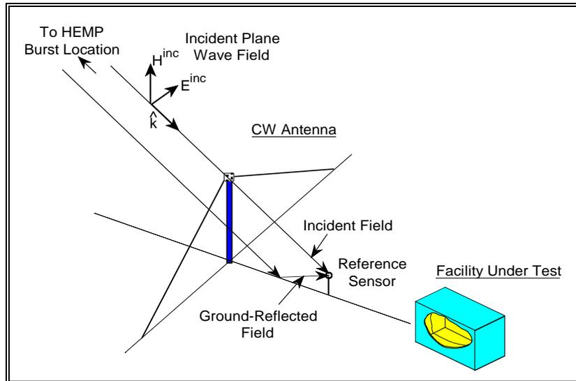
Figure 21. Incident and ground-reflected field contributions to the reference sensor excitations.
