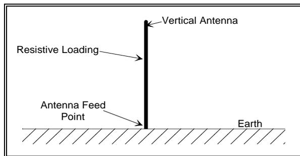
b. Vertically polarized antenna
