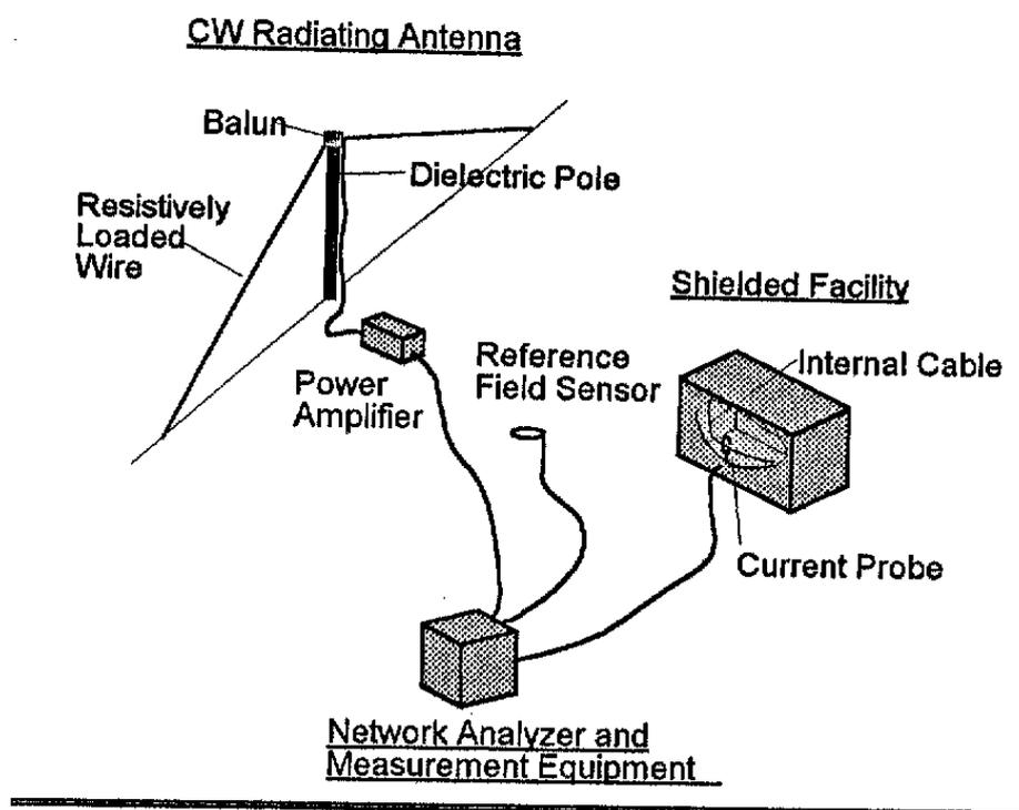
Figure 6. Configuration for CW testing.
