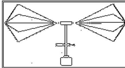
a. The biconical E-field sensor
