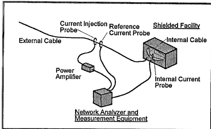
Figure 7. Current injection testing of a facility.
