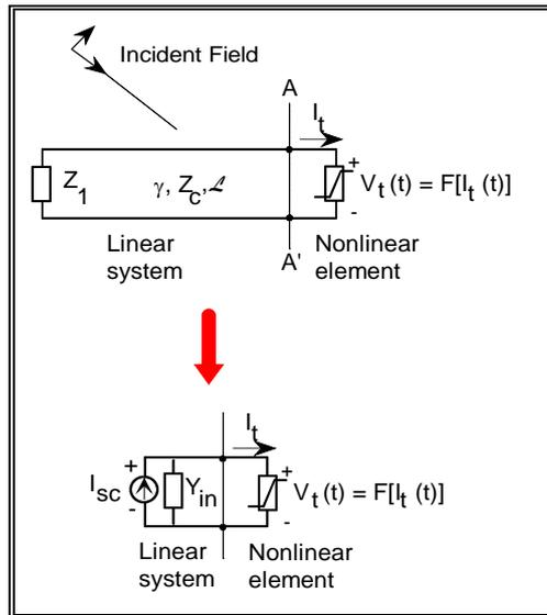
Figure B-1. Transmission line with a nonlinear load.
