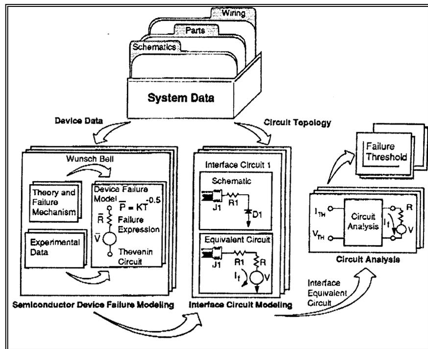
Figure C-1. Analysis elements of pin-level failure threshold analysis and evaluation.
