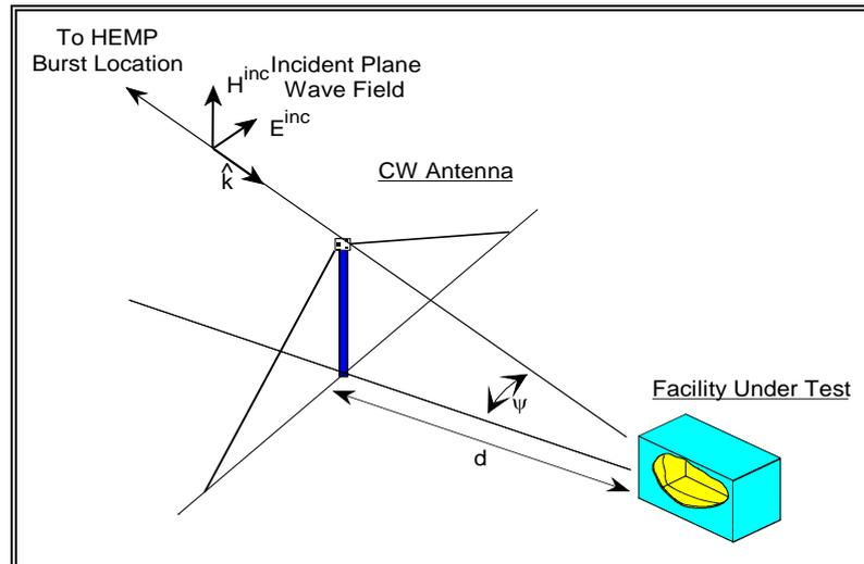
Figure 20. Relationship between the CW antenna and the Incident HEMP field.
