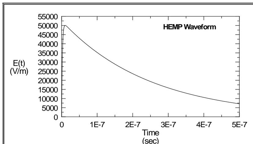
Figure 2. Transient HEMP waveform.
