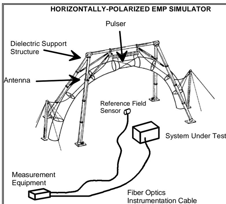
Figure 5. System-level testing using a threat-level EMP simulator.
