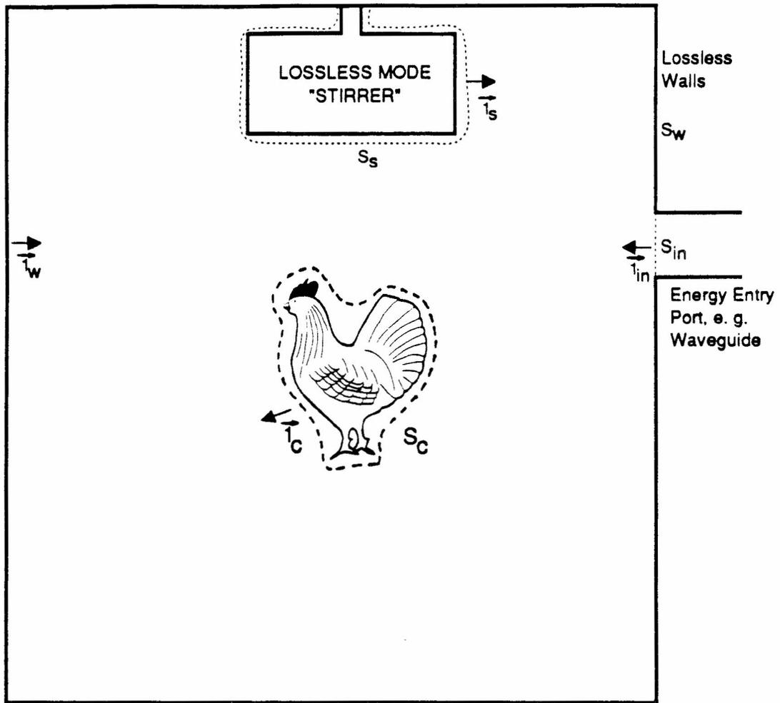
**Figure 1. Microwave Oven or Mode-Stirred Chamber**
