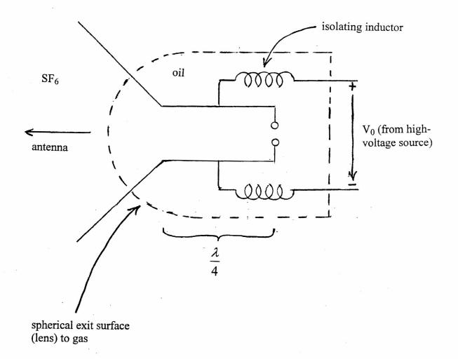
Figure 1. Low-Impedance, Quarter-Wave, Transmission-Line Oscillator Feeding High-Impedance Antenna
