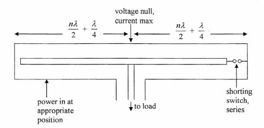
When the switch closes the open circuit (+1 reflection) goes to a short (-1 reflection) changing the phase of the reflection and making the center go to a voltage maximum, thereby sending power to the load. For maximum transfer of power to the load we need  $Z_c = 2\,Z_L$ .
