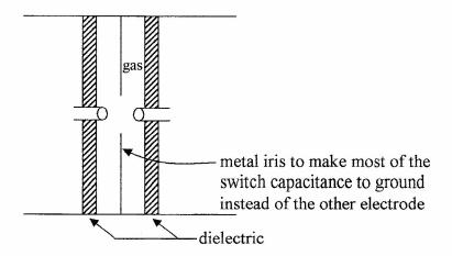
Note that the iris capacitance needs to be included when designing a particular resonant frequency for the oscillator.
