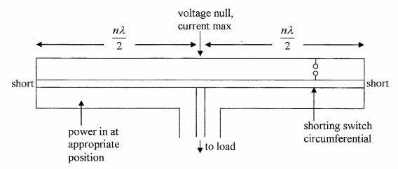
Sliding contacts at ends can tune up the null position to allow for perturbation due to switch capacitance.
