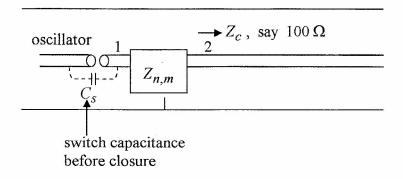
Think of a 2 port network, reactive, which puts no voltage on terminal 2 (loaded by  $Z_c$ ) at  $f_0$ . When switch closes  $\Rightarrow C_s$  is replaced by a short circuit. Then power is delivered to  $Z_c$ . Is this possible?
