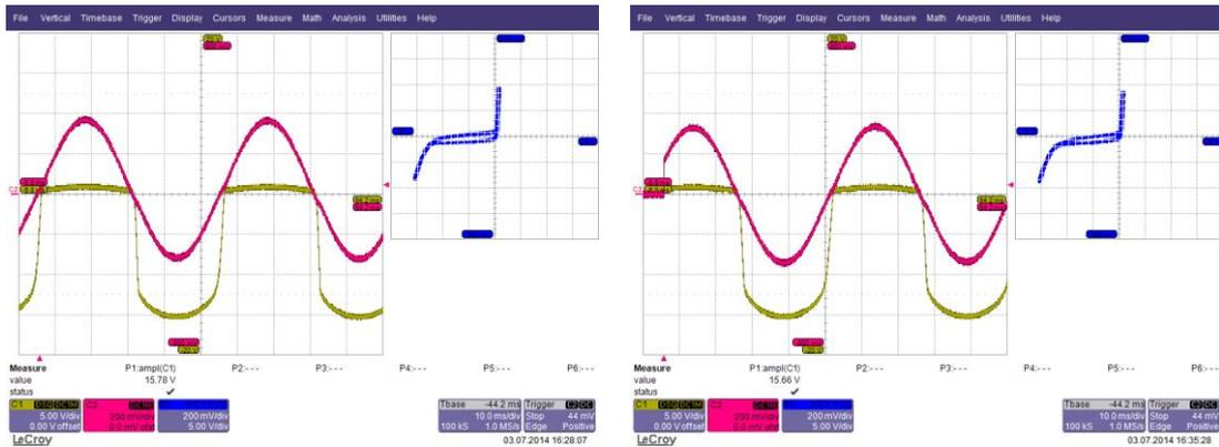
Figure 9: The I-V-Characteristic of a polycrystalline PV-cell before (left) and after 2000A surge in forward direction (right) shows no degradation.
