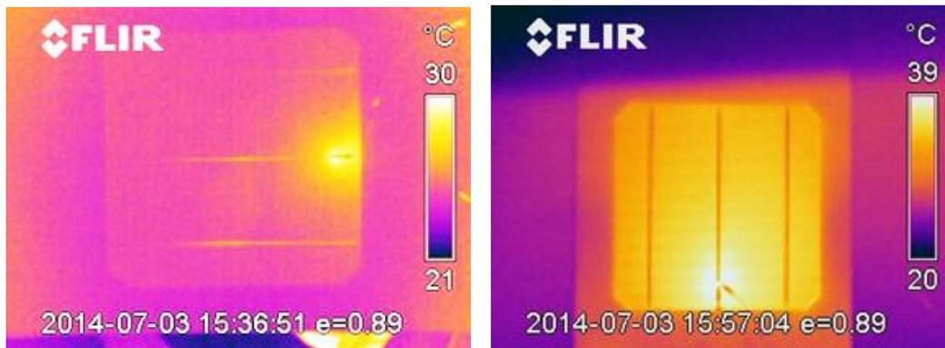
**Figure 8: Current density on the broken monocrystalline cell using an external current of 0.1 A (left) and same active cell without load in sunlight (right).**
