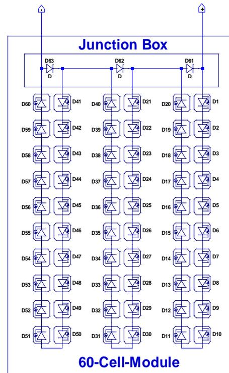
Figure 3: Electrical circuit of a module
