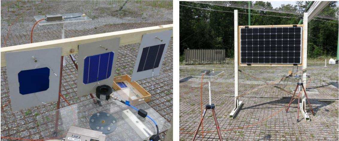
**Figure 11: HEMP-field tests of different PV-cells (left) and of 60 cells PV-modules (right)**
