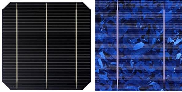
Figure 1: Monocrystalline cell (left) and Polycrystalline cell (right)
