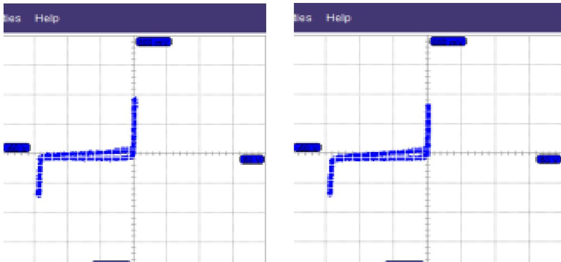
Figure 7: The I-V-characteristics of a monocrystalline PV-cell before (left) and after (right) a series of ESD discharges directly to the surface showed no changes and damages.
