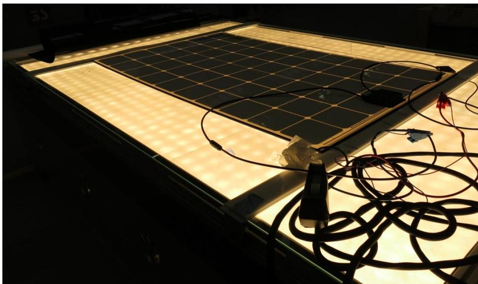
**Figure 12: This flasher made by PASAN (the worldwide reference for measurement systems for modules and cells in the photovoltaic industry) is used to measure the performance curve of a PV-module before and after EMP-illumination tests.**
