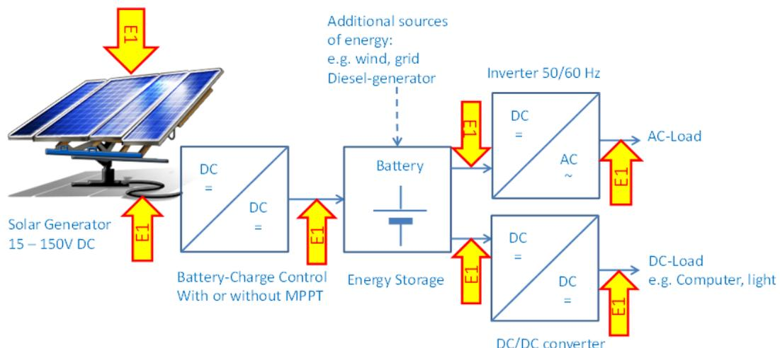
**Figure 13: E1 coupling paths for HEMP and lower frequency coupling to PV-systems**
