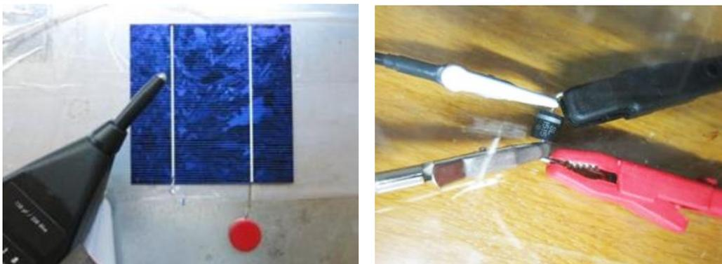
**Figure 6: ESD on cell surface (left) and surge on a bypass-diode (right)**
