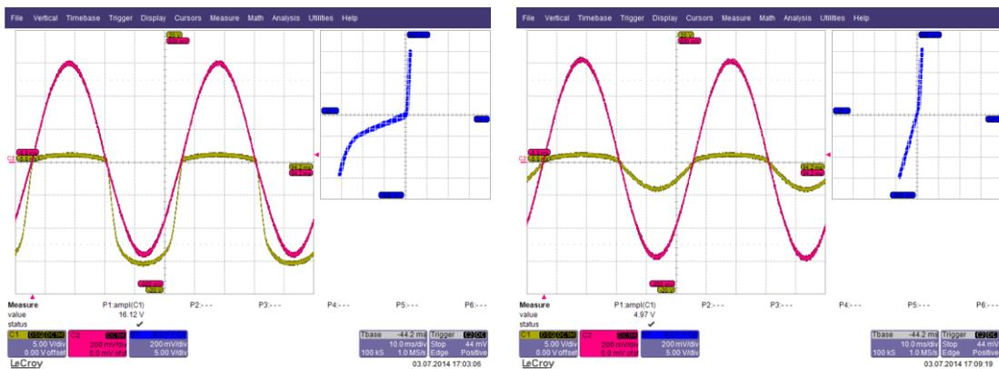
Figure 10: The I-V-Characteristic of a polycrystalline PV-cell shows some resistive leakage after a 250A surge in reverse direction (left). After a 500A surge in reverse direction the cell is damaged and behaves almost like a resistor (right).
