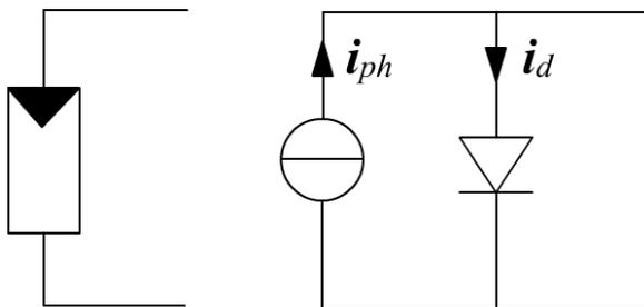
Figure 2: Schematic / Principle of PV-cells
