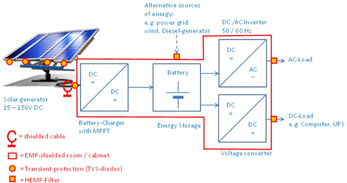
**Figure 14: Transient voltage suppressors on modules and integral shielding enclosure of control system**
