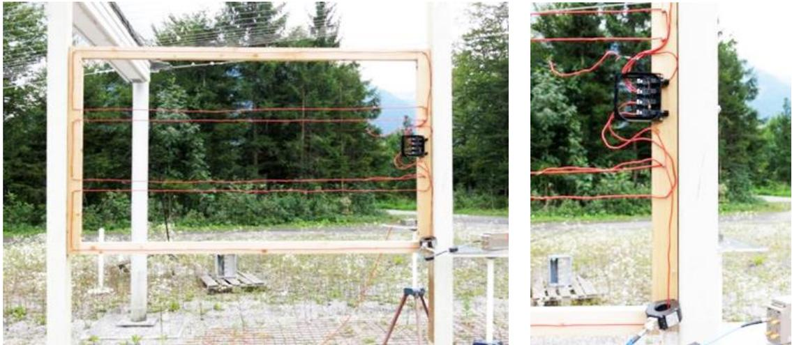
**Figure 4: Wire model of module (left) and a single loop (right) in the HEMP simulator**
