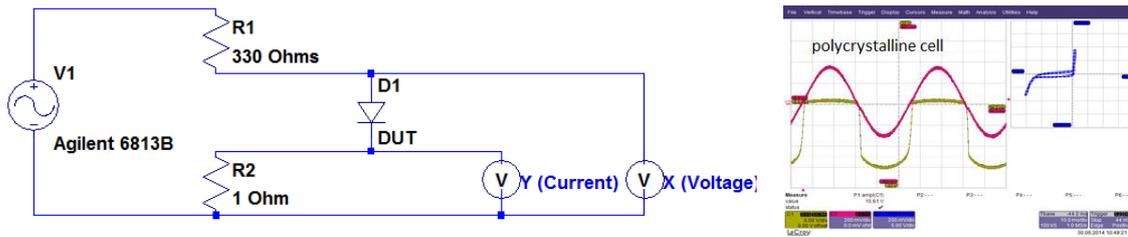
**Figure 5: I-V Diode characteristic test scheme (left) and test result (right)**
