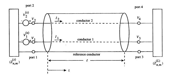
Fig. 2.1 Two-Wire Transmission-Line Directional Coupler
