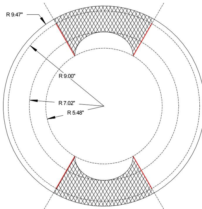
Figure 3-2. Shaped IRA-5 dish with removed area crosshatched.
