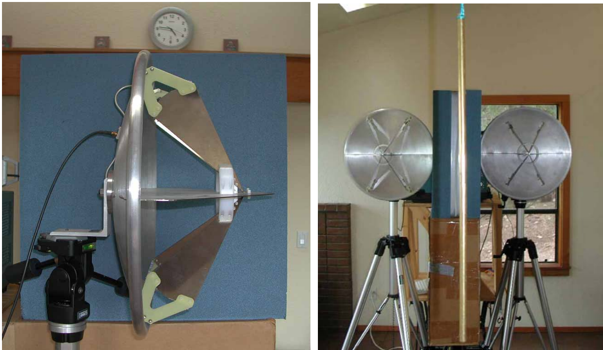
Figure 3.4. RF absorber material placement between IRAs. Target in foreground on left.
