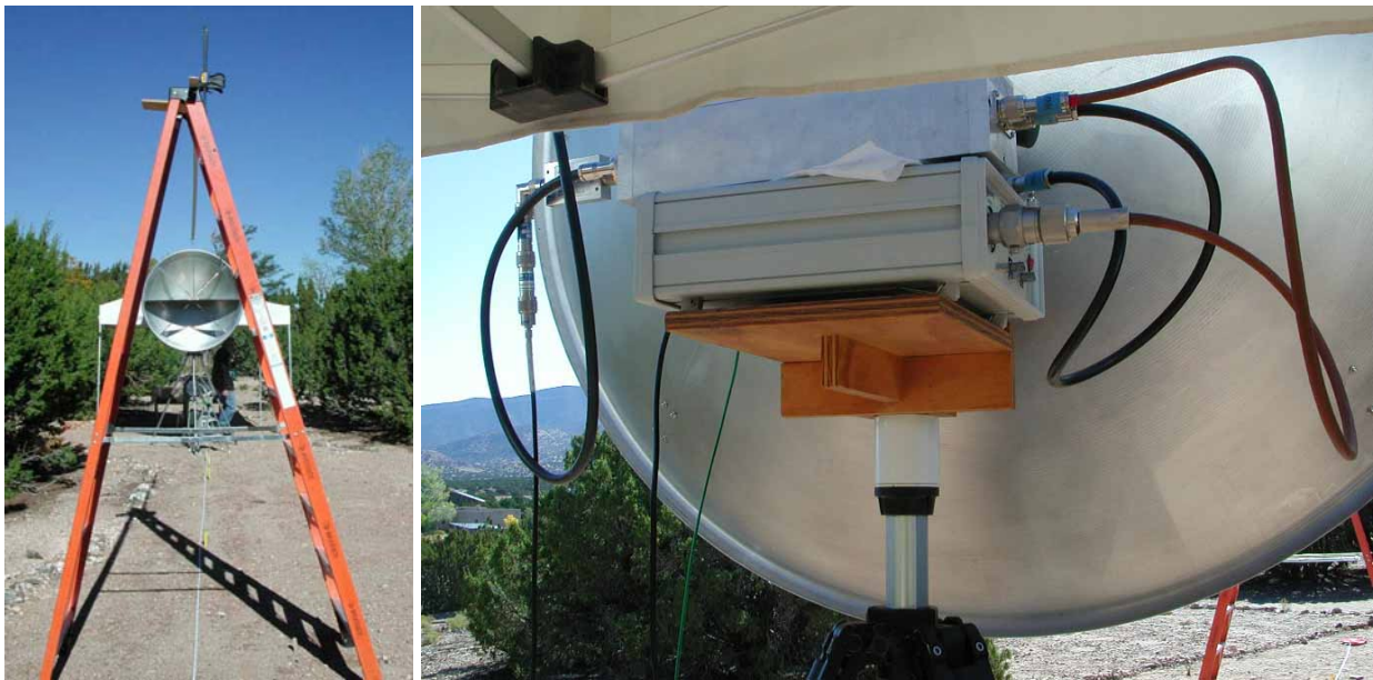
Figure 4.2. Target stand (left); FID pulser, oil-filled directional coupler and IRA-6 back (right).
