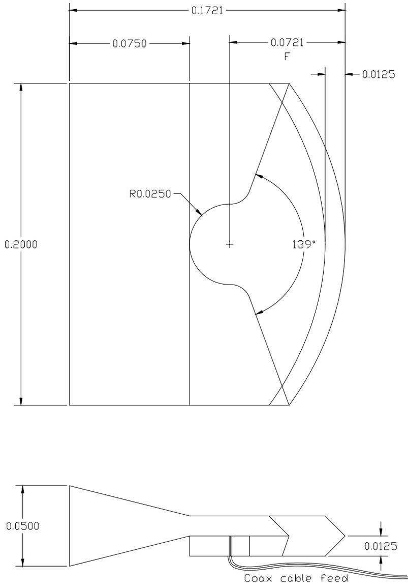
Figure 3.1. FH-1 drawing. Dimensions are in meters.
