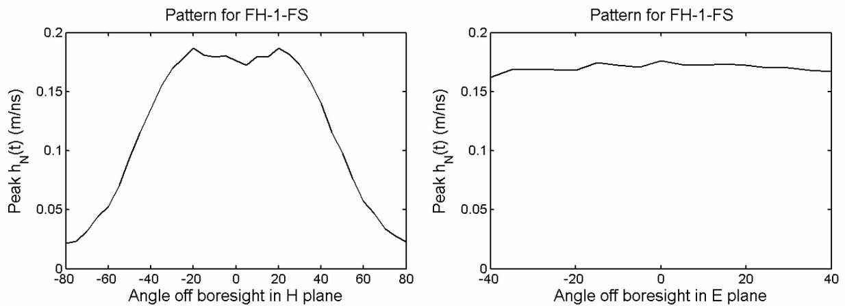
Figure 4.3. Antenna pattern for FH-1-FS feed section.
