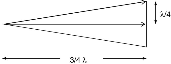
Figure 2.4. Geometry for calculating the level of defocus in the folded horn Aperture section.
