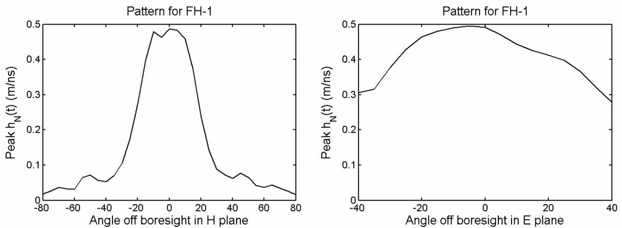
Figure 4.6. Antenna pattern for FH-1 folded horn.
