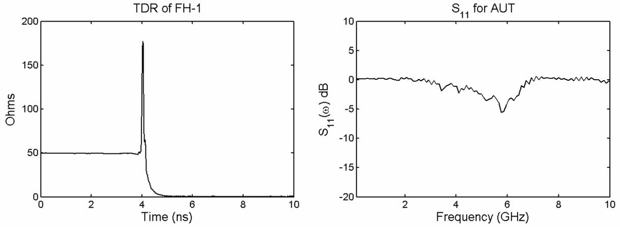
Figure 4.4. TDR and  $S_{11}$  of FH-1 folded horn.
