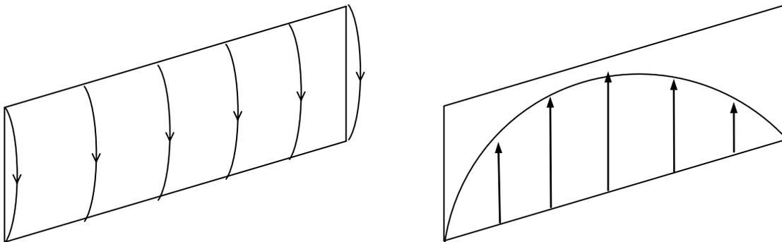
Figure 2.3. Aperture electric fields of the folded horn.
