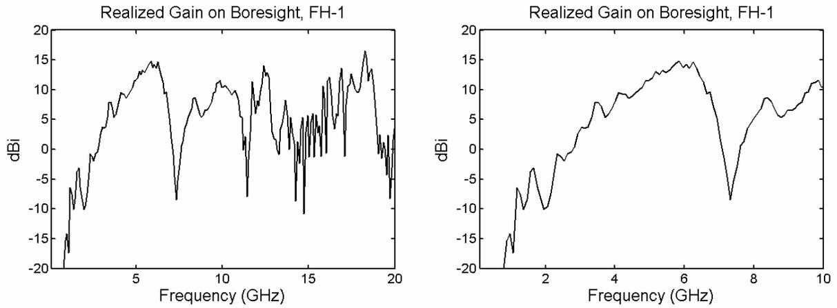
Figure 4.5. Realized Gain of FH-1 folded horn.
