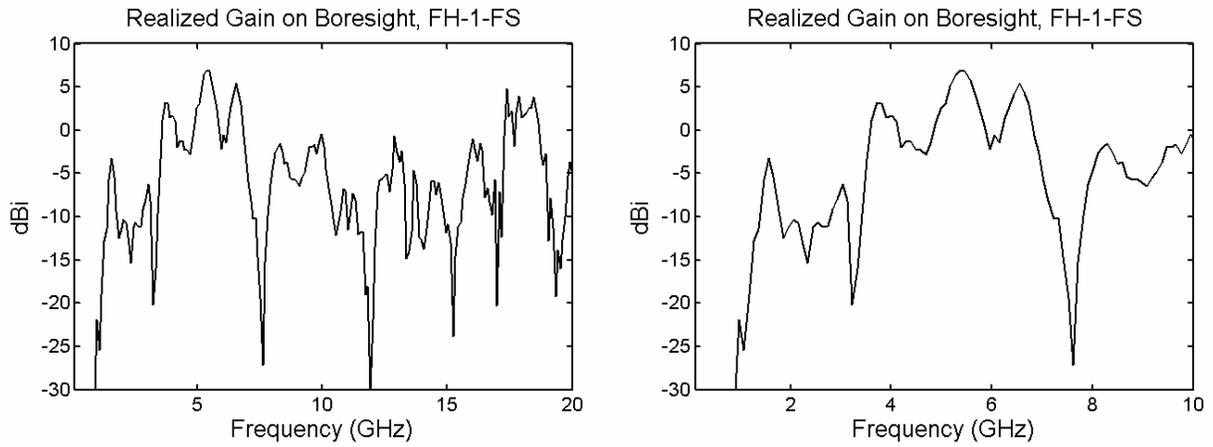
Figure 4.2. Realized Gain of FH-1-FS feed section.
