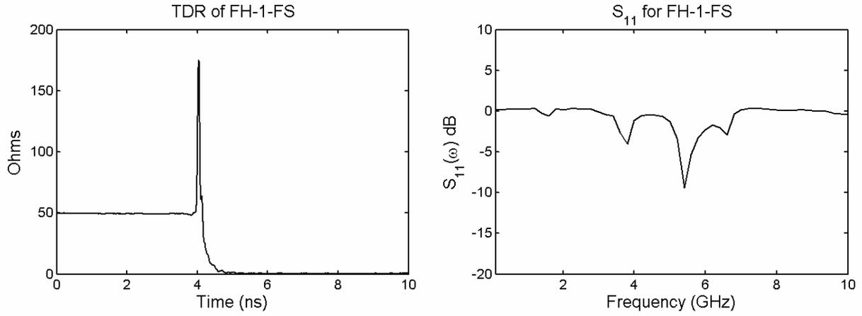
Figure 4.1. TDR and  $S_{11}$  of FH-1-FS feed section.
