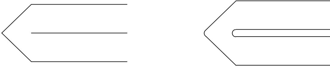
Figure 8.1. Softening the  $180^\circ$  bend, current design (left) and proposed modification (right).
