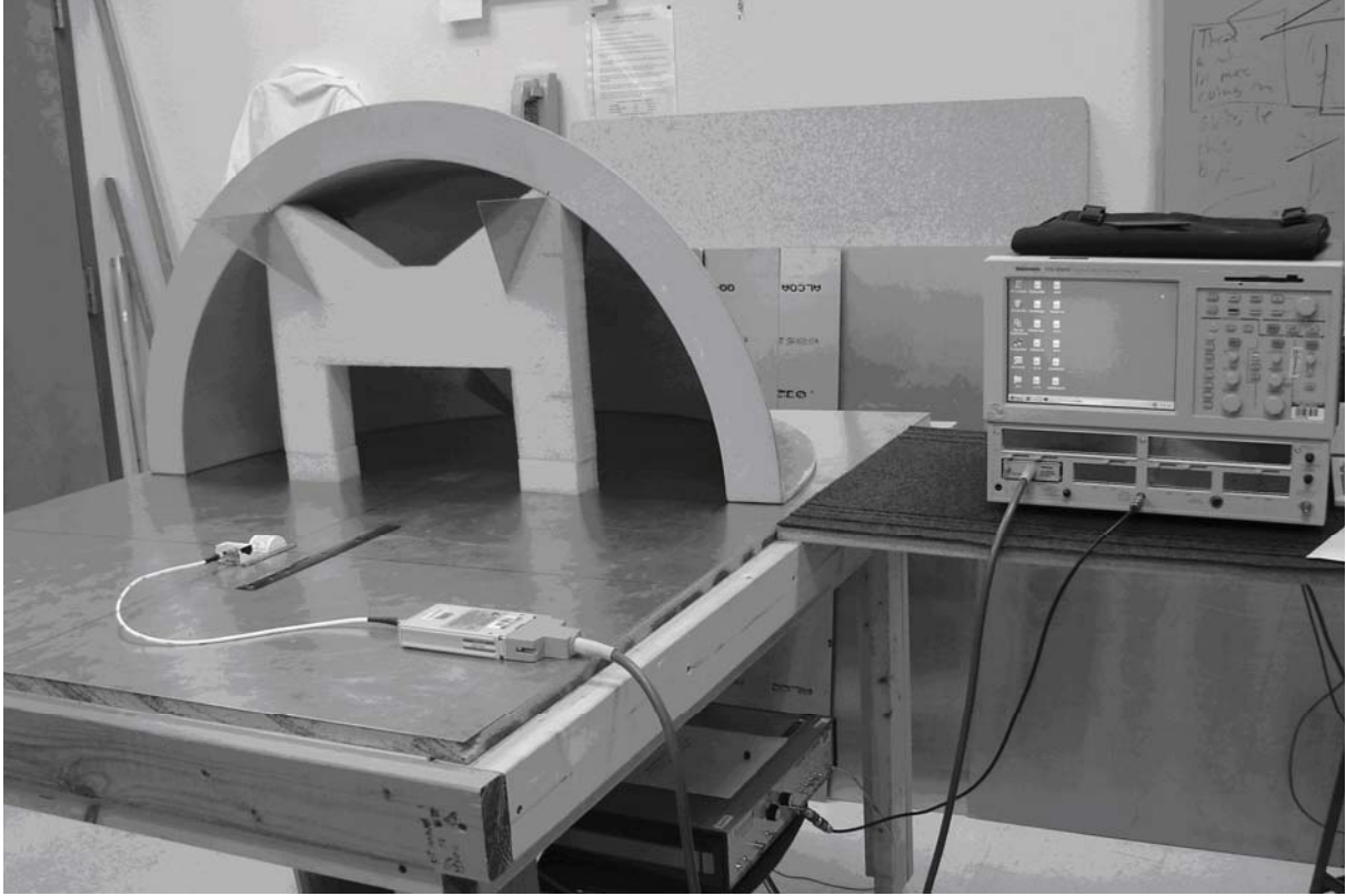
Figure 3: Experimental setup for a 60^\circ four-feed arm prolate-spheroidal IRA.
