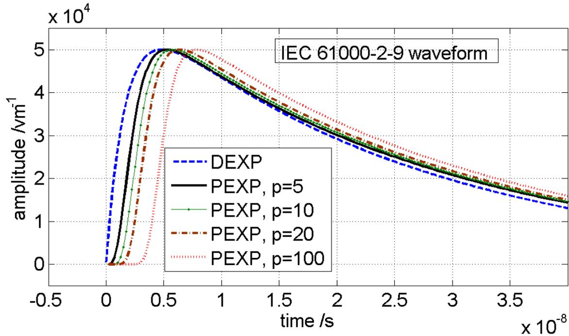
Fig.3 The influence of the value of  $p$  to pulse shape
