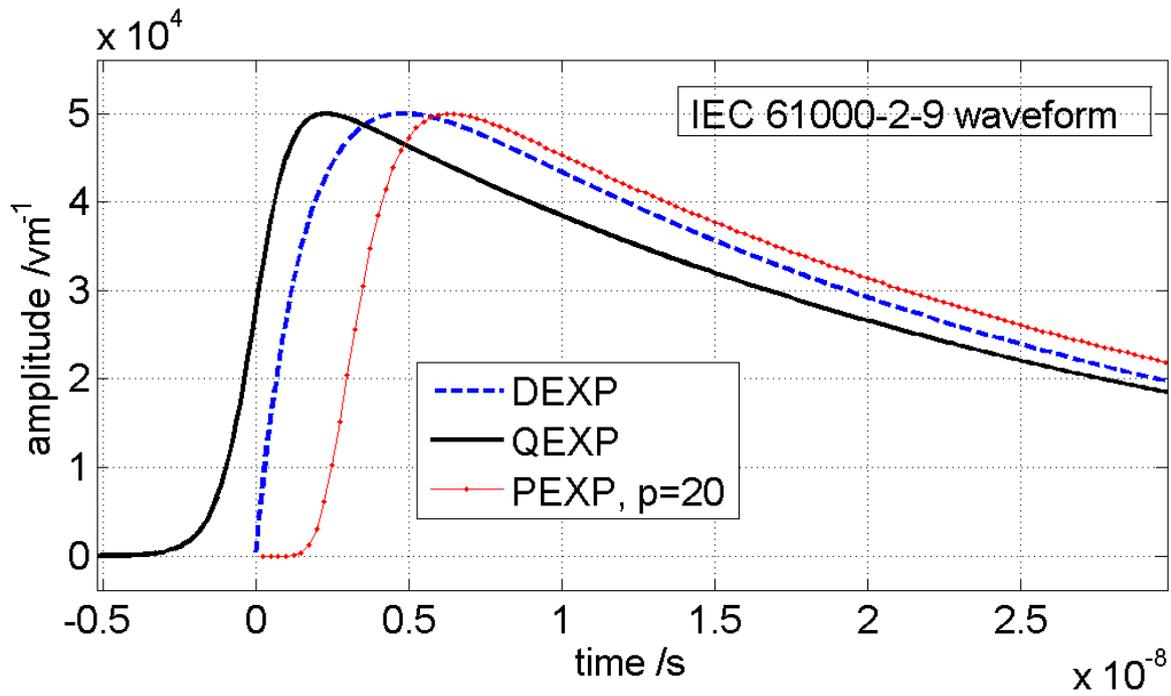
Fig.1 Temporal waveforms of three HEMP descriptions
