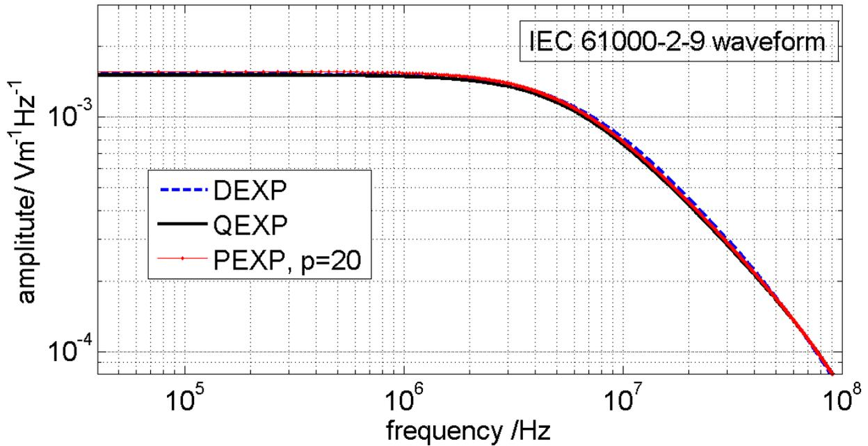
Fig.4 Spectral magnitude of the waveforms in Fig.1
