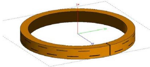
Figure 4: Horizontally mounted RSSWA with 31 slots (15 dB) at 2.4 GHz.
