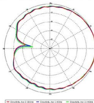
Figure 7: Radiation pattern of a vertically mounted (RSSWA) with 31 slots in x-y plane at various frequencies
