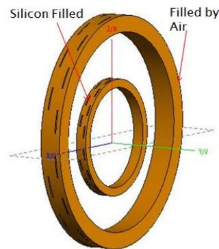
Figure 12: 2 RSSWAs (15dB) one filled with Silicon and the other filled by Air.
