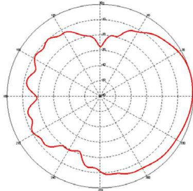
Figure 5: Radiation pattern of an (RSSWA) with 31 slots in x-y plane at 2.4 GHz.
