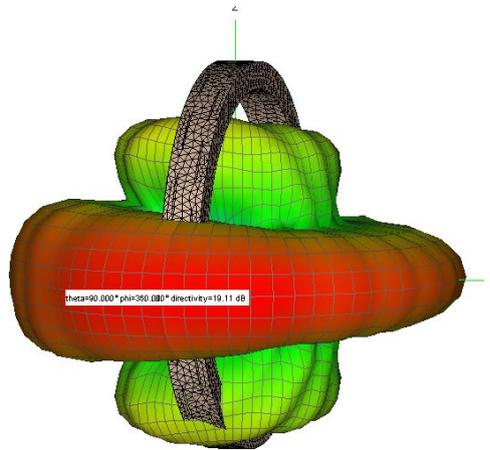
Figure 9: 3-D Radiation pattern of a vertically mounted (RSSWA) with 31 slots.
