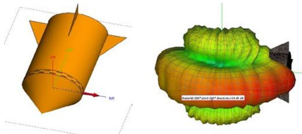
Figure 10: Integrated RSSWA in a missile with its simulated 3-D Radiation Pattern.
