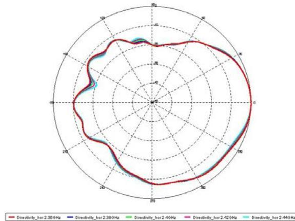
Figure3: Radiation pattern of an (RSSWA) with 18 slots in x-y plane at various frequencies.
