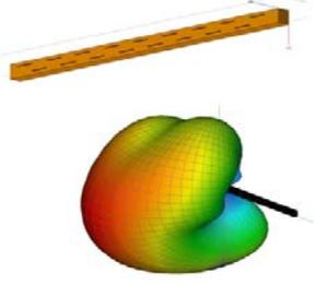
Figure 1: Radiation pattern of a regular unidirectional slotted waveguide antenna.
