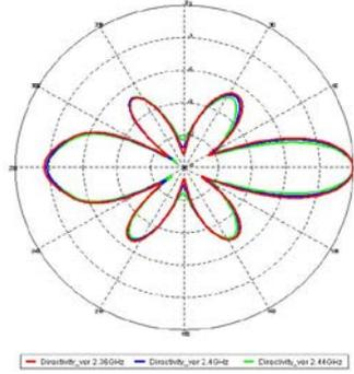
Figure 8: Radiation pattern of a vertically mounted (RSSWA) with 31 slots in the vertical plane at various frequencies
