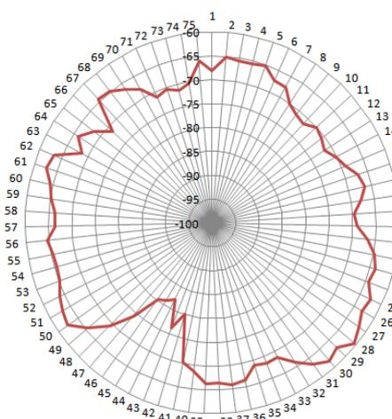
Figure 14: Measured radiation pattern in x-y plane with 18slots
