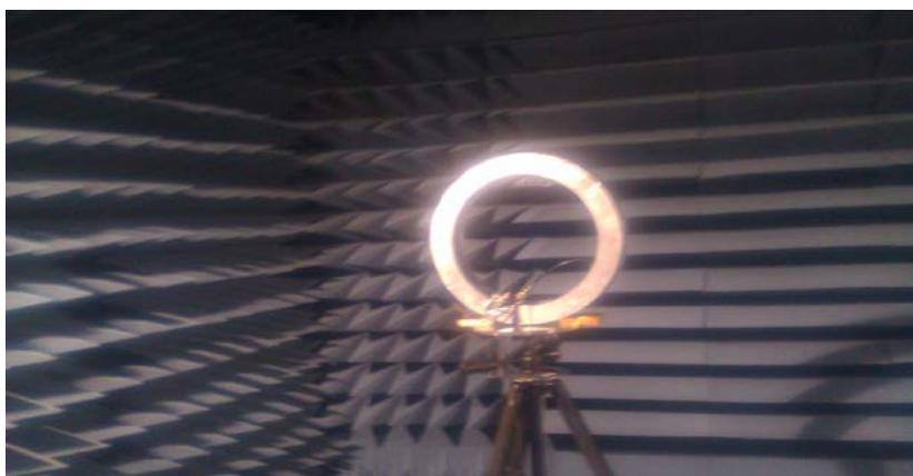
Figure 13: The fabricated antenna with 18 slots
