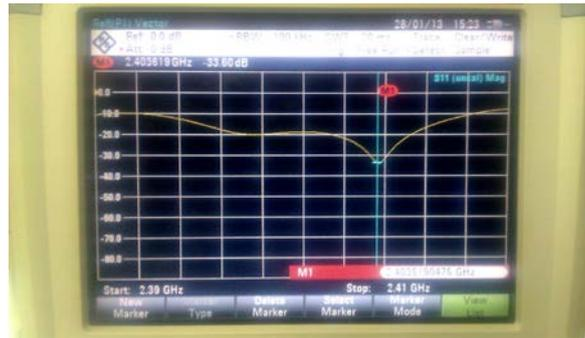
Figure 15: Reflection loss versus frequency
