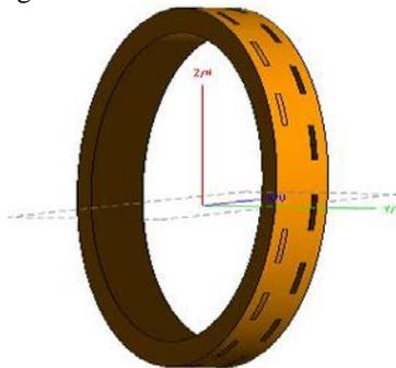
Figure 6: Vertically mounted (RSSWA) with 31 slots (15 dB) at 2.4 GHz.
