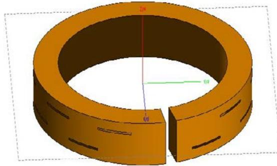
Figure2: Ring-shape slotted waveguide antenna (RSSWA) with 18 slots (12 dB) at 2.4 GHz.
