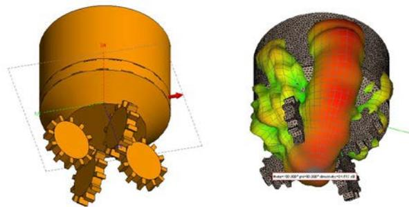
Figure 11: Integrated RSSWA in an Oil Drilling Device with its simulated 3-D Radiation Pattern.
