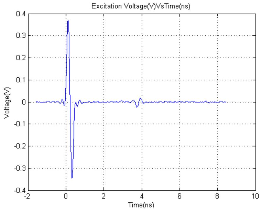
Fig. 13 Excitation signal used for time domain measurement
