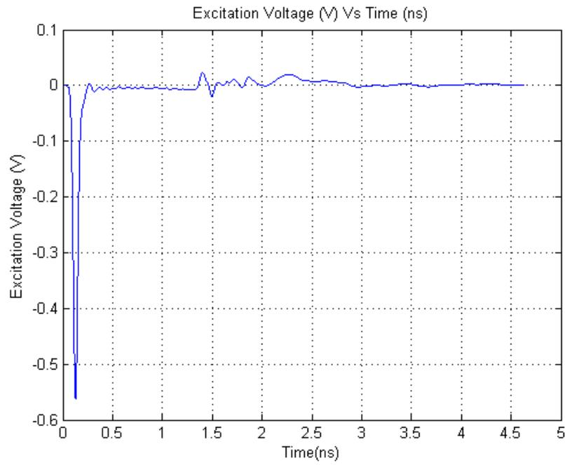
Fig. 3.Input excitation signal (Simulation)
