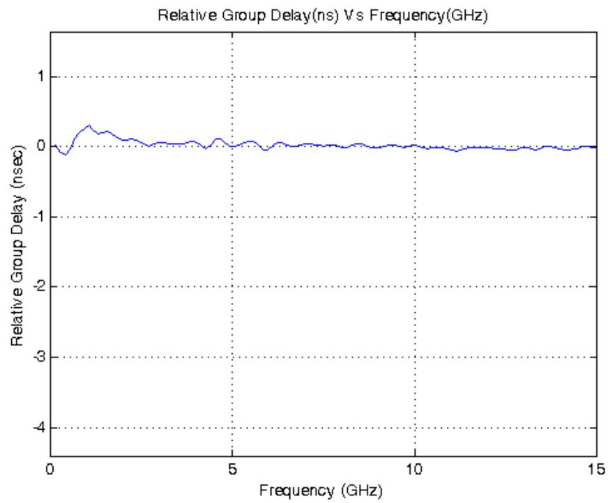
Fig. 8. Relative Group delay using Conjugate Gradient method
