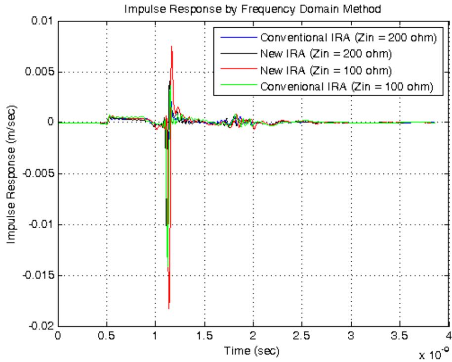
Fig. 10. Impulse response of full IRAs using Fourier transforms method
