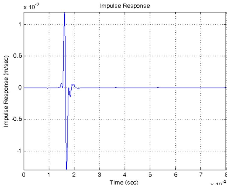
Fig. 15. Impulse response of ACD fed HIRA using Conjugate gradient method
