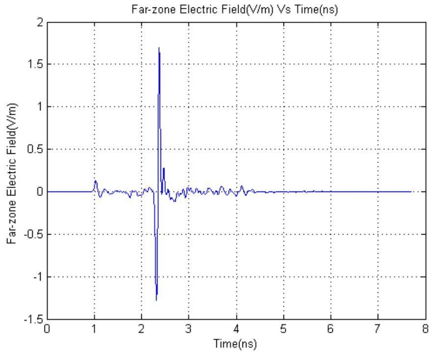
Fig. 4.Far zone electric field (Simulation)
