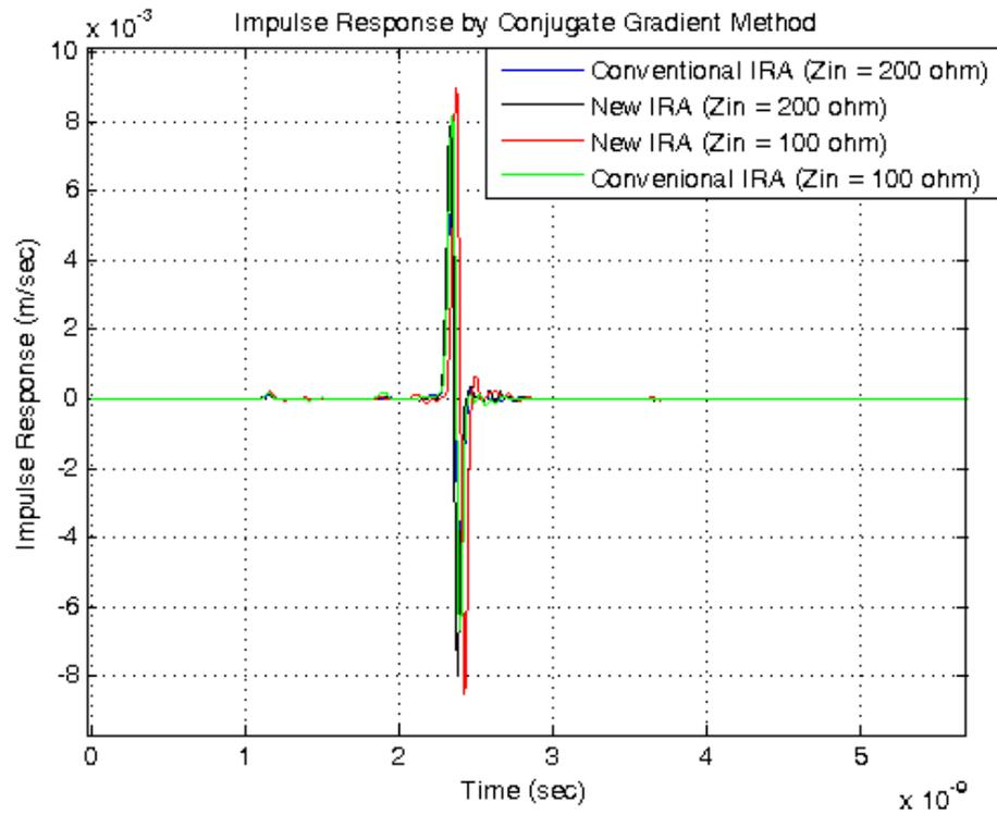
Fig. 11. Impulse response of full IRAs using Conjugate gradient method
