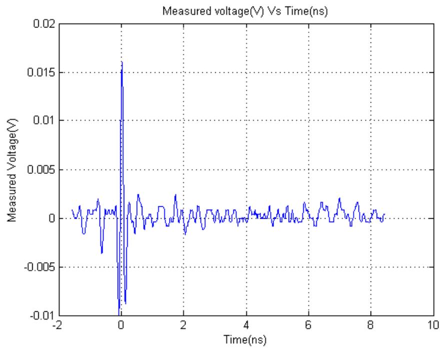
Fig. 14 Measured time domain response of new HIRA
