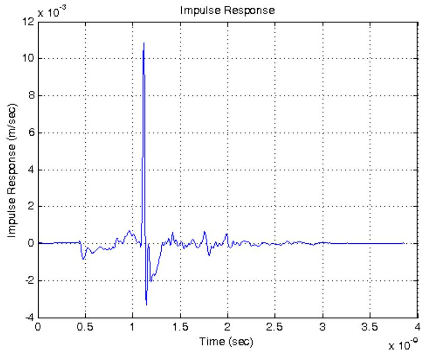
Fig. 5. Estimated impulse response using Fourier transform method
