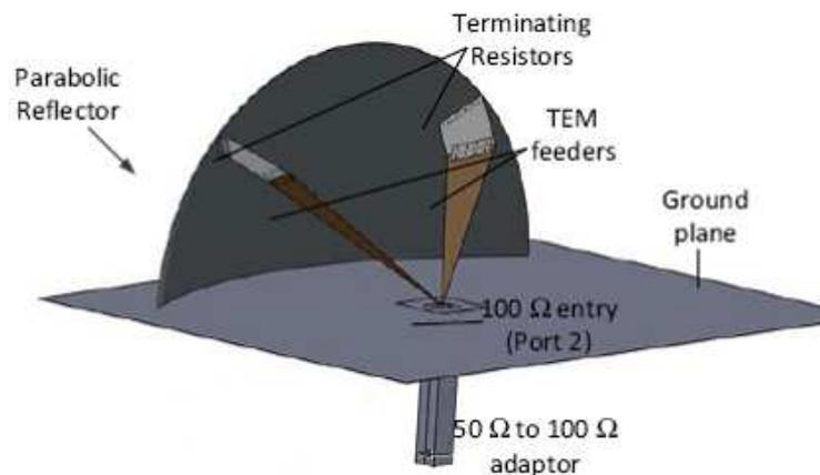
Fig. 1. Schematic of Conventional HIRA
