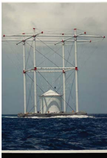
Figure 17. EMPRESS II HEMP Simulator [reproduced from 24], which is basically a resistively loaded monocone antenna above a ground plane
