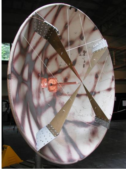
Figure 1. Illustration of an impulse radiating antenna (IRA) at the Swiss HPE Laboratory
