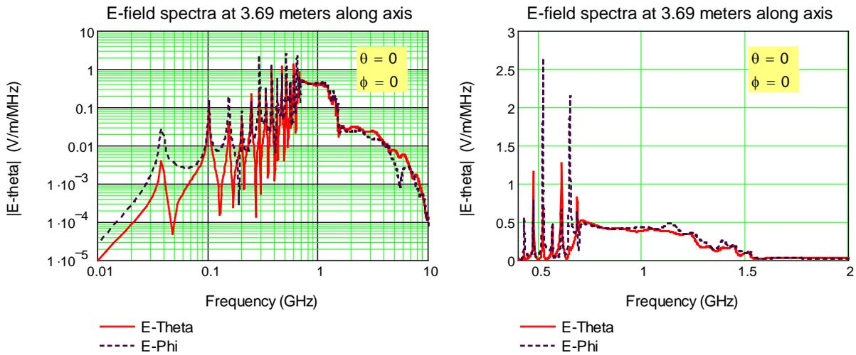
**Figure 7.** Calculated spectral field at a distance of 3.69m; [500 (V/m)/GHz]
