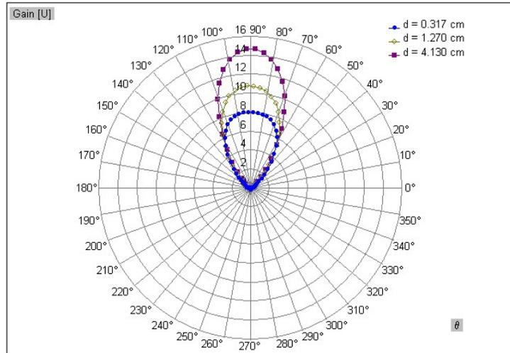
**Figure 3. Effect of the conductor diameter on the realized gain of the helical antenna at 400 MHz (WIPL-D calculations)**
