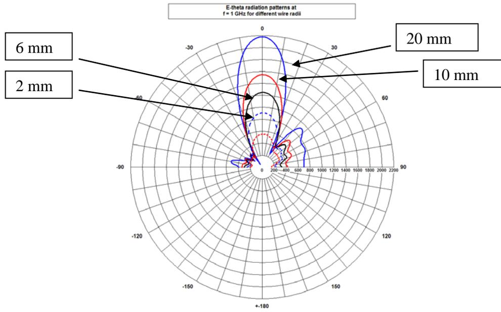
**Figure 8.** Radiation patterns at 1 GHz, for a range of minor diameters
