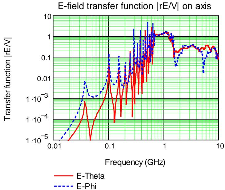
**Figure 4.** Calculated transfer function as a function of frequency
