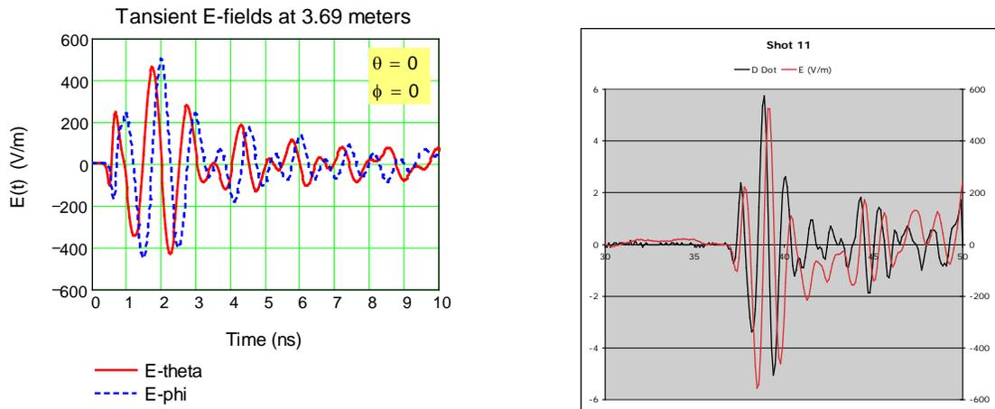
**Figure 5.** Comparison of calculated and measured transient field at a distance of 3.69m
