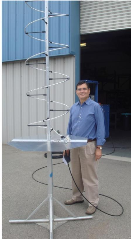
**Figure 21. The helical antenna for a center frequency of 200 MHz.**
