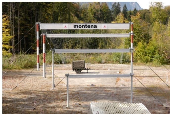
**Figure 2.** View of the wave-guiding structure and working volume of the Swiss VEPES simulator.
