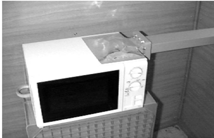
**Figure 23. Power extraction from a microwave oven using a WR-340 Waveguide.**
