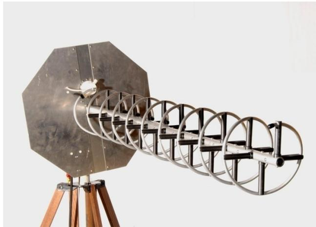
**Figure 17. Photo of the 500 MHz Swiss Helix Antenna.**
