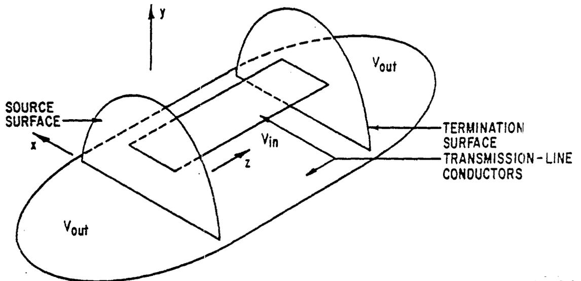
B. PARALLEL-PLATE TRANSMISSION LINE WITH ONE VERY LARGE PLATE
