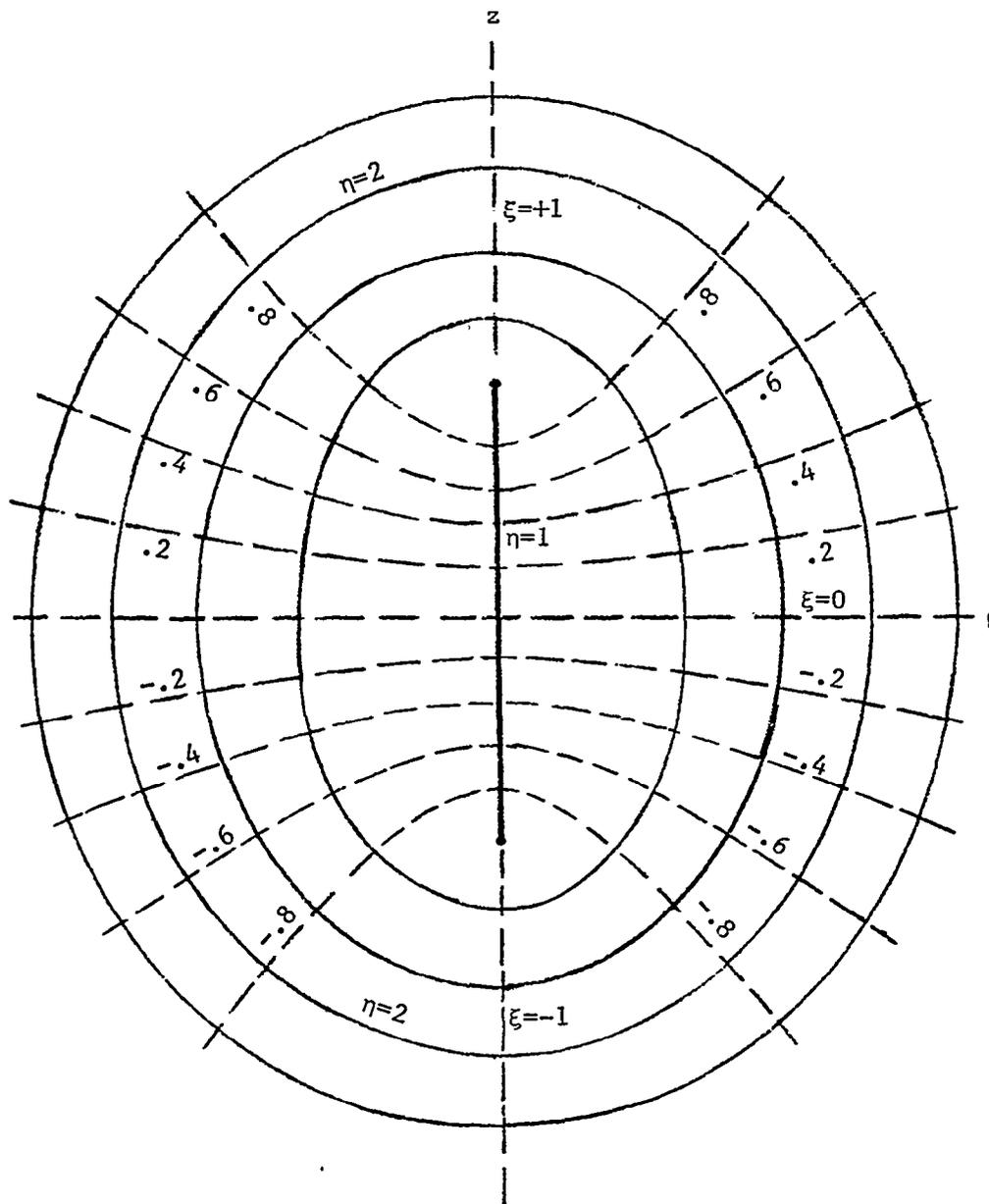
FIGURE 2. Prolate Spheroidal System of Coordinates.
