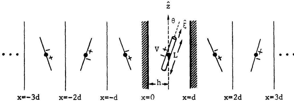
Figure 1a. Geometry of the antenna in a parallel plate region.
