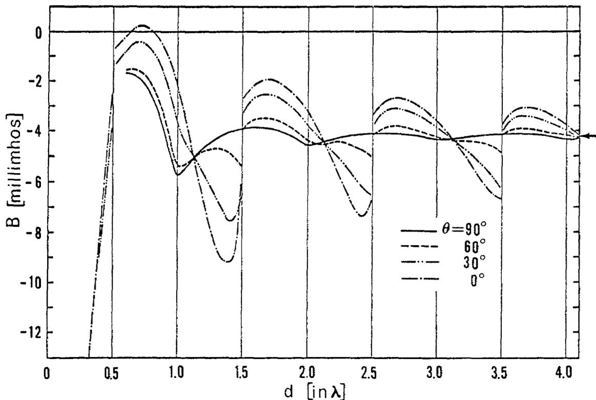
Figure 4. Plots of the input conductance  $G$ , and susceptance  $B$ , of the antenna as a function of the plate separation. The arrow indicates the computed free space values.  $L = \lambda/2$ ,  $h = d/2$ ,  $\Omega = 10$ .
