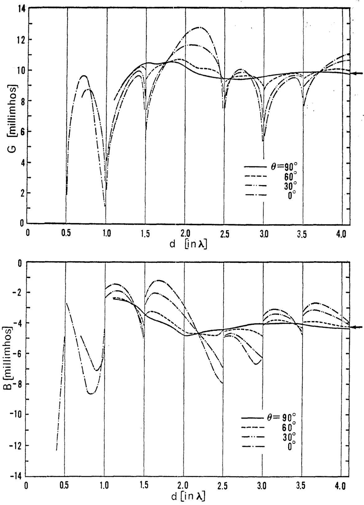
Figure 5. Plots of the input conductance  $G$ , and susceptance  $B$ , of the antenna as a function of the plate separation. The arrow indicates the free space values.  $L = \lambda/2$ ,  $h = d/4$ ,  $\Omega = 10$ .
