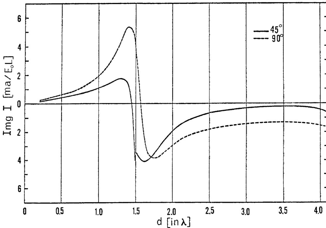
Figure 8. Plots of the real and imaginary parts of the current at the midpoint of a scattering element with a TEM wave of magnitude  $E_0$  incident.  $L = .3d$ ,  $h = d/2$ ,  $\Omega = 10$ ,  $\phi = 0^\circ$ .
