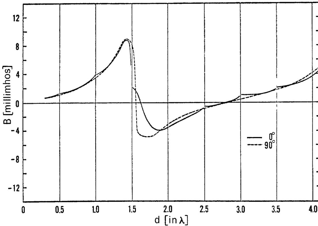
Figure 6. Frequency response of the input admittance,  $G$  and  $B$ , of the antenna. In this case,  $L = .3d$ ,  $h = d/2$ , and  $\Omega = 10$ .
