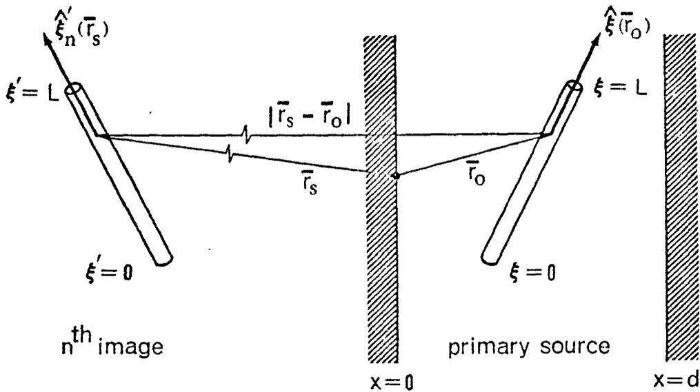
Figure 1b. Relevant quantities in defining the Green's function for the parallel plate.
