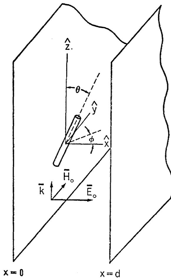
Figure 2. Orientation of the wire scattering element with a TEM wave incident.
