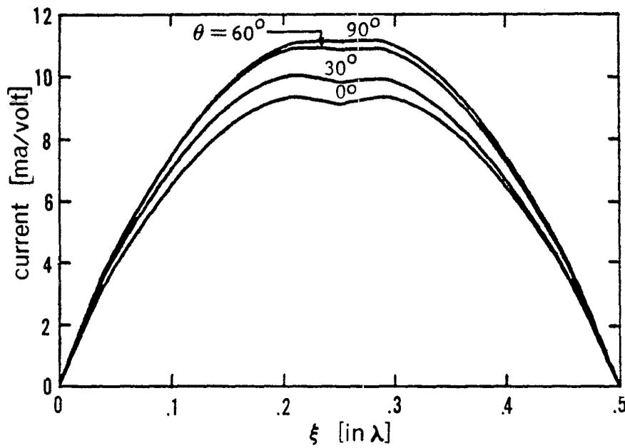
Figure 3. Magnitude of the antenna current distribution for various inclination angles.  $L = .5\lambda$ ,  $d = 1.49\lambda$ ,  $h = d/2$  and  $\Omega = 10$ .
