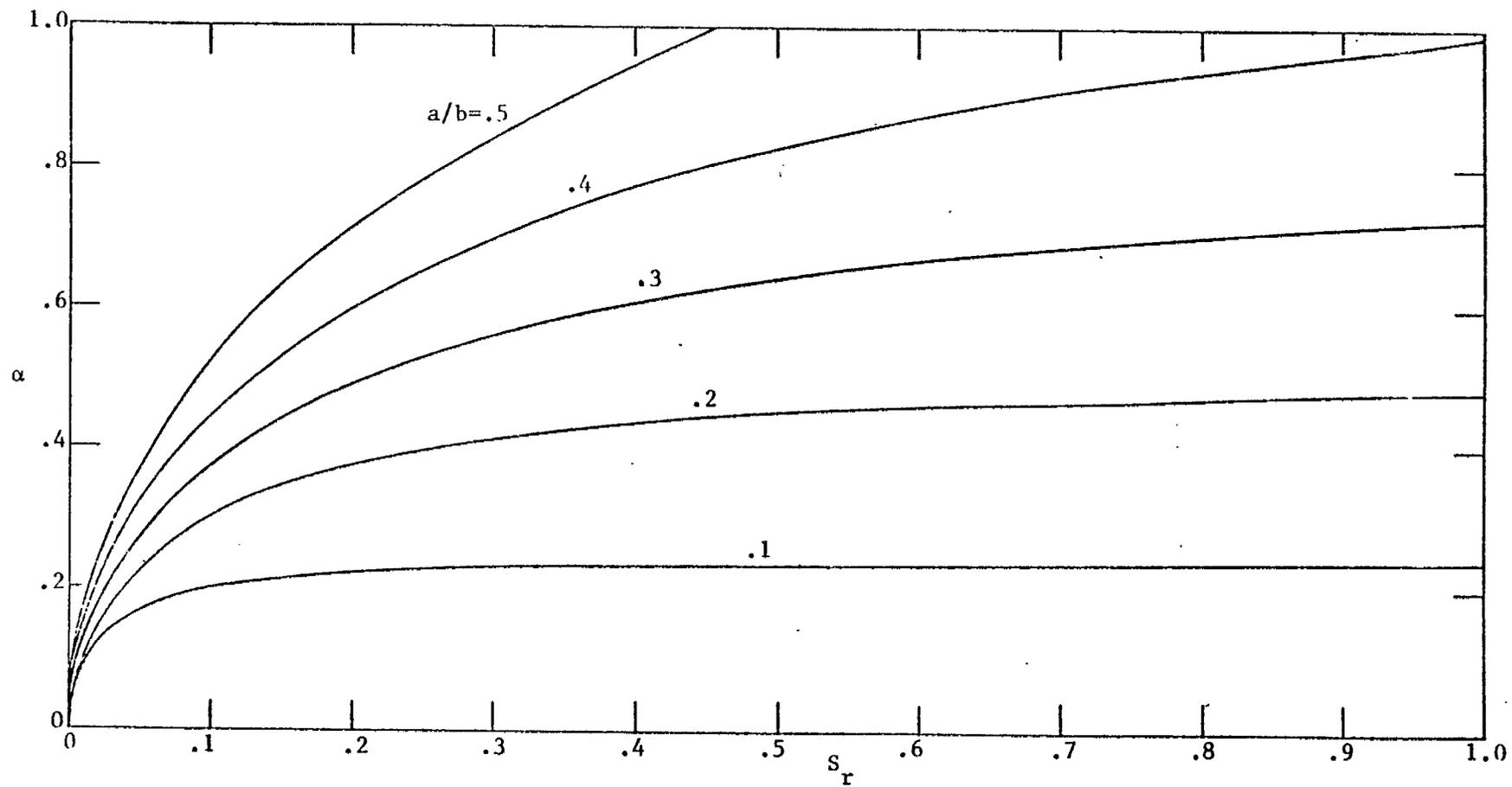
Figure 4.  $\alpha$  vs. relative elastance for thin inner conductors.
