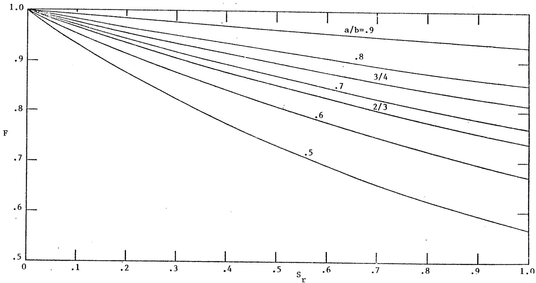
Figure 3. Correction factor vs. relative elastance for thick inner conductors.
