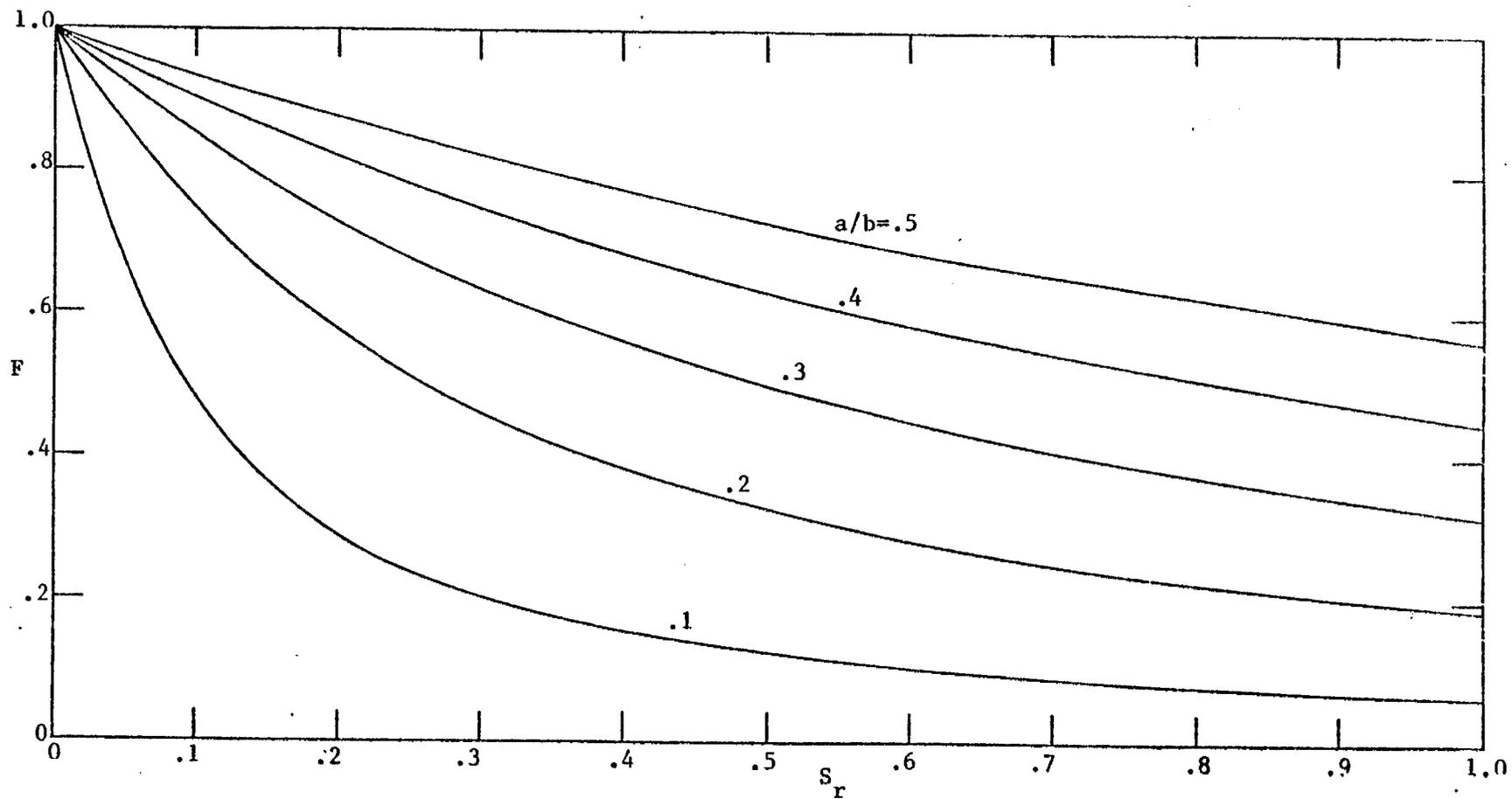
Figure 2. Correction factor vs. relative elastance for thin inner conductors.
