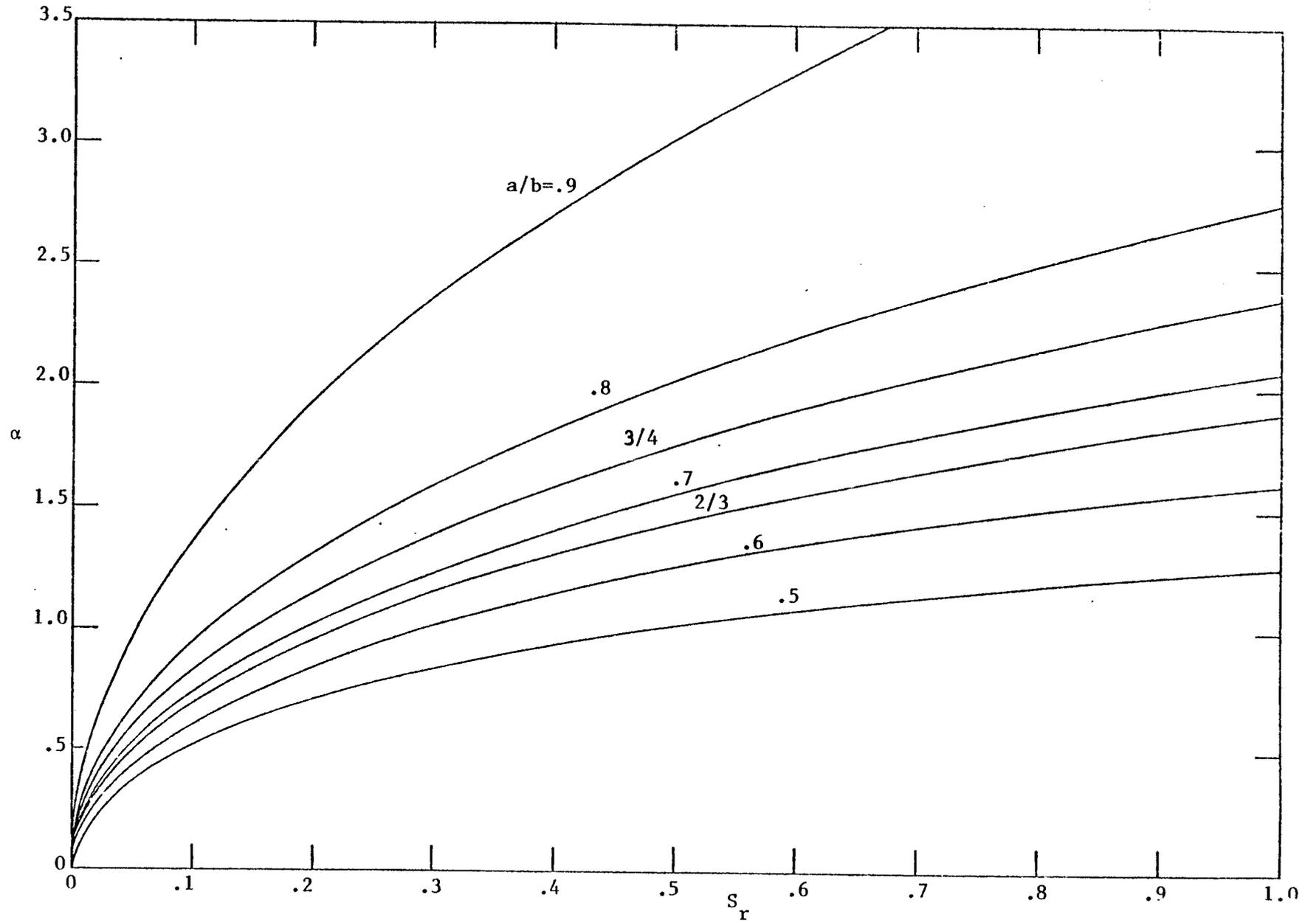
Figure 5.  $\alpha$  vs. relative elastance for thick inner conductors.
