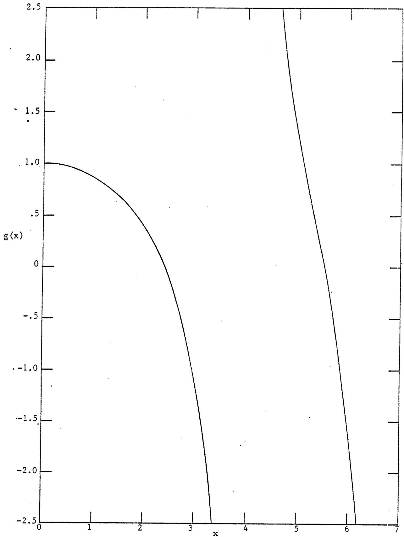
Figure 10. Auxiliary function for computing effective  $S_r$  of a disk line.
