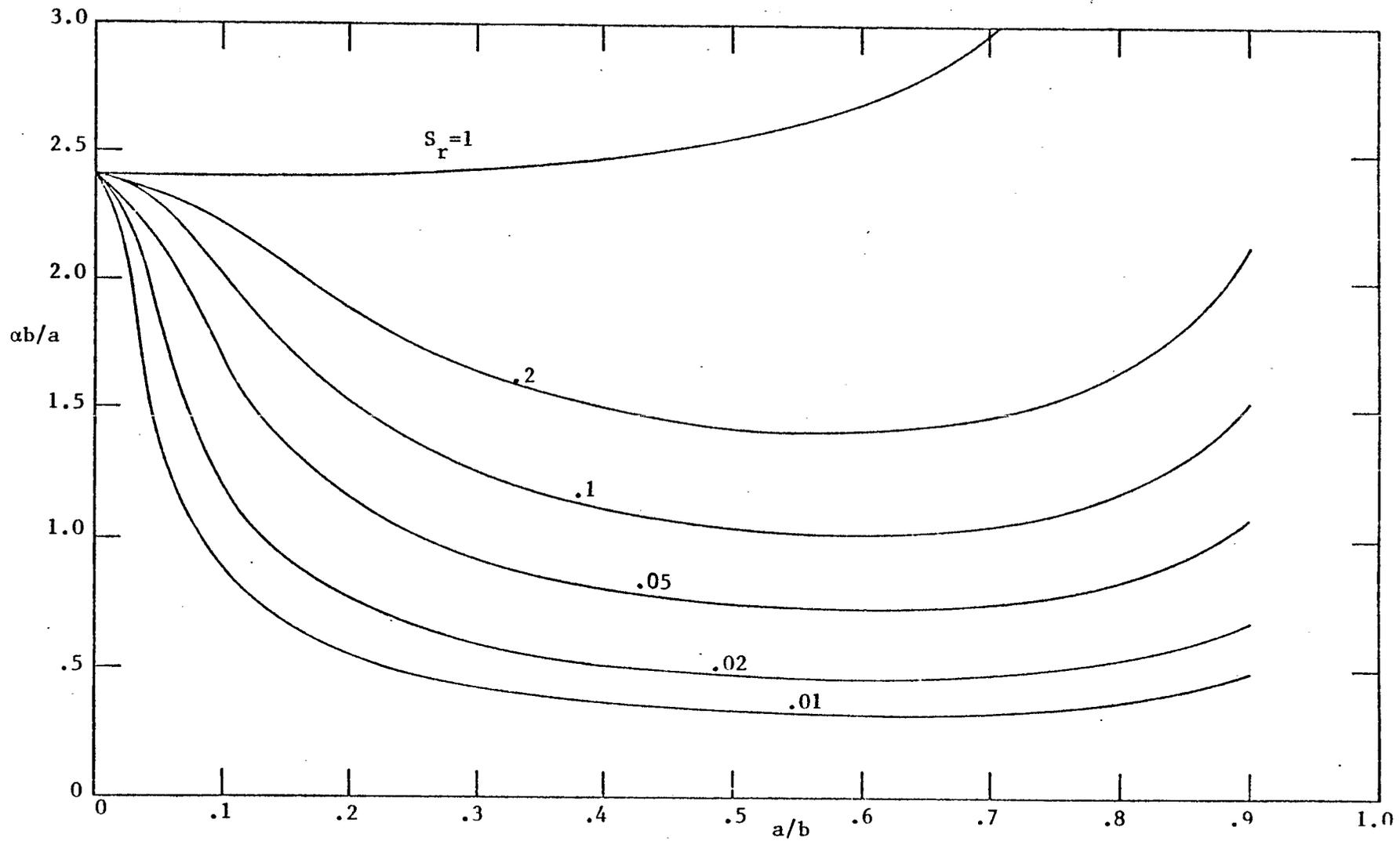
Figure 6.  $(\alpha b/a)$  vs.  $a/b$  for a few values of relative elastance.
