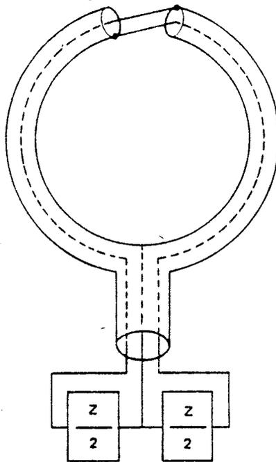
(B) EQUIVALENT CIRCUIT FOR LOAD
