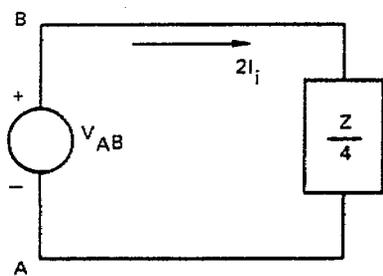
(B) FINAL SIMPLIFIED EQUIVALENT CIRCUIT
