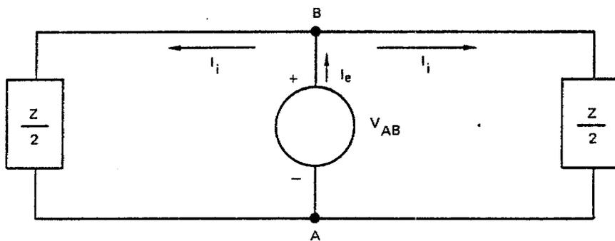
(A) SOURCE VOLTAGE – LOAD IMPEDANCE EQUIVALENT CIRCUIT
