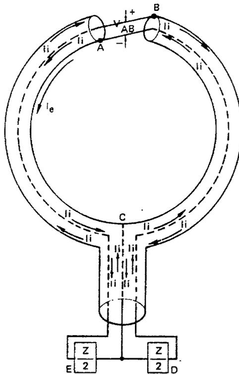
Figure 3. Relationship Between  $i_e$  and  $i_i$
