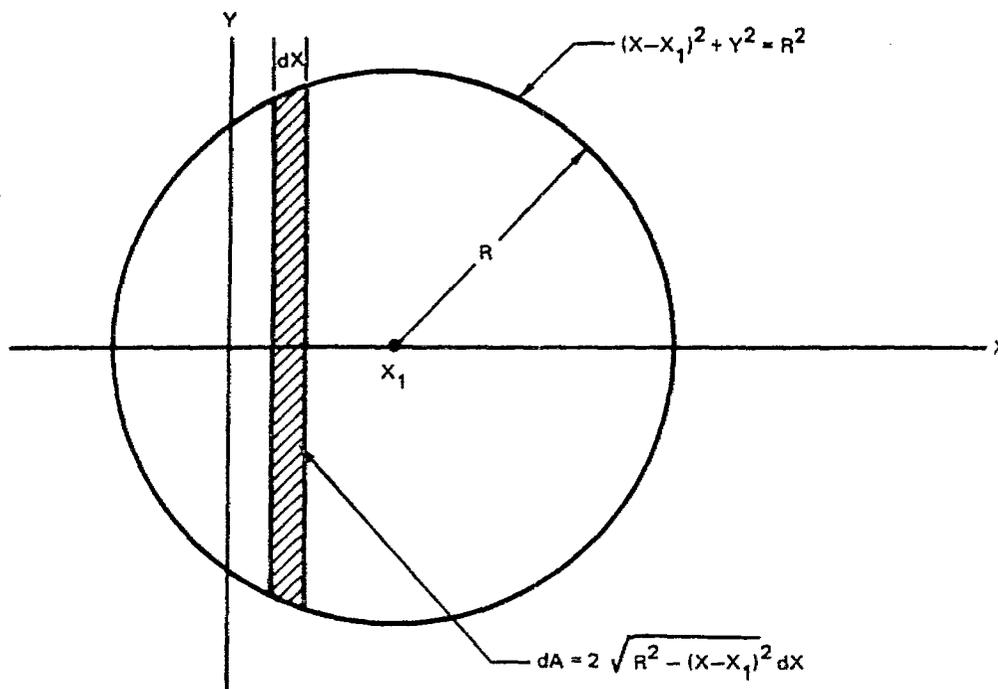
Figure A.1. Equation for the Loop Boundary, Illustrating a Differential Area Element
