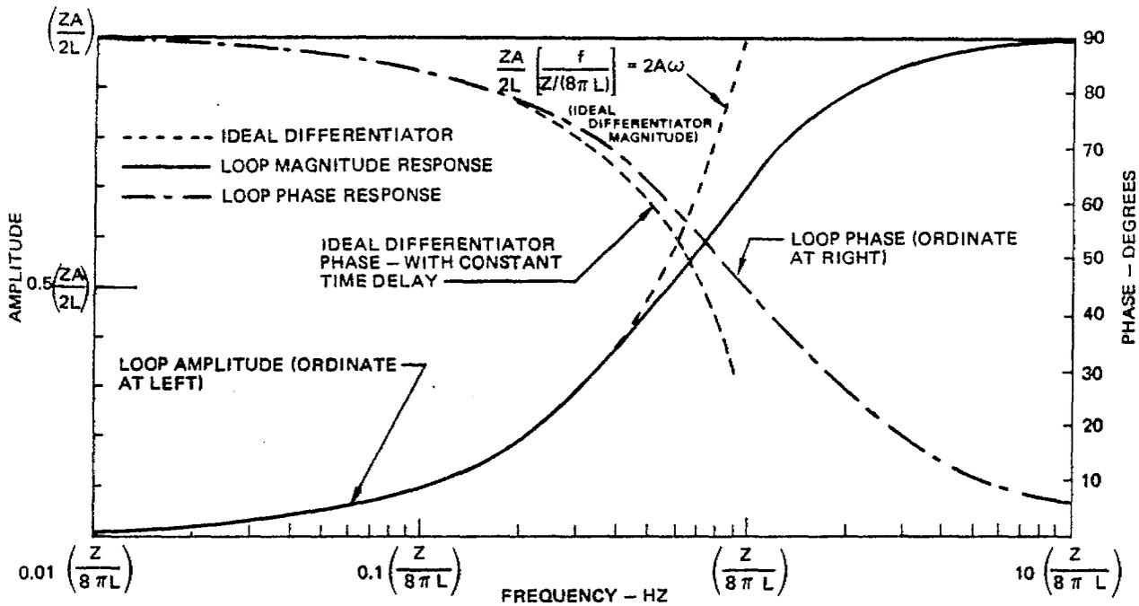
Figure 6. Transfer Function  $H(j2\pi f) = \frac{V(j2\pi f)}{B(j2\pi f)}$
