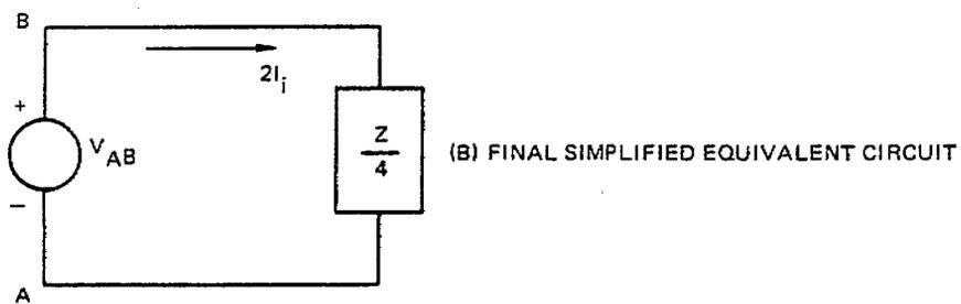
(B) FINAL SIMPLIFIED EQUIVALENT CIRCUIT
