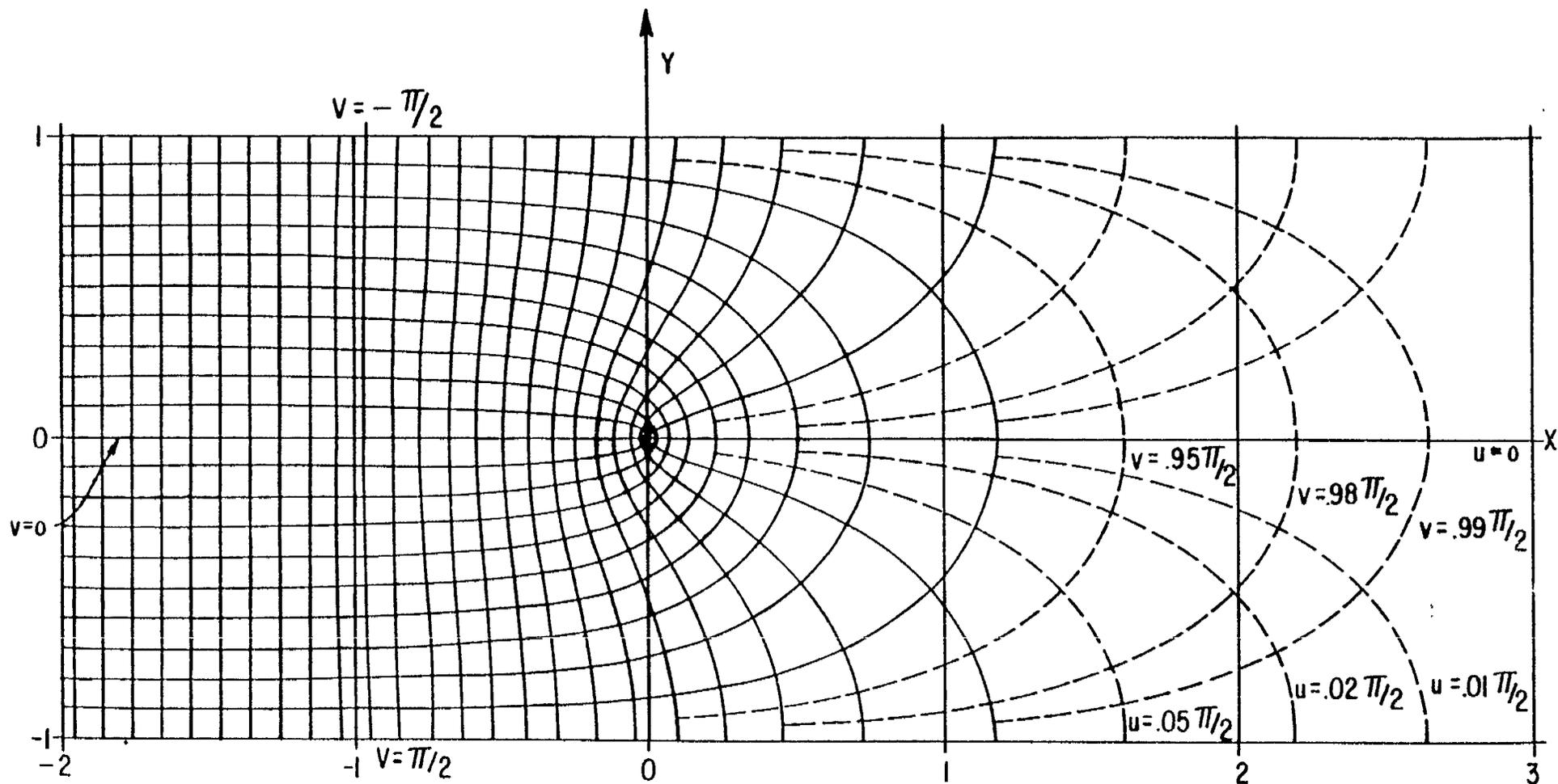
FIGURE 2. FIELD AND POTENTIAL DISTRIBUTION WITH SEMI-INFINITE CENTER CONDUCTOR IN INFINITE THREE CONDUCTOR PARALLEL-PLATE TRANSMISSION LINE
