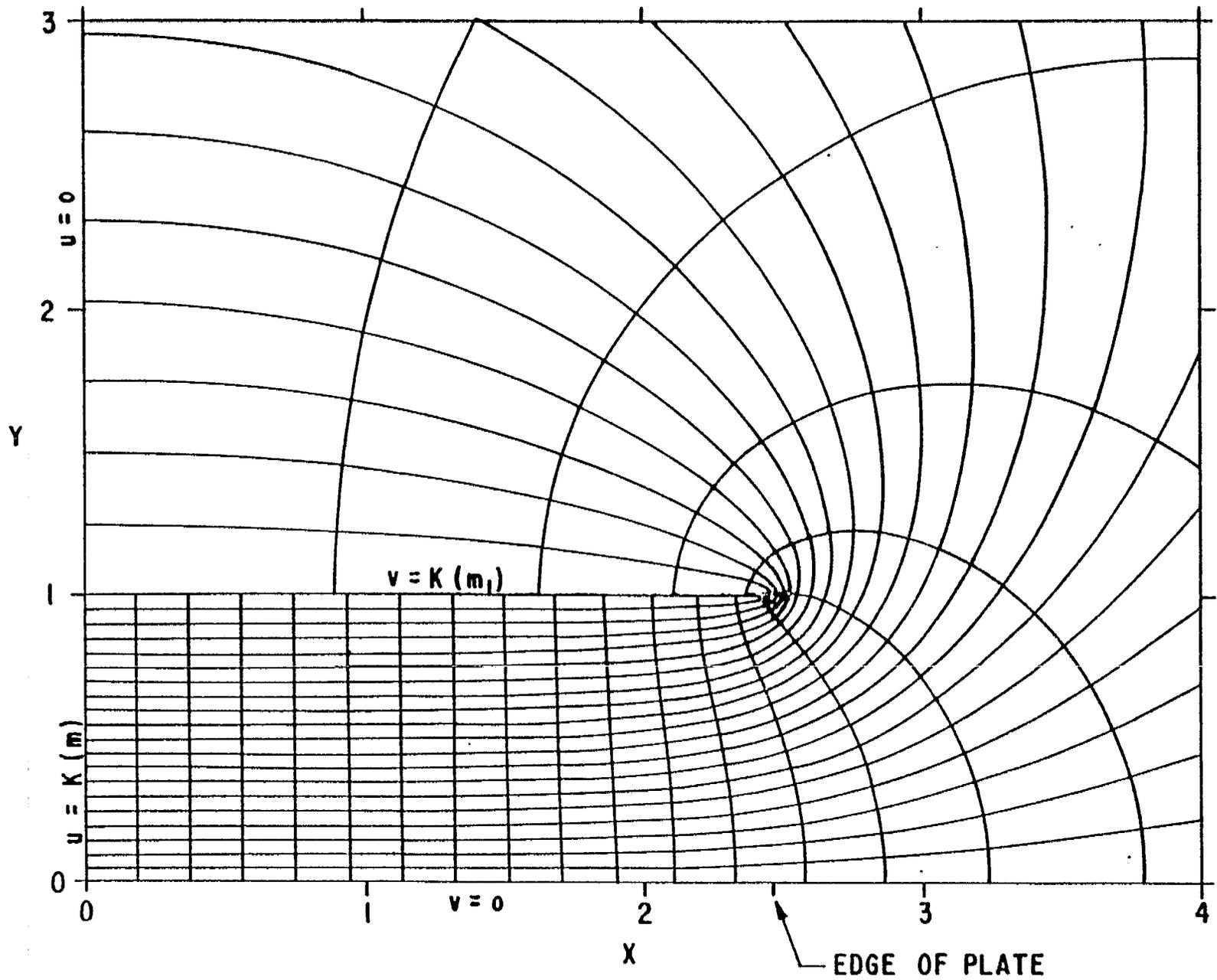
FIGURE II. FIELD AND POTENTIAL DISTRIBUTION FOR PARALLEL, TWO-PLATE TRANSMISSION LINE:  $100 \Omega$
