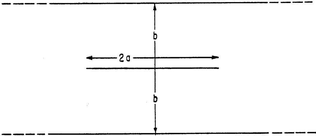
A. INFINITE OUTER PLATES, THREE CONDUCTOR, PARALLEL PLATE TRANSMISSION LINE
