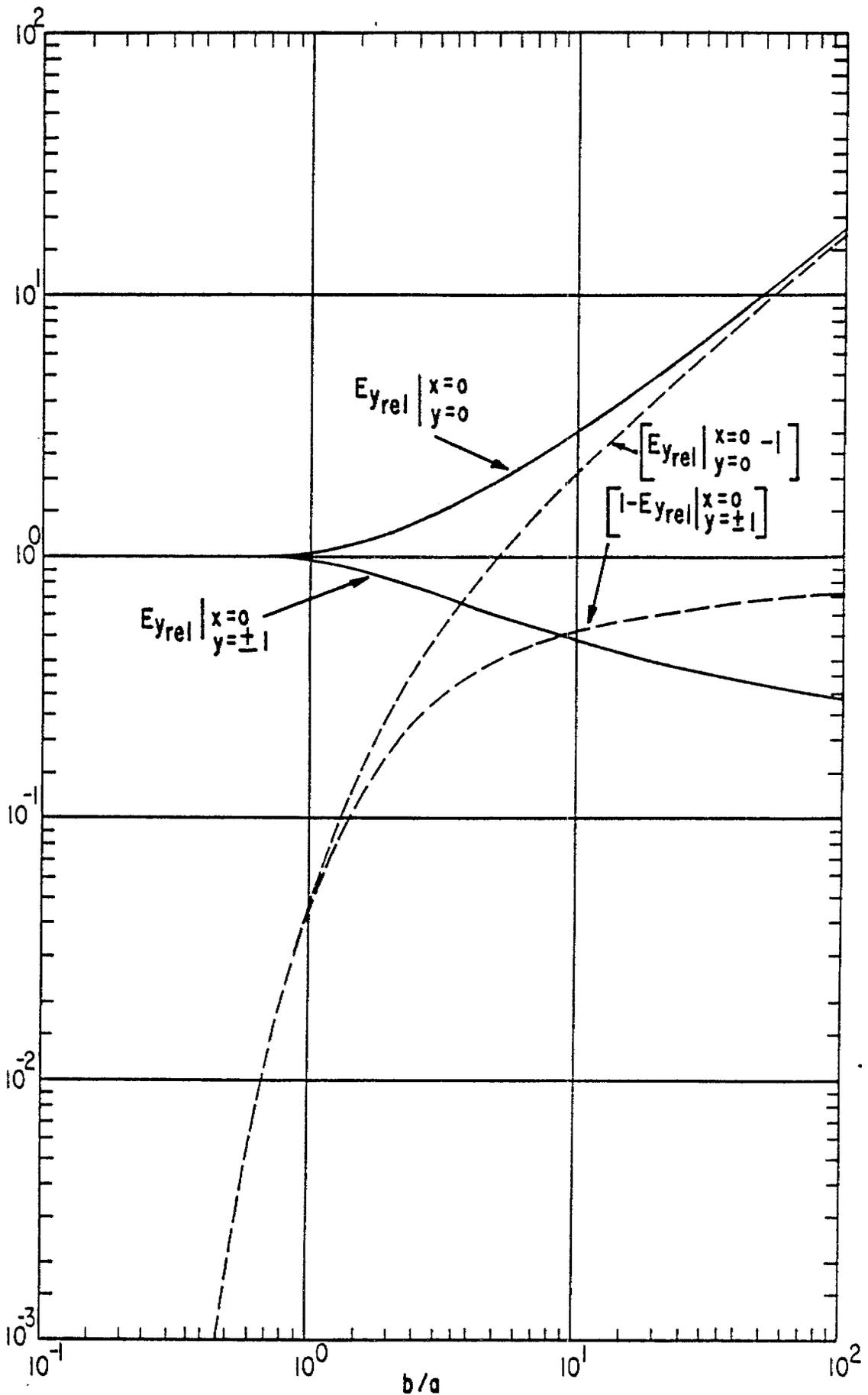
FIGURE 7. NORMALIZED FIELD VARIATION FOR FINITE CENTER CONDUCTOR IN INFINITE THREE CONDUCTOR, PARALLEL PLATE TRANSMISSION LINE
