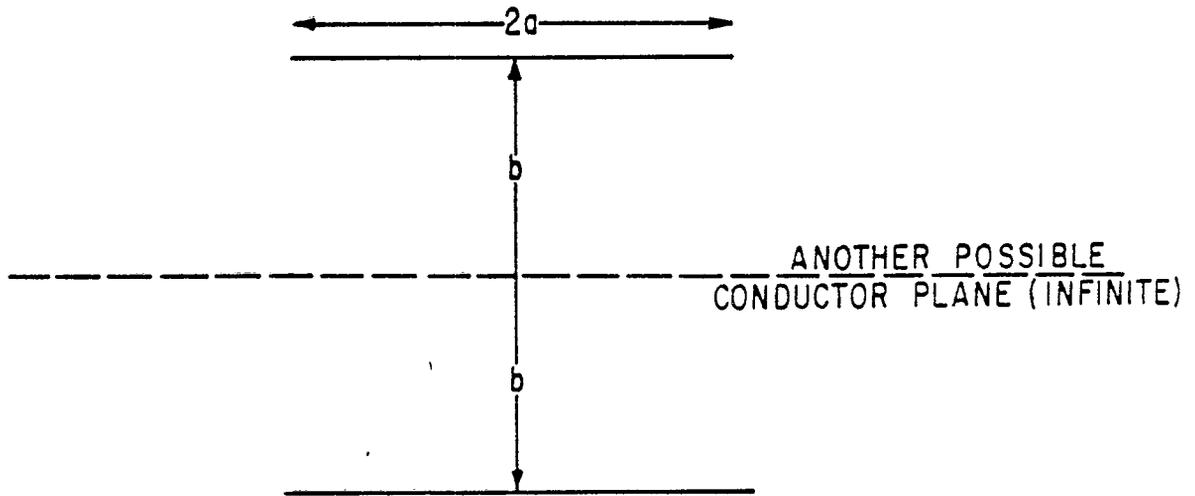
B. TWO CONDUCTOR, PARALLEL PLATE TRANSMISSION LINE
