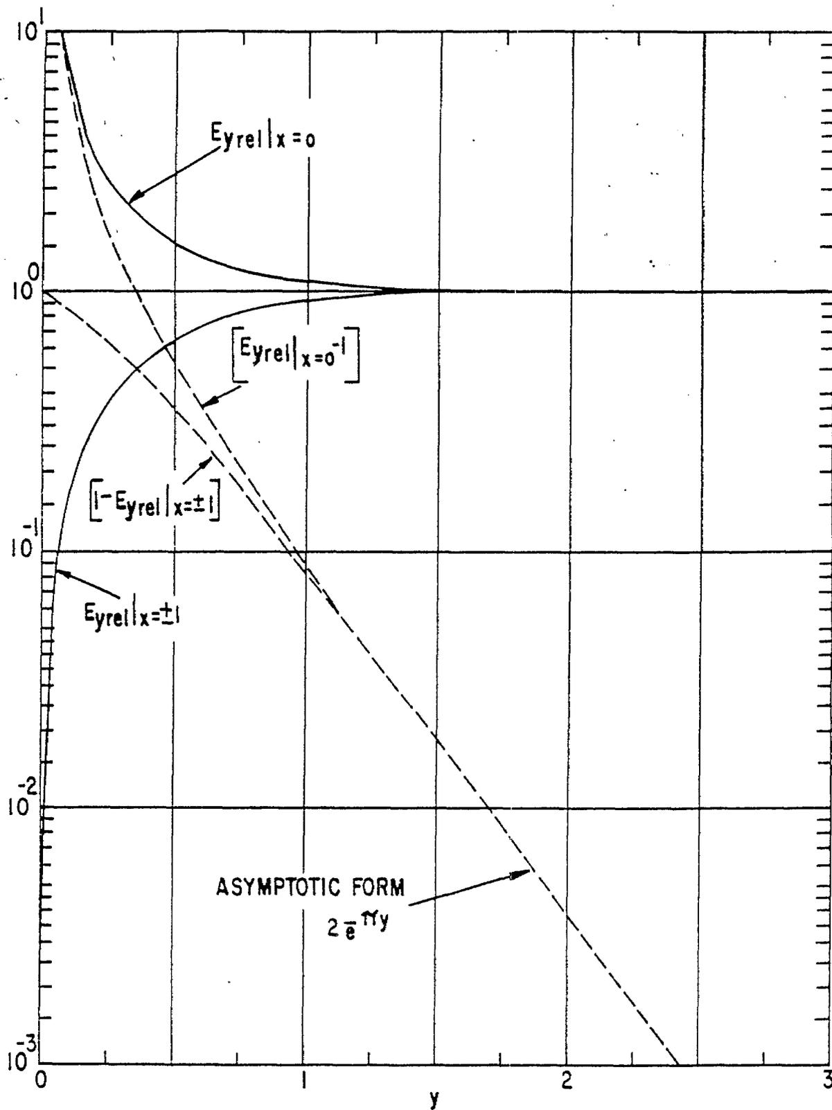
FIGURE 18. NORMALIZED FIELD DISTRIBUTION FOR WIRE GRID TERMINATING EQUAL AND OPPOSITE UNIFORM FIELDS ON BOTH SIDES OF GRID
