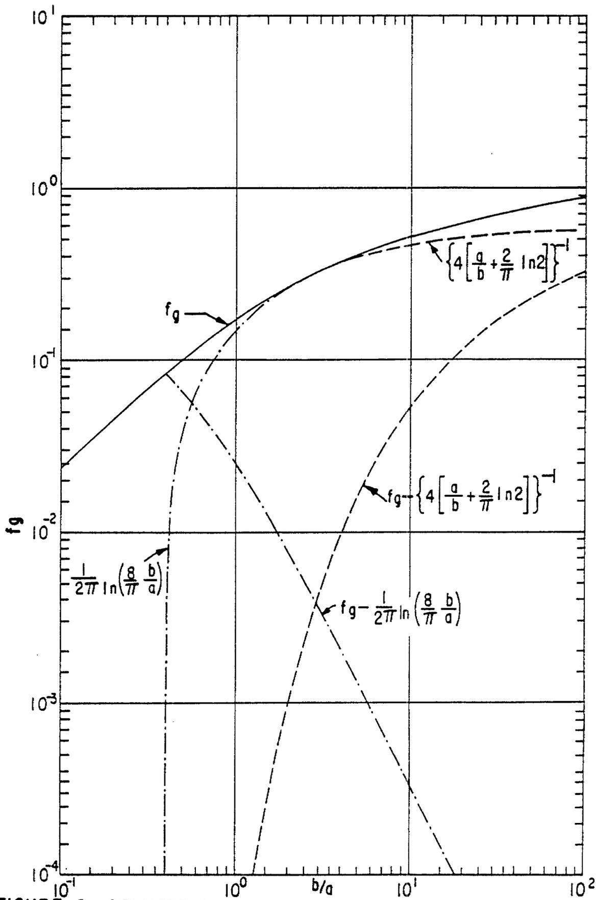
FIGURE 6. GEOMETRIC IMPEDANCE FACTOR FOR FINITE CENTER CONDUCTOR IN INFINITE THREE CONDUCTOR, PARALLEL PLATE TRANSMISSION LINE
