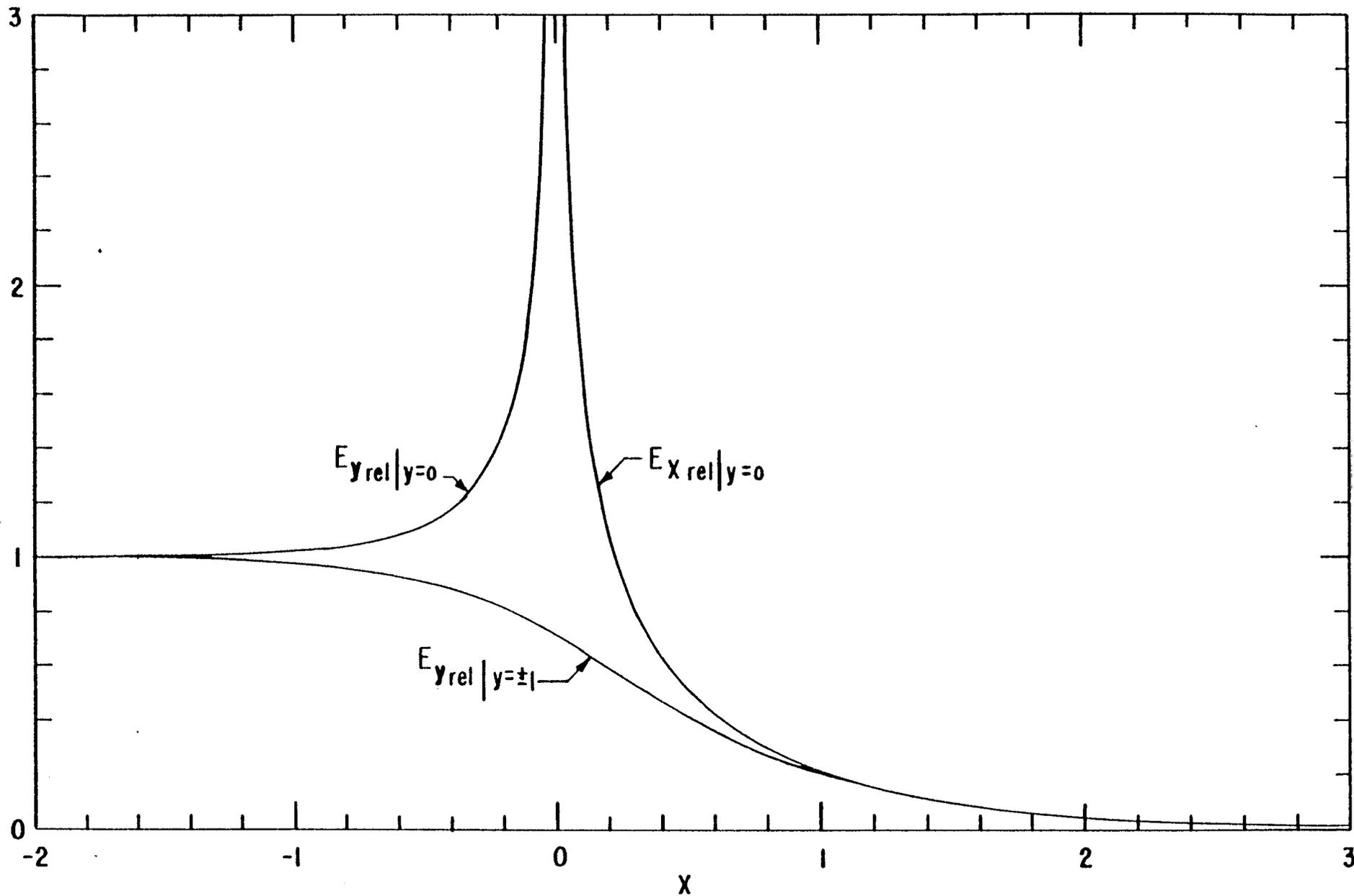
FIGURE 3. NORMALIZED FIELD DISTRIBUTION WITH SEMI-INFINITE CENTER CONDUCTOR IN INFINITE THREE CONDUCTOR PARALLEL PLATE TRANSMISSION LINE
