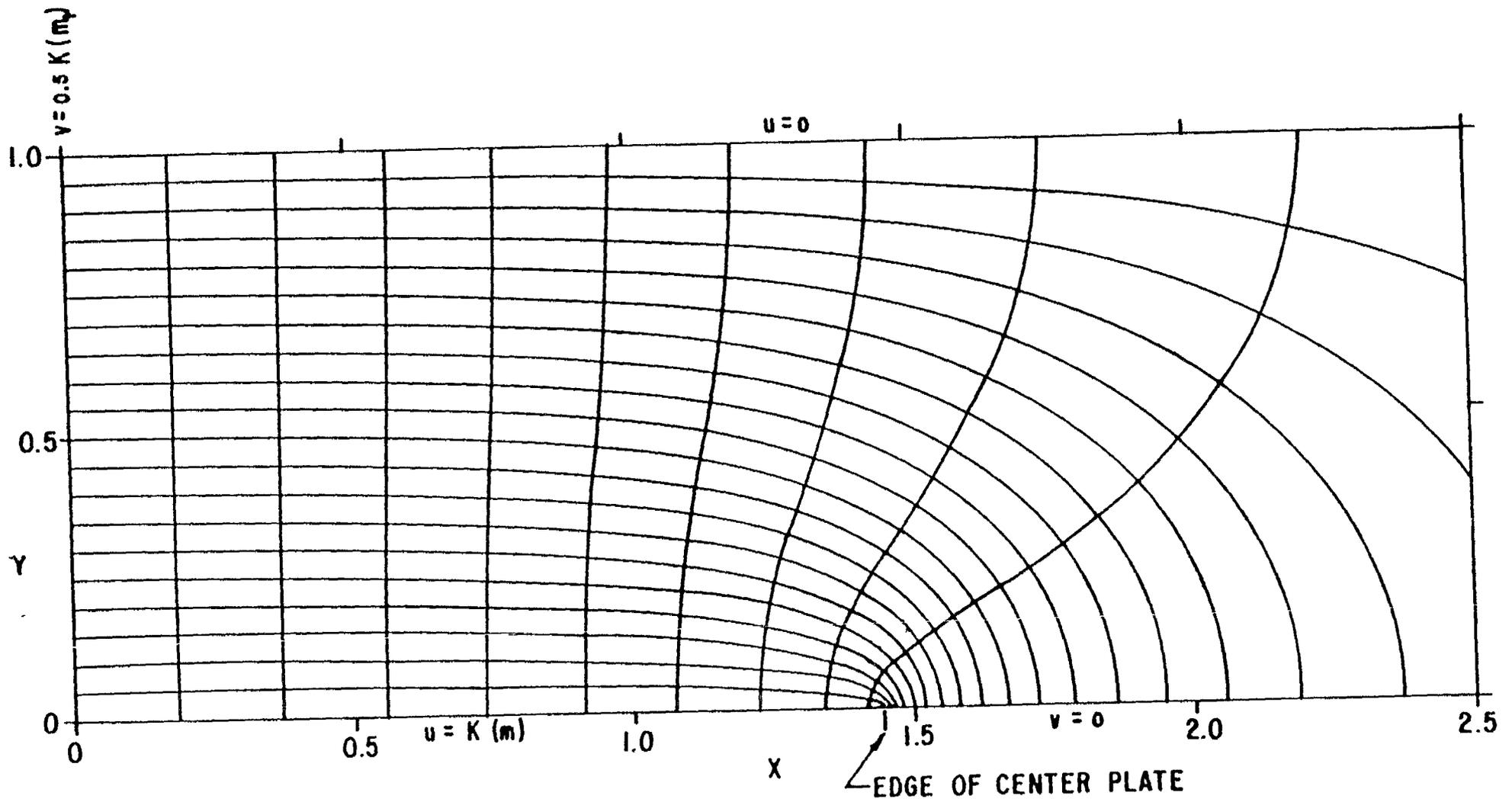
FIGURE 5. FIELD AND POTENTIAL DISTRIBUTION FOR FINITE CENTER CONDUCTOR IN INFINITE THREE CONDUCTOR PARALLEL-PLATE TRANSMISSION LINE:  $50\Omega$
