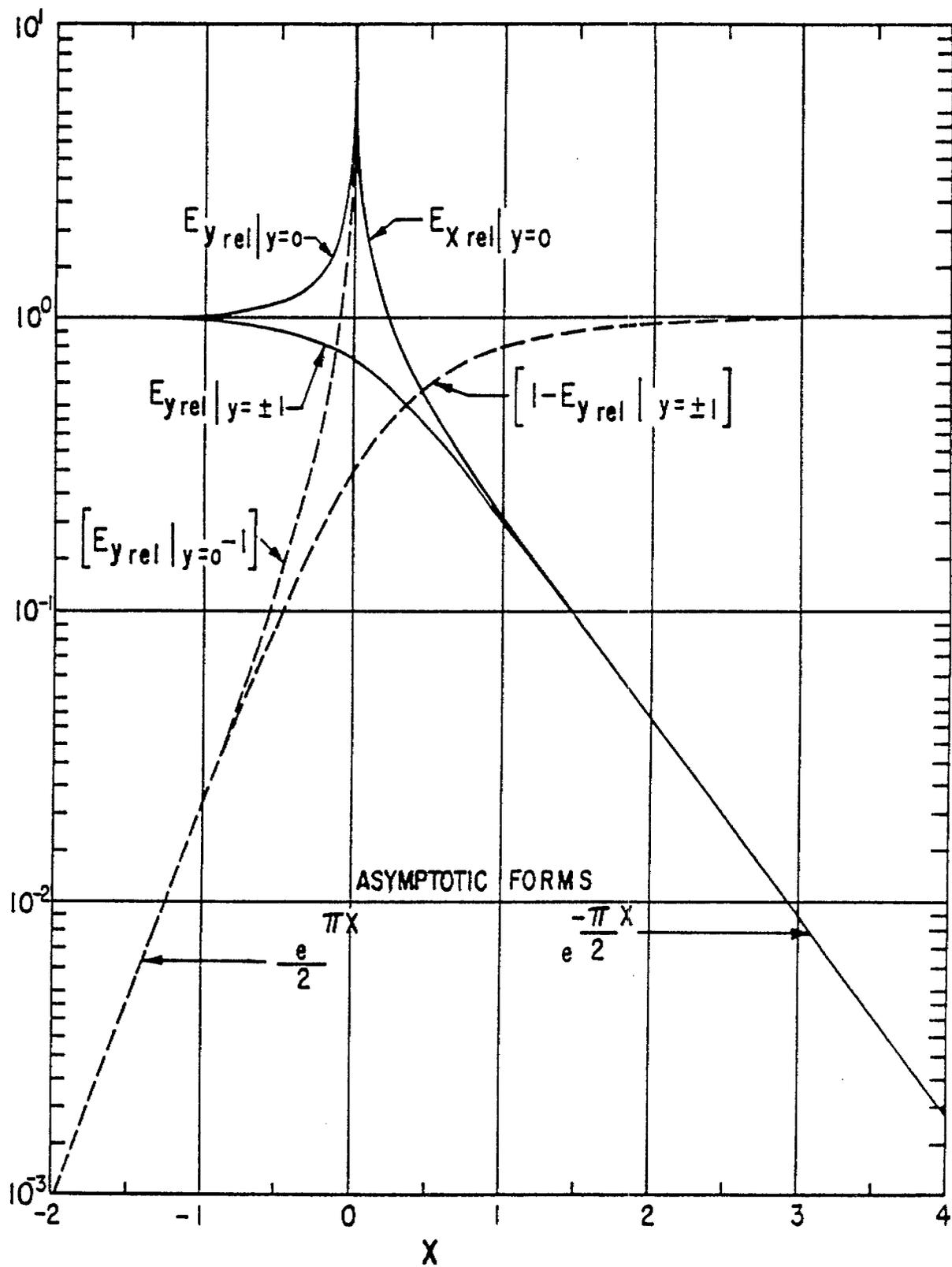
FIGURE 4. NORMALIZED FIELD DISTRIBUTION WITH SEMI-INFINITE CENTER CONDUCTOR IN INFINITE THREE CONDUCTOR PARALLEL PLATE TRANSMISSION LINE
