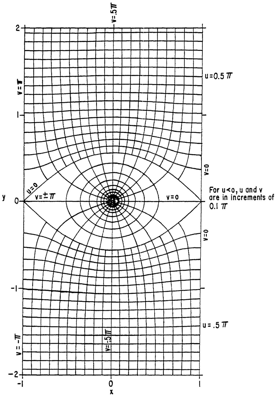
FIGURE 17. WIRE GRID (ONE CELL) TERMINATING EQUAL AND OPPOSITE UNIFORM FIELDS ON BOTH SIDES OF GRID
