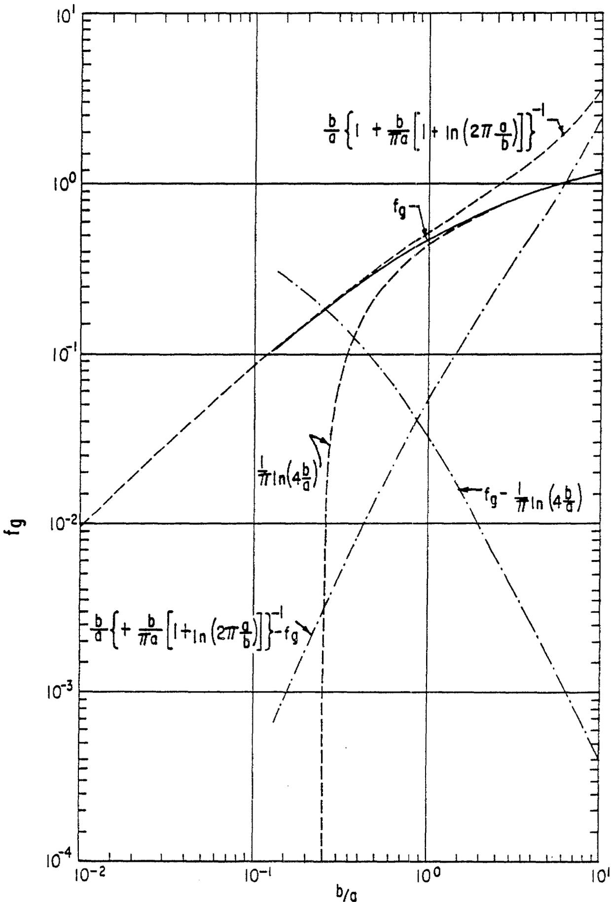
FIGURE 12. GEOMETRIC IMPEDANCE FACTOR FOR FINITE, SYMMETRICAL, TWO PLATE TRANSMISSION LINE
