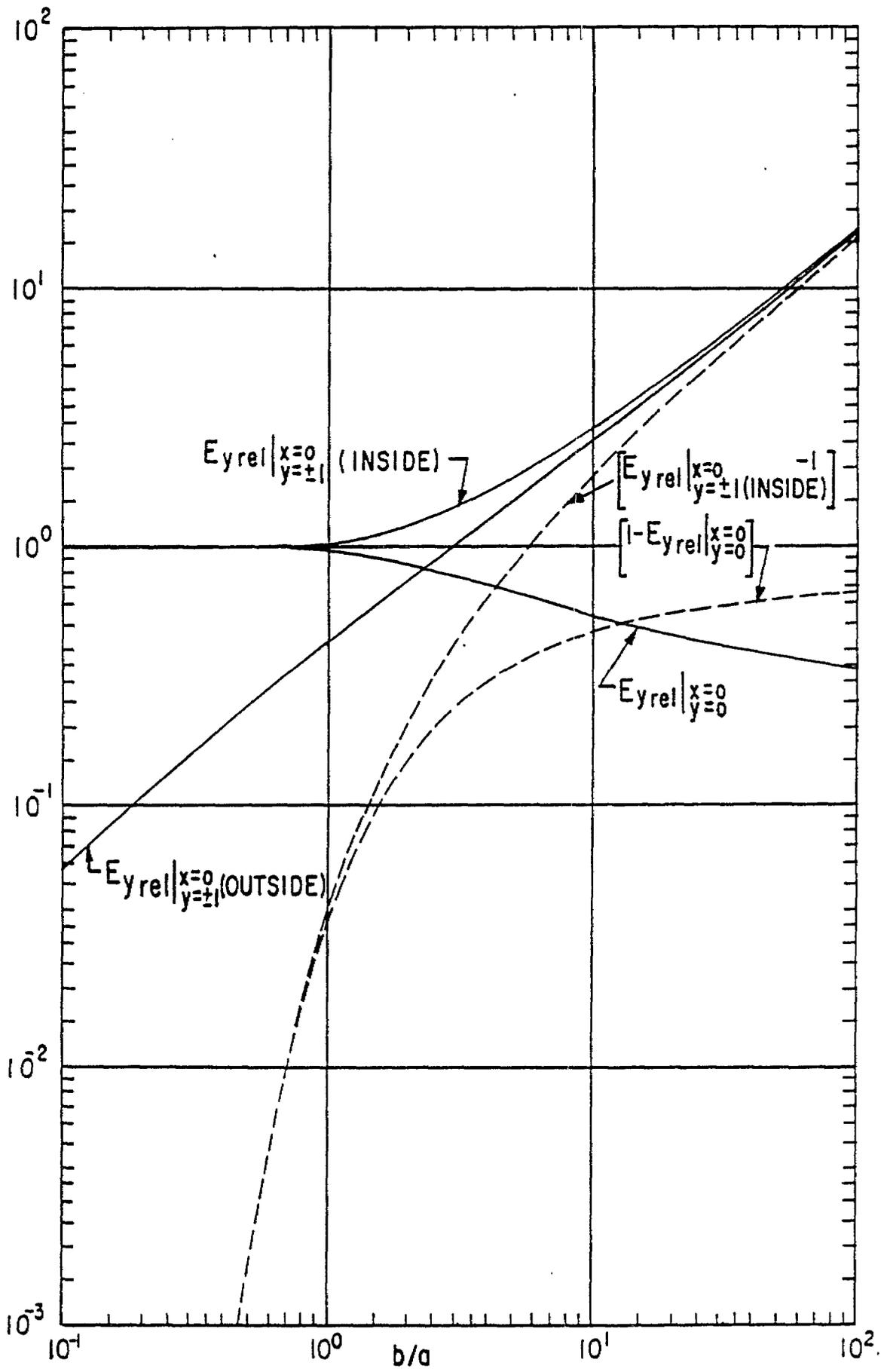
FIGURE 13. NORMALIZED FIELD VARIATION FOR FINITE, SYMMETRICAL, TWO PLATE TRANSMISSION LINE
