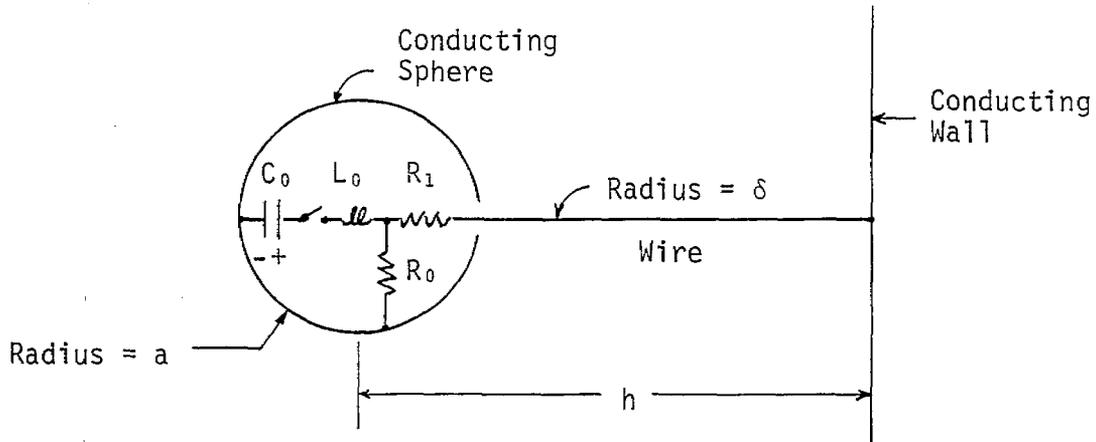
Figure 1. Basic scheme for use of self-contained pulser.
