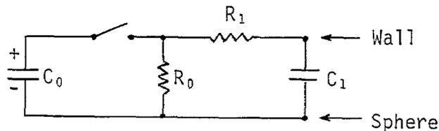
Figure 2. Approximate equivalent circuit for Figure 1.
