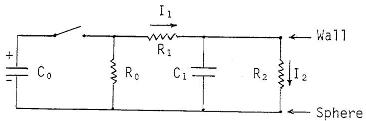
Figure 4. Equivalent circuit for modification I.
