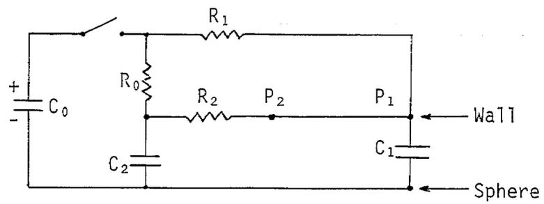
Figure 6. Equivalent circuit of modification II.
