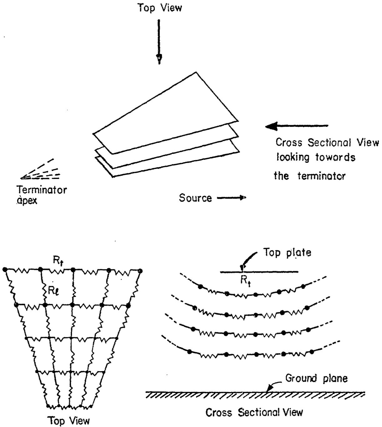
Figure 5.1 Structure of the volumetric spatial modal filter
