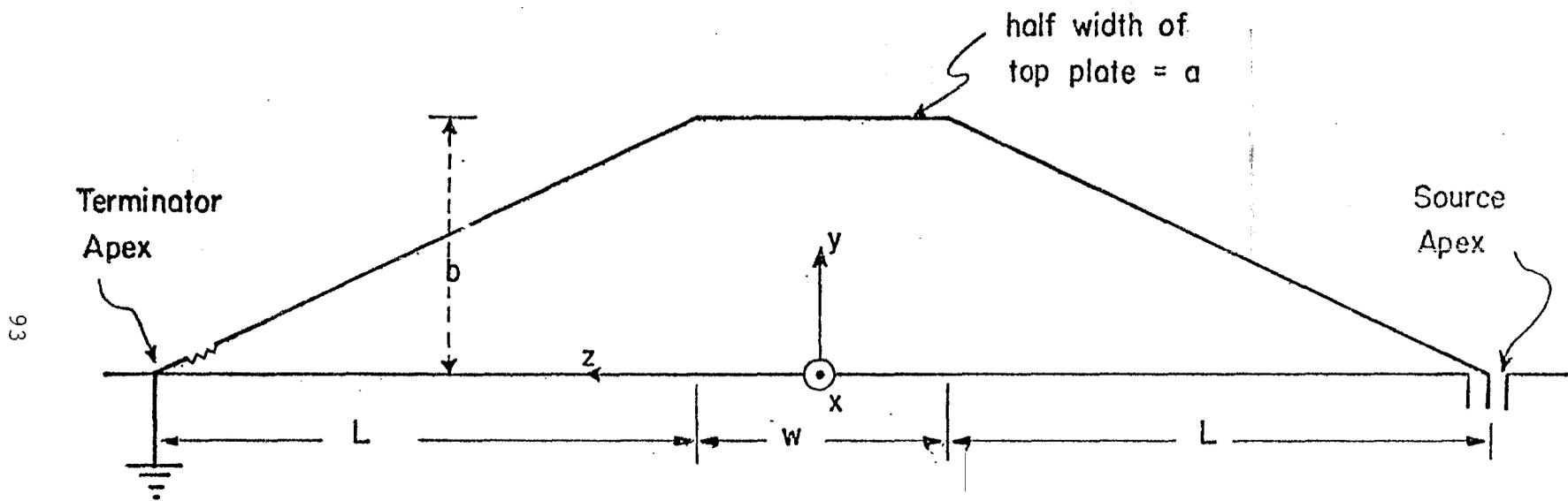
Figure 2.1 Geometry of a vertically polarized, two-parallel plate transmission-line type of EMP simulator
