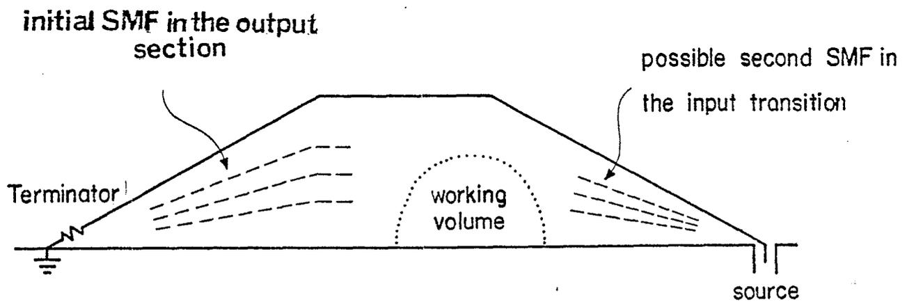
Figure 6.1 Side view of the simulator showing the approximate locations of two possible spatial modal filters (SMF)
