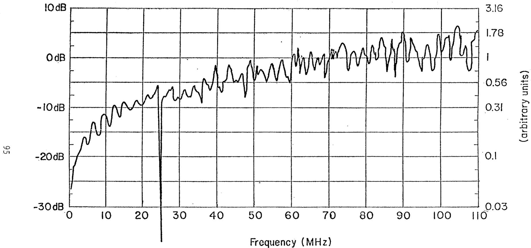
Figure 2.2 Measured  $|\dot{B}_x/\text{constant}|$  at the center with coordinates  $(0,0,0)$  in ALECS facility
