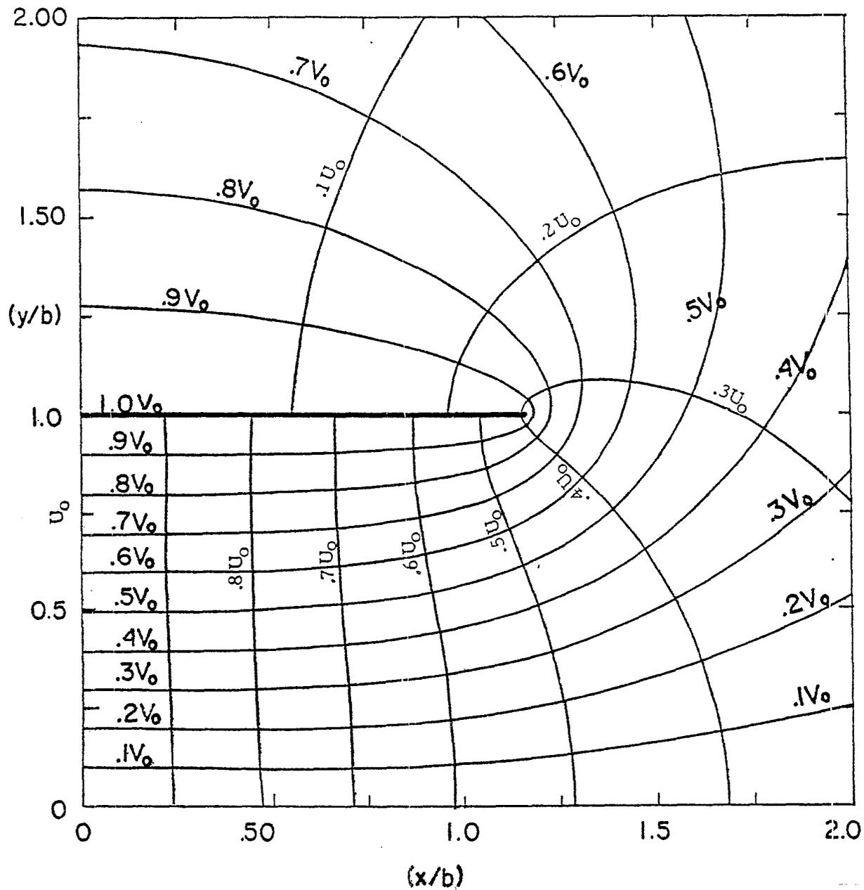
Figure 5.2 A typical TEM equipotential and electric field lines in the conical transmission line [(b/a) = 0.857 and (L/b) = 4.2; scale model simulator with  $z_c^{(TEM)} = 82\Omega$  from top plate to ground plane]
