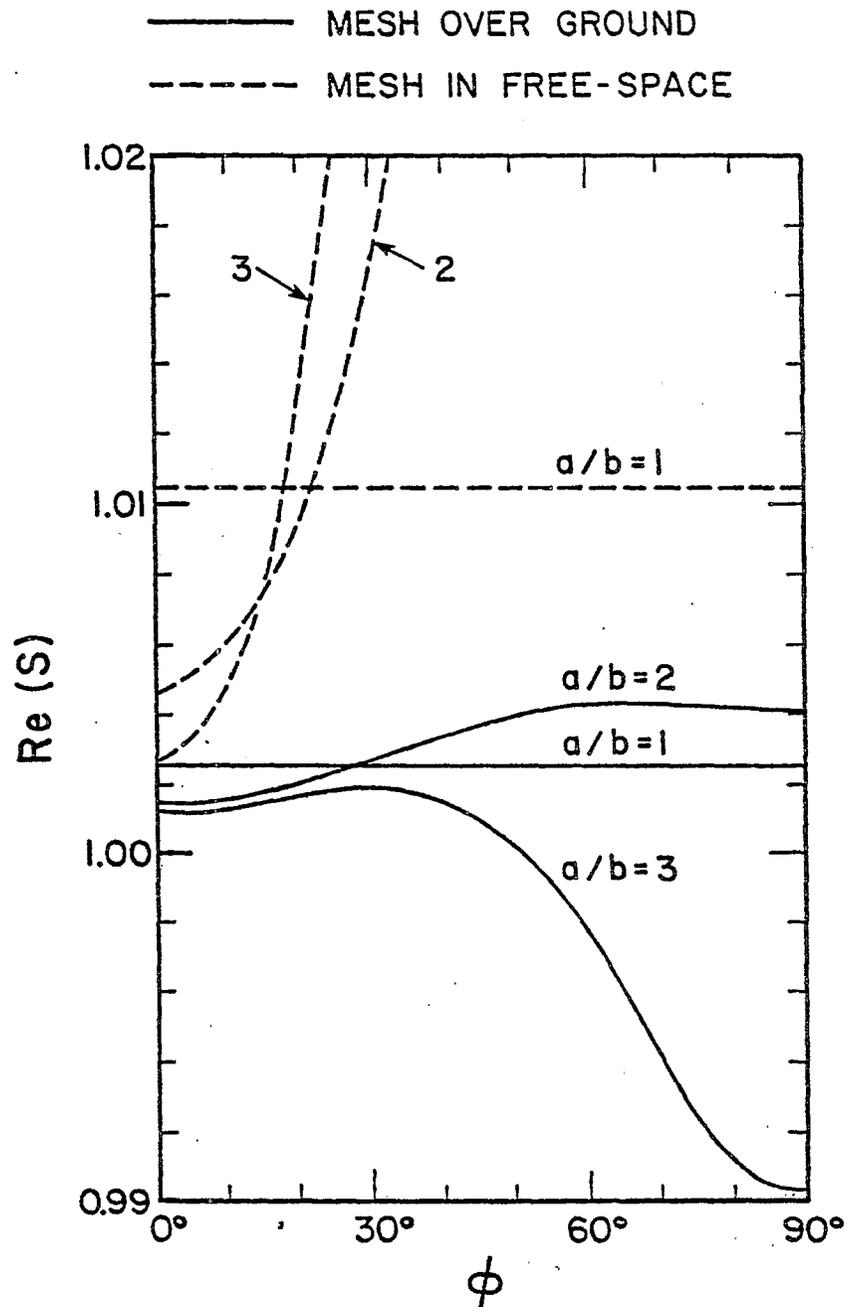
Figure 2. Real part of the normalized propagation constant  $S$  as a function of propagation direction  $\phi$ .
