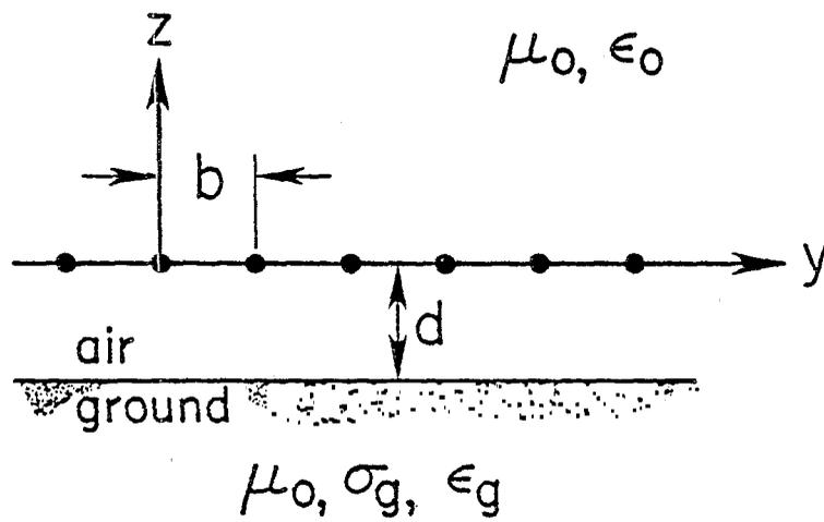
Figure 1. A bonded rectangular wire mesh over a conducting half-space (perspective and side view).
