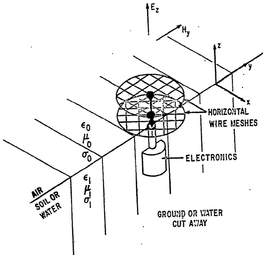
FIGURE 2. PARALLEL WIRE MESH, VERTICAL DIPOLE
