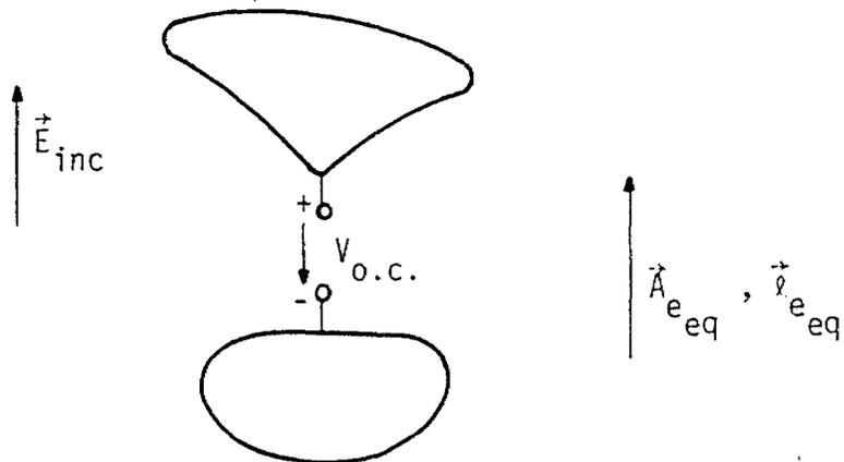
c. Electric Dipole Sensor
