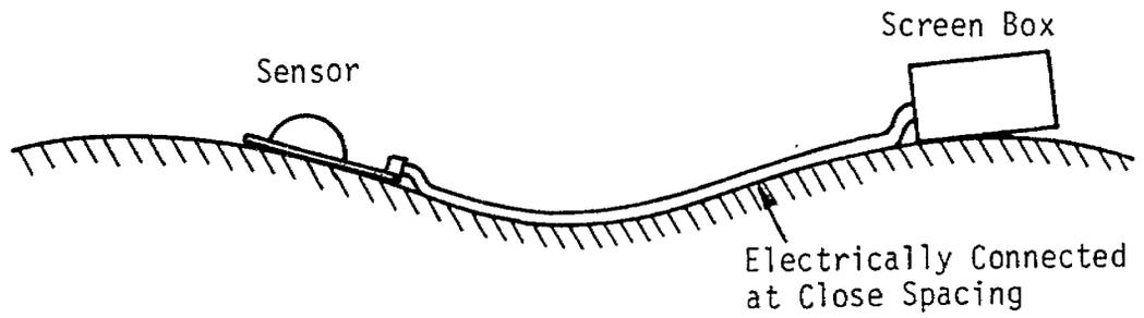
a. Conforming measurement conductors to experiment conductors
