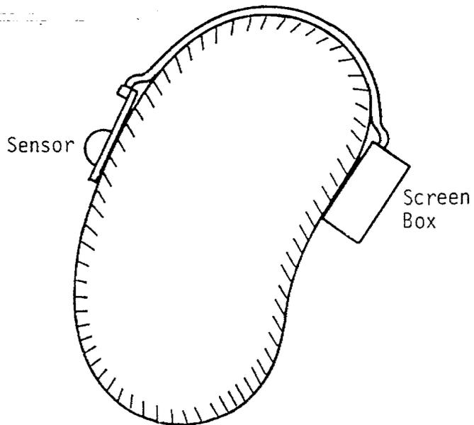
b. "Shadowing" sensor from screen box
