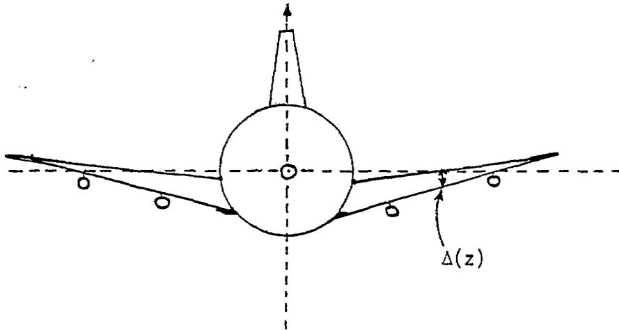
Figure 9a. Nose-on view of aircraft showing the wing and wing-engines thickness parameter  $\Delta(z)$ .
