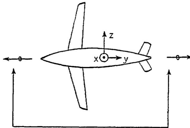
Two possible sensor locations for an antisymmetric incident magnetic field measurement.
