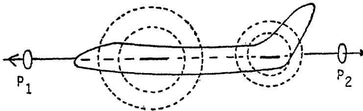
Figure 4. Sensor location and orientation which minimizes coupling from both wing and horizontal stabilizer ( $P_W$  and  $P_H$  coincide with each other and with the incident field quantity to be measured).
