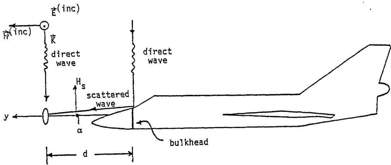
Figure 11. Example geometry for high-frequency scattering estimates.
