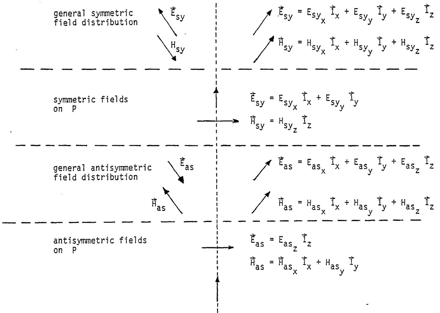
Figure 2. Symmetry plane, coordinate system, symmetric fields and antisymmetric fields.
