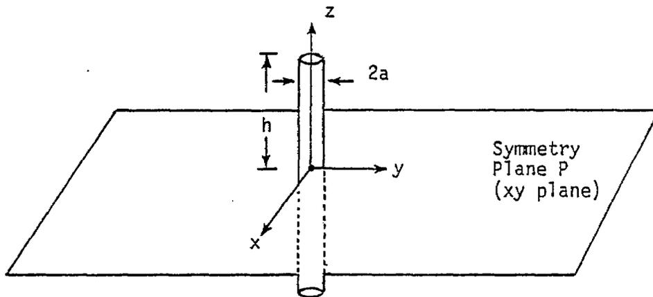
Figure 8. Conducting post model for the wing (or horizontal stabilizer).
