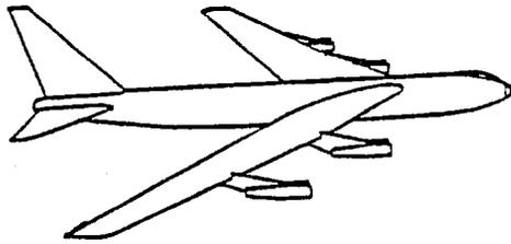
(a) Engines on the wings (aft and forward booms are possible, preferred location has to be determined by calculations or scaled experiments)
