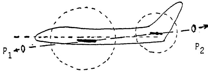
Figure 6. Location  $P_1$  or  $P_2$  such that coupling from both wing and horizontal stabilizer are determined from geometrical calculations and/or scale model experimentation.
