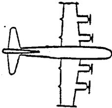
(b) Engines on the wings & wings forward (aft or tail boom)
