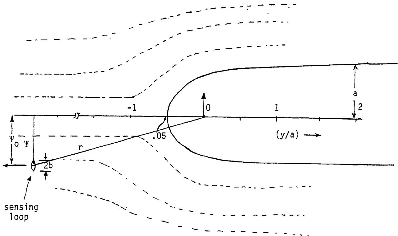
Figure 10(b). Scattering model for fuselage
