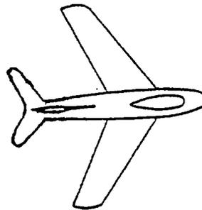
(c) Jet engine along fuselage axis (forward or nose boom)
