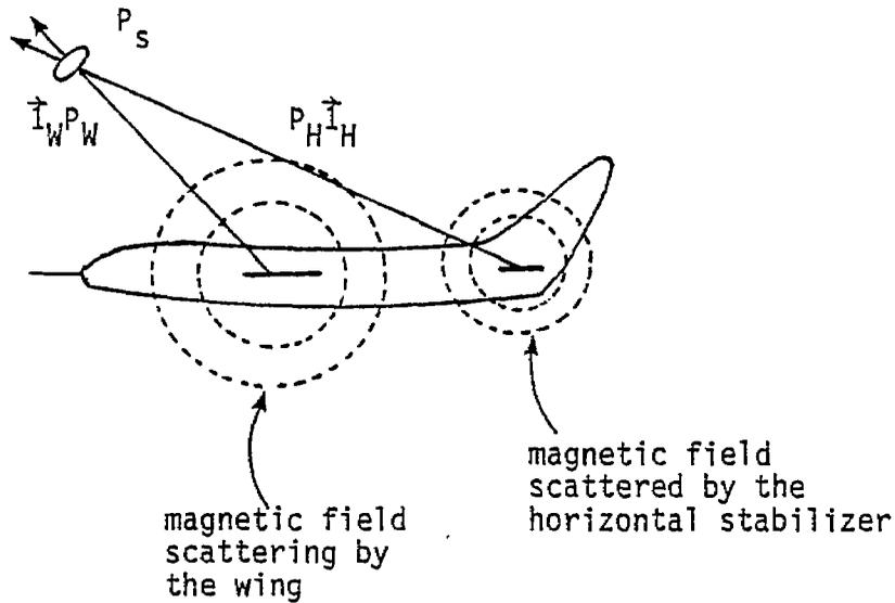
Figure 3. A general location and orientation for sensor where the wing scattering or the horizontal stabilizer scattering can be minimized, by orienting the sensor axis along  $P_W$  or  $P_H$ .
