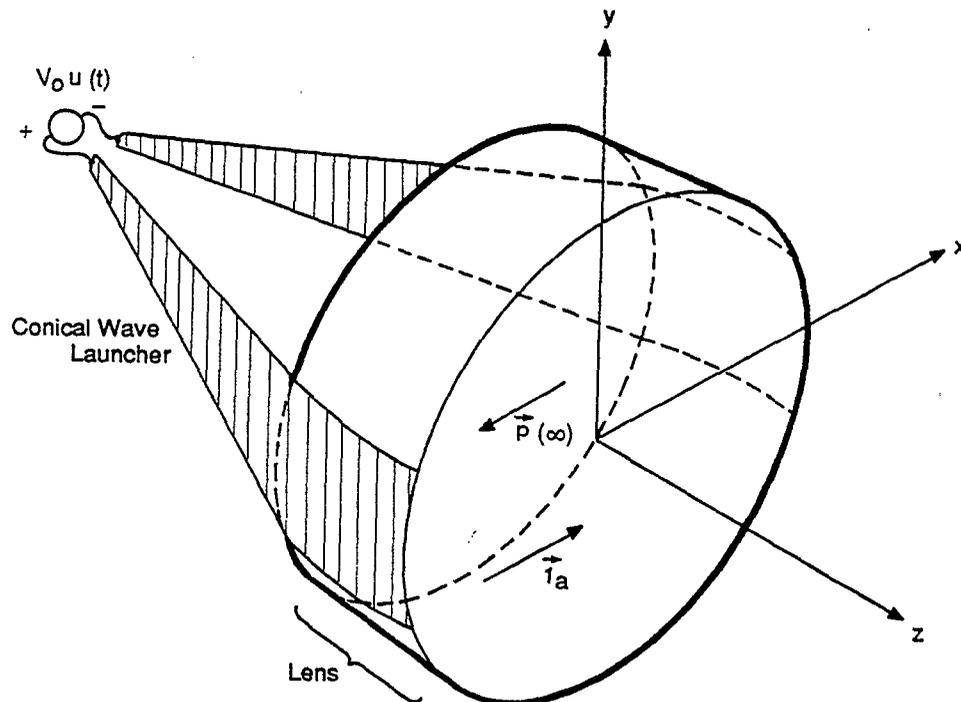
Figure 4.1. TEM Horn and Lens as Wave Launcher
