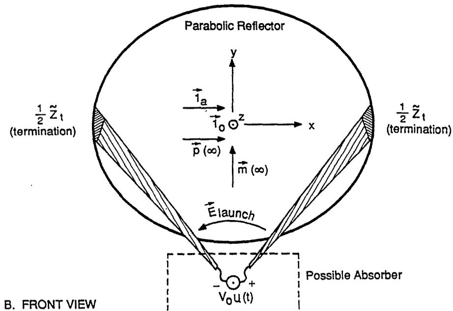
Figure 5.1. Conical TEM Wave Launcher Feeding Reflector
