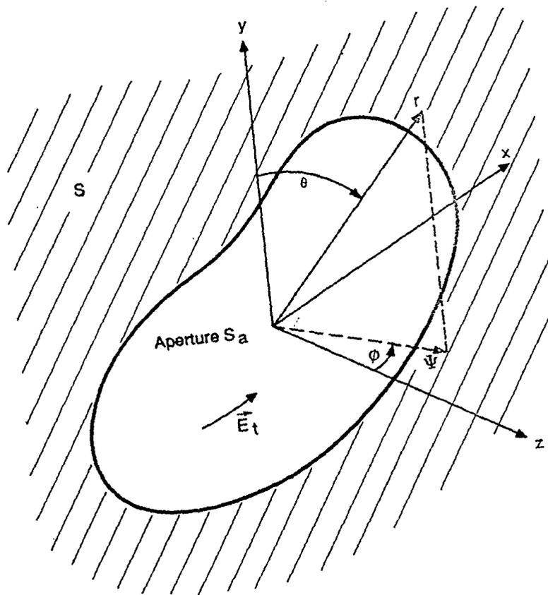
Figure 2.1. Aperture Antenna with Specified Tangential Electric Field
