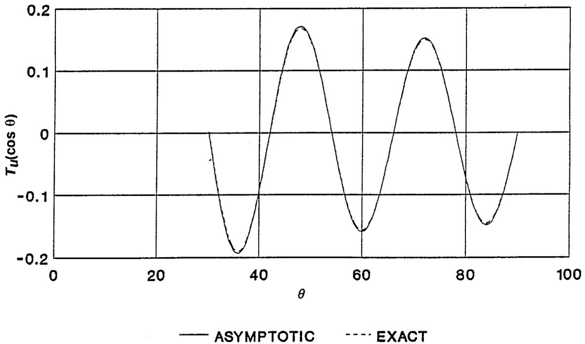
Figure A-12. Comparison between asymptotic and exact  $T_U$  for  $\theta_0 = 30^\circ$  and  $m = 5$ .
