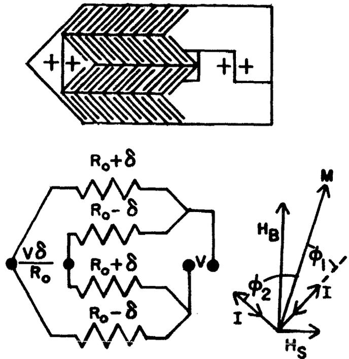
Figure 1. Pattern of Wheatstone bridge used to etch film with an equivalent circuit showing resistances for the given field configuration. The black lines on the pattern refer to locations where the film is etched away. The crosses correspond to lead connections, or to dots on the equivalent circuit.
