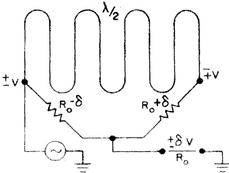
Figure 2. Photo and equivalent circuit of a bridge which needs only two connections and operates with a 300 MHz carrier.
