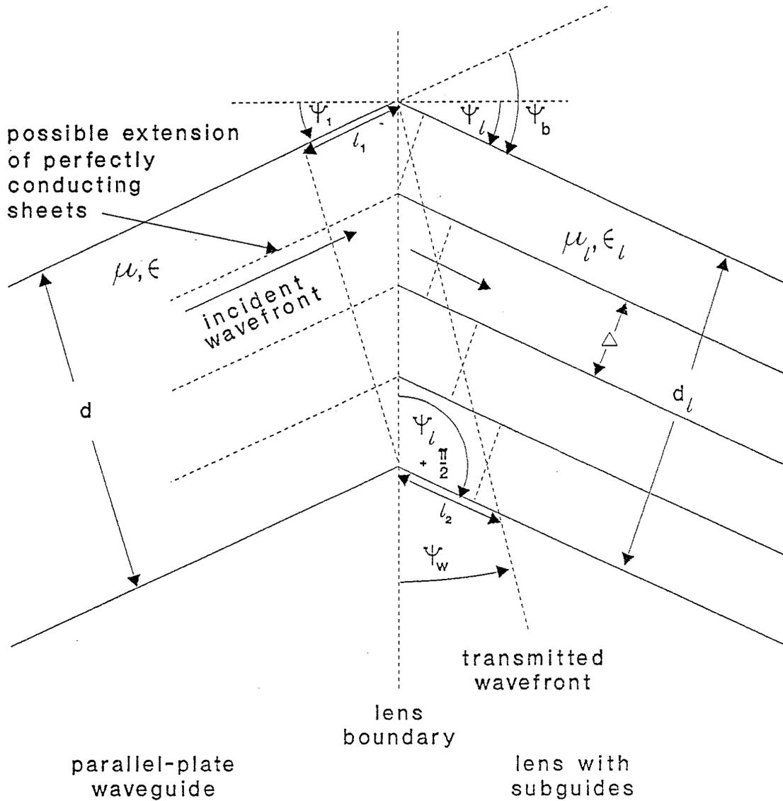
Fig. 2.2 Matched Transmission of TEM Wave at Bend from Parallel-Plate Region to Lens Region
