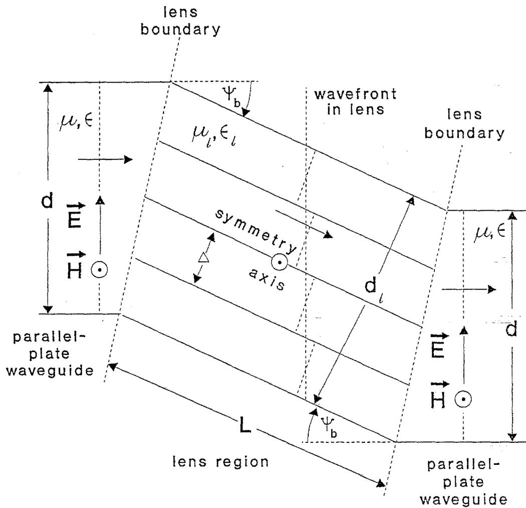
Fig. 3.1 Lateral Displacement Lens
