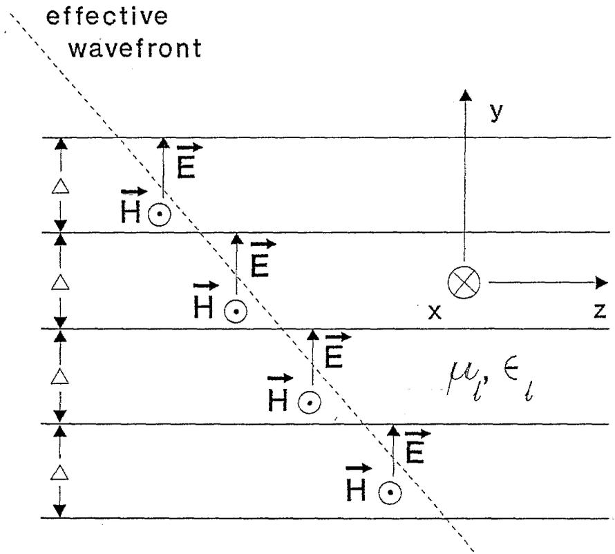
Fig. 2.1 Skewed TEM Wave Propagating on Set of Parallel Perfectly Conducting Sheets
