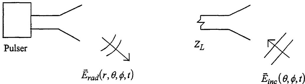
Figure 4.1. The antenna and pulser in transmission, and the antenna and load in reception.
