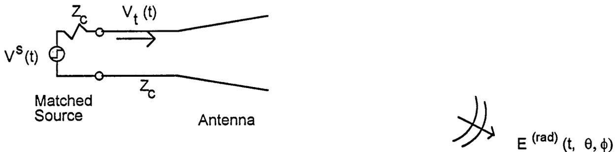
Figure 5.1. A transient antenna in transmit mode.
