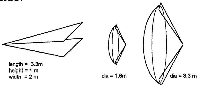
Figure 9.1. Three antennas for comparing transient gains.
