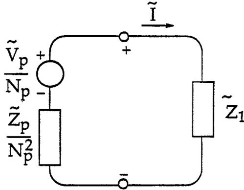
Figure 4.1. Equivalent Circuit of Pulser with Ideal Transformer.
