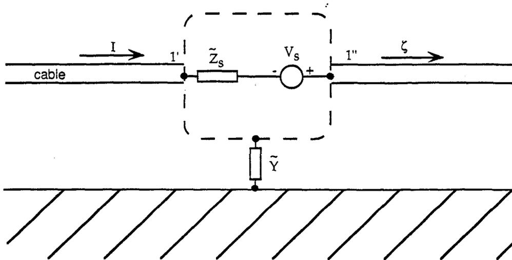
Fig. 3.1. Insertion of a Local Equivalent Source
