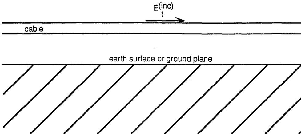
B. Cable above a conducting medium (e.g., lossy earth or a ground plane)
