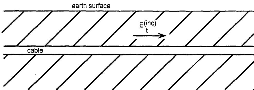
C. Cable buried near surface of conducting medium
