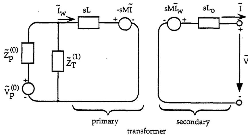
Figure 4.3. Equivalent Circuit of Pulser with Inductive Coupler (Simplified)
