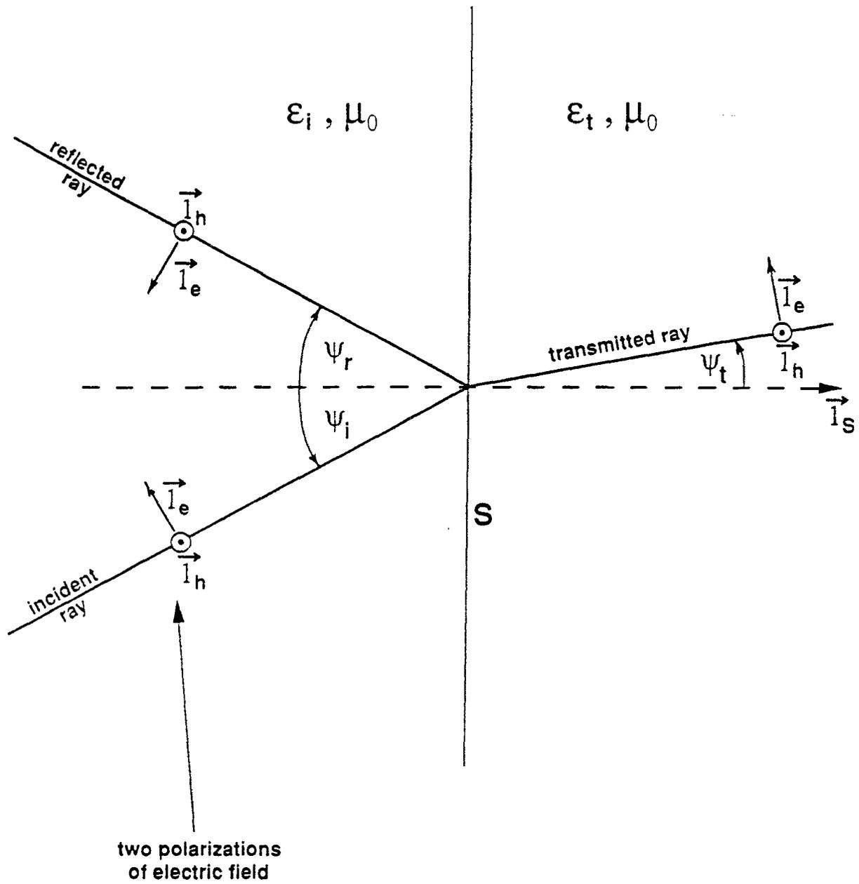
**Fig. 2.1: Transmission and Reflection of Plane Wave at Interface Between Two Dielectric Media**
