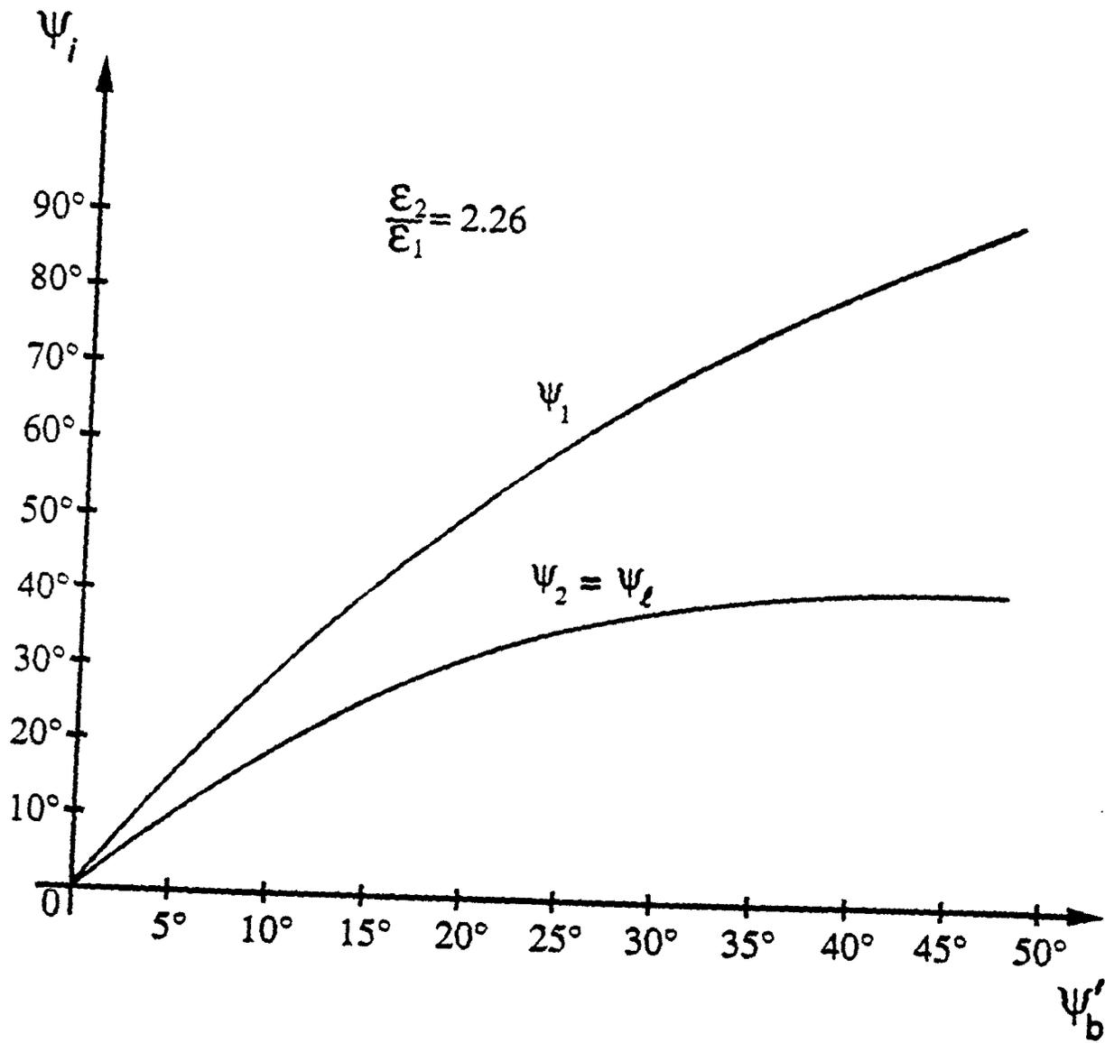
**Fig. 4.2: Lens Angles for Particular Permittivity Ratio**
