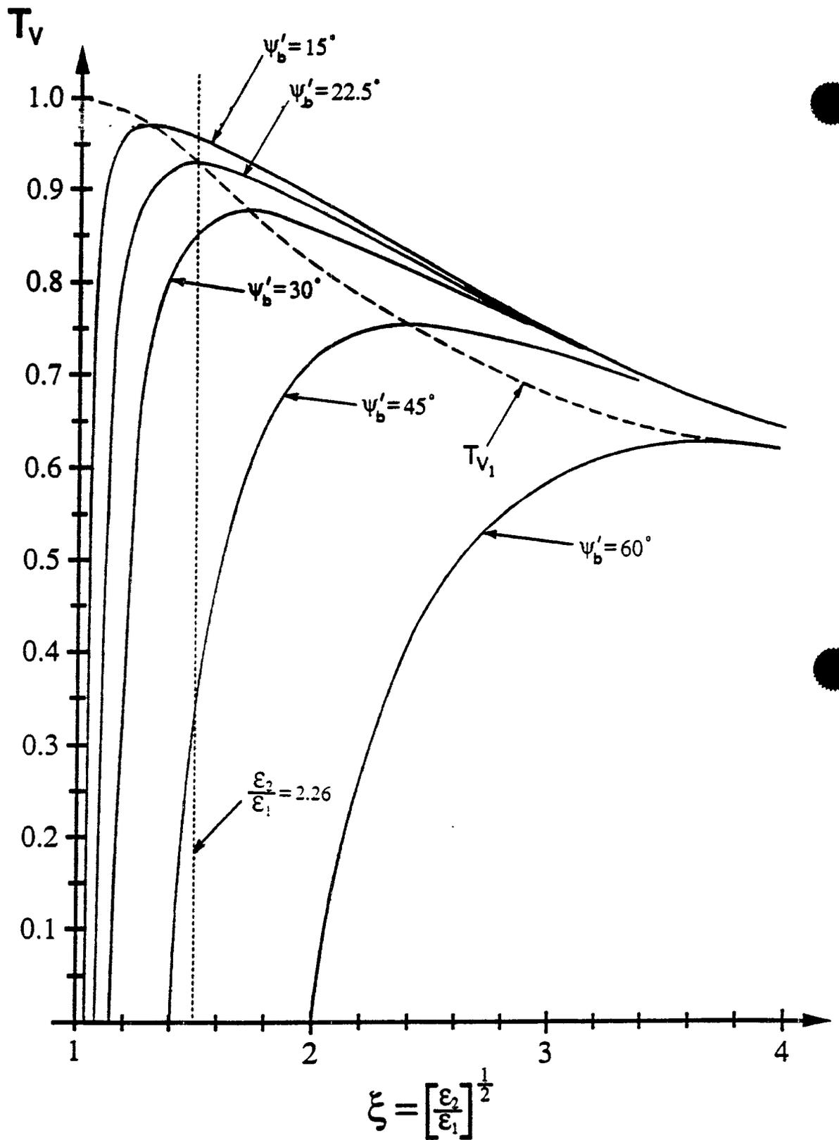
Fig. 4.1: Initial Transmission of TEM Mode
