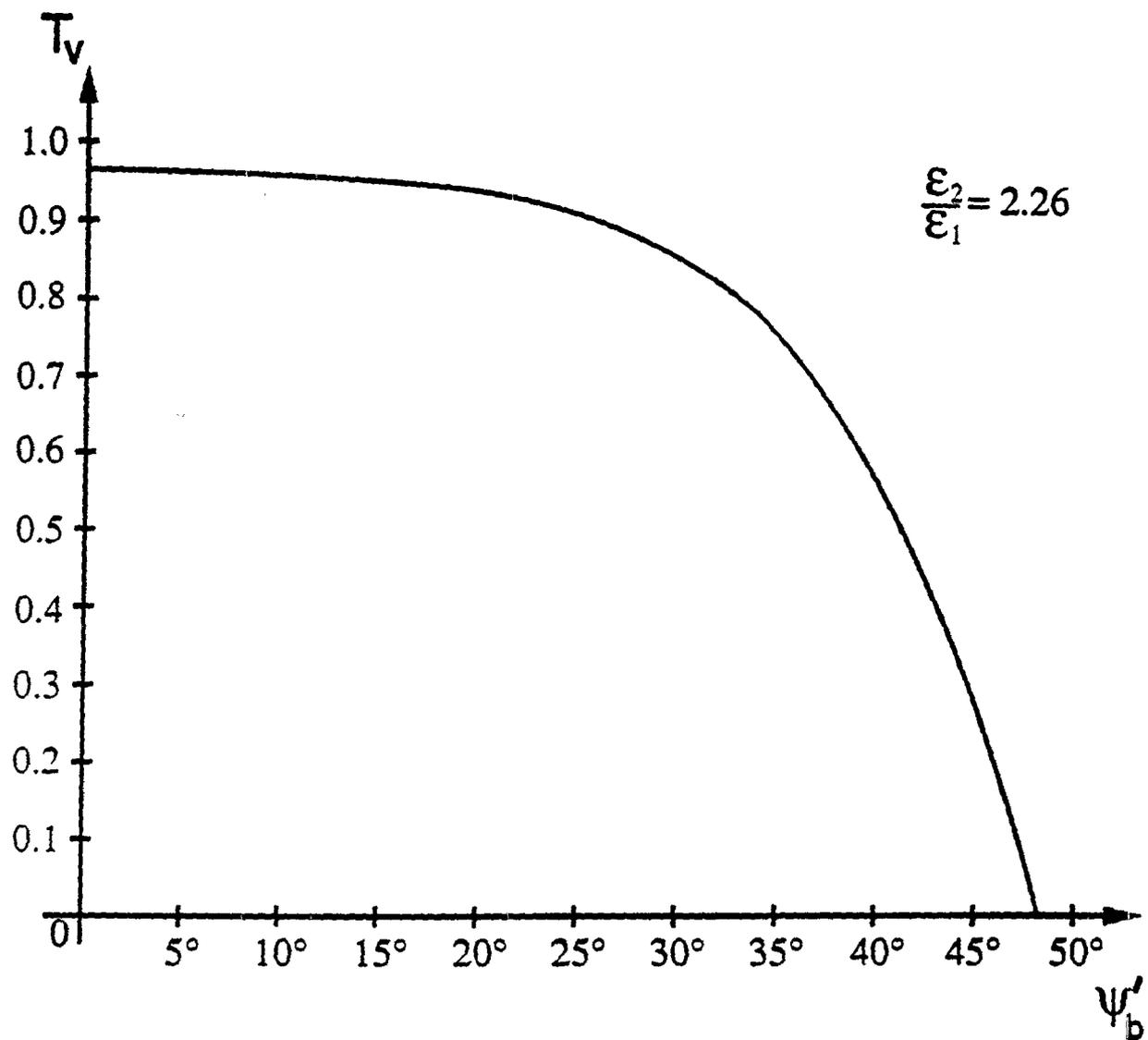
**Fig. 4.3: Initial TEM Transmission for Particular Permittivity Ratio**
