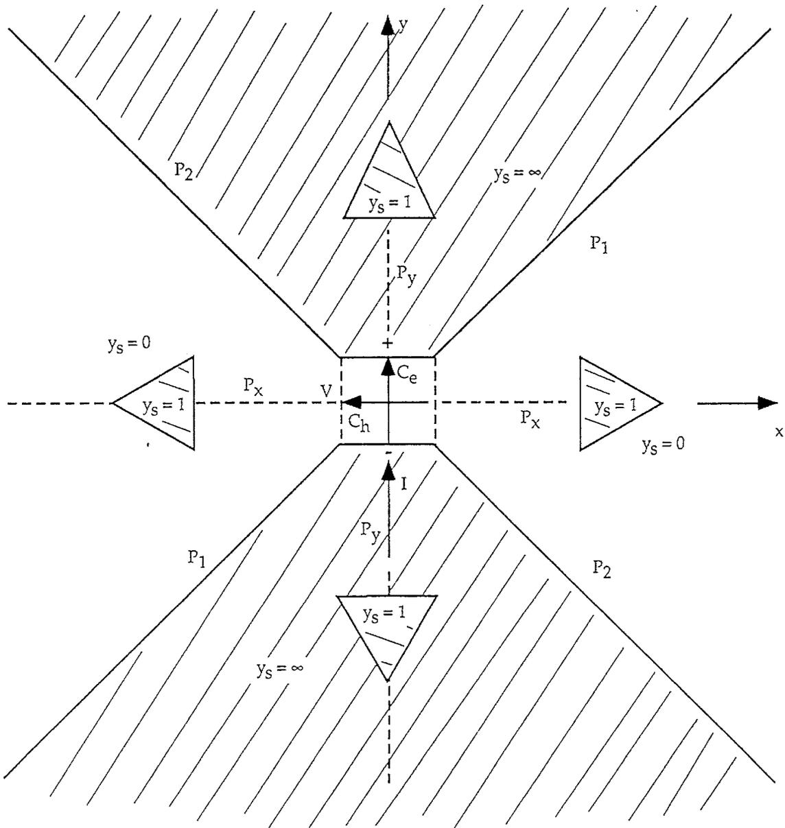
Fig. 3.2.  $C_{2ac}$  Self-Complementary Antenna
