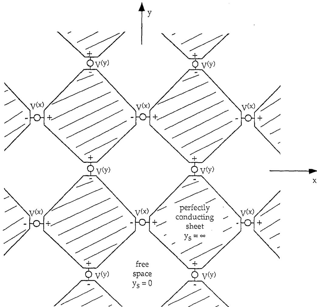
Fig. 6.1. Planar Array with  $C_{2ac}$  Symmetry and Dual Polarization
