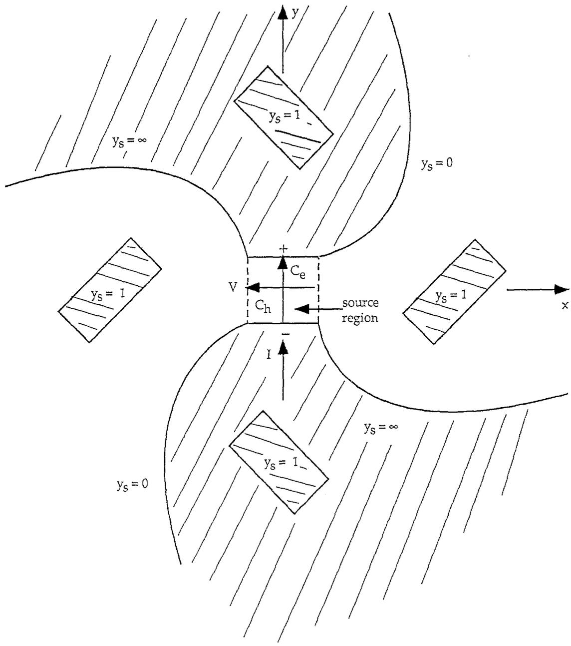
Fig. 3.1.  $C_{2c}$  Self-Complementary Antenna
