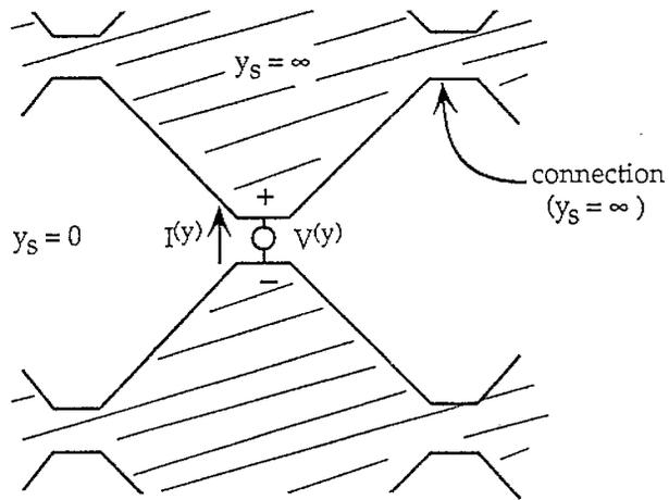
A. Array with connection (zero impedance) at corners
