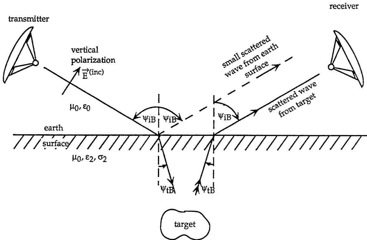
Fig. 3.1 Reflector IRA Oriented at Brewster Angle to Earth Surface: Side View.
