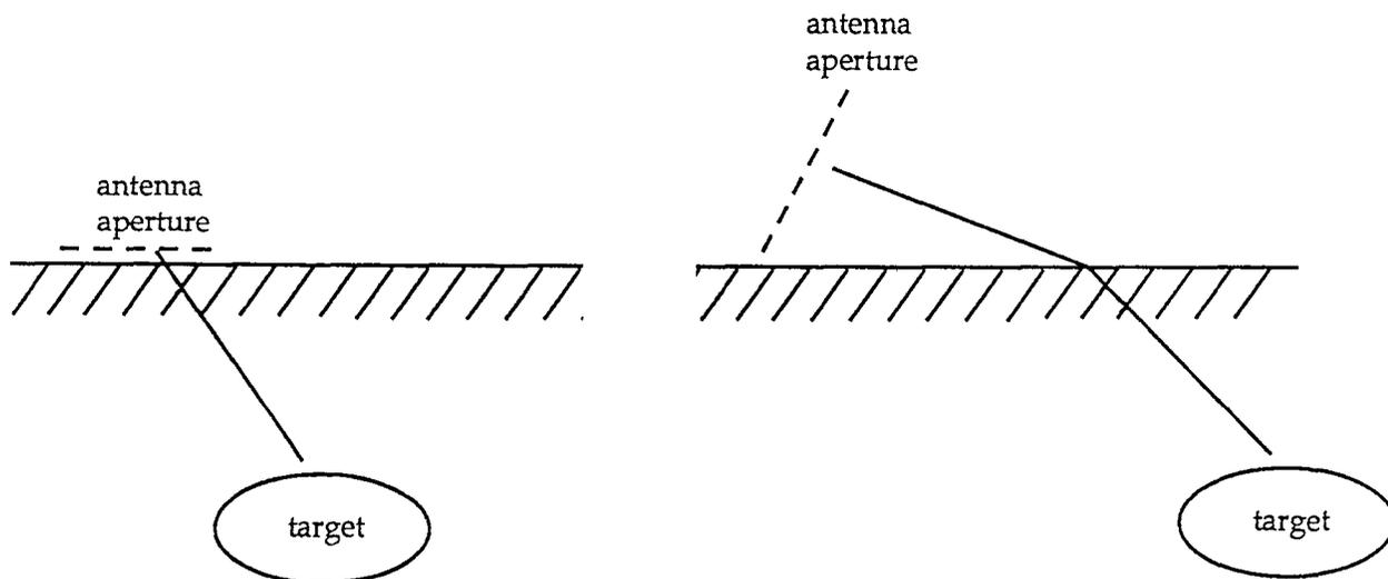
Fig. 1.2 Antenna Apertures At or Above the Earth Surface
