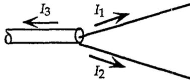
A. Unbalanced connection (two TEM-like modes on exterior).
