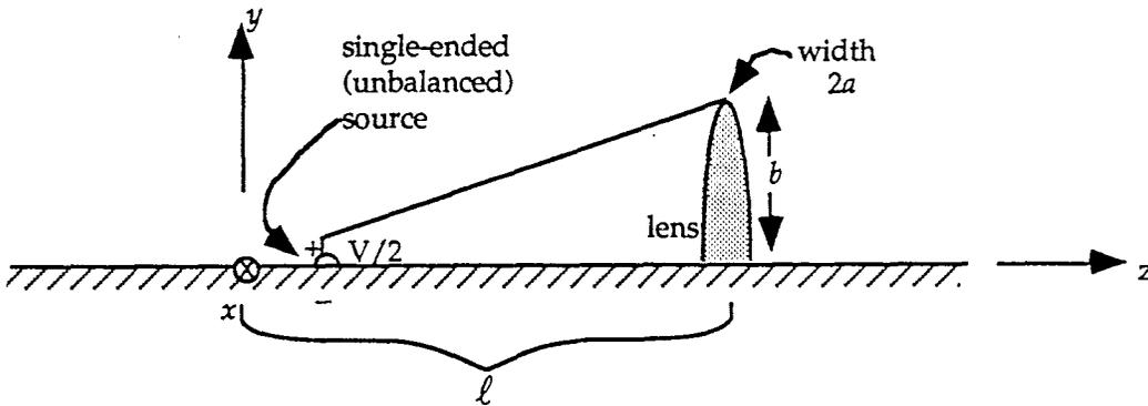
C. Flat-plate cone with ground plane.
