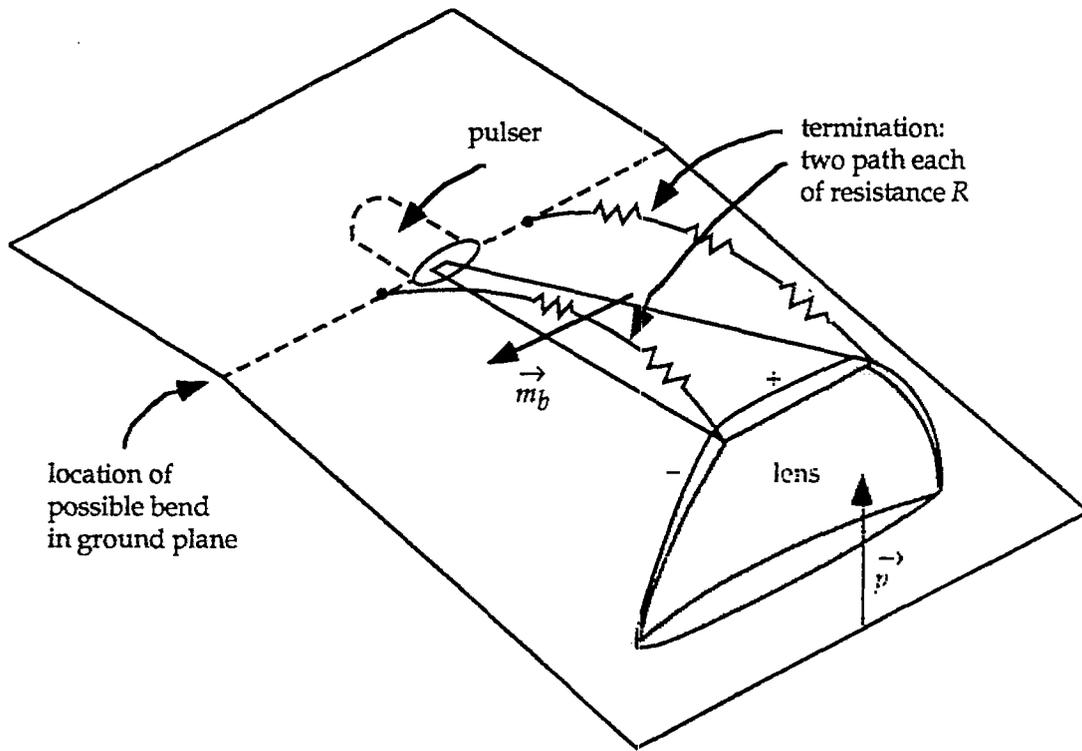
Fig. 3.1 TEM Horn and Lens (Lens IRA) With One Flat-Plate Cone, Ground Plane, and Termination to Location Behind Horn.
