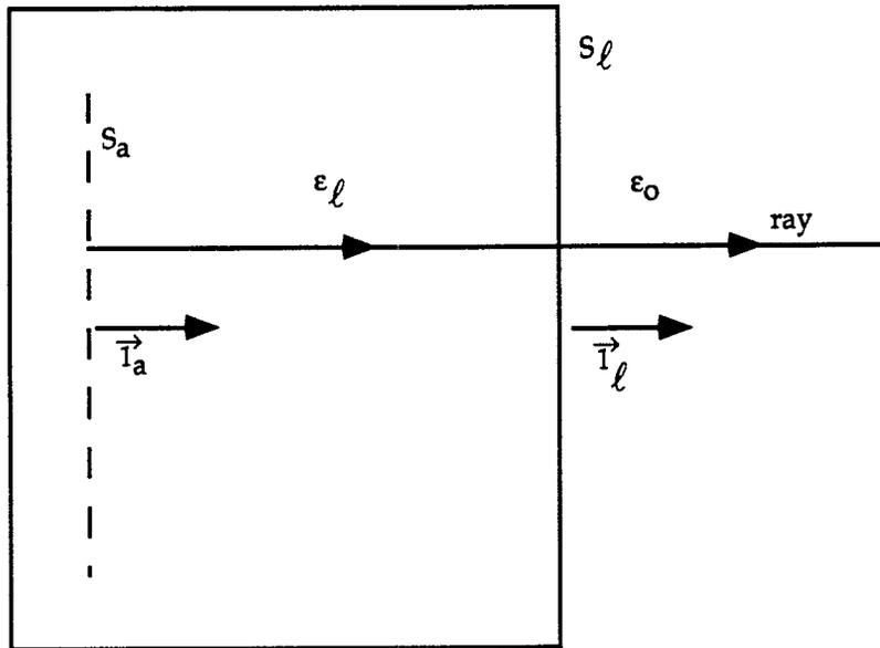
A. Normal incidence on lens surface: rays straight
