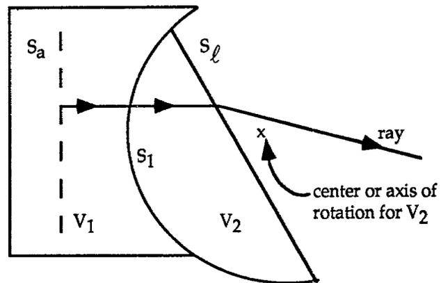
B. Rays bent: sliding contact of two lens parts at  $S_1$
