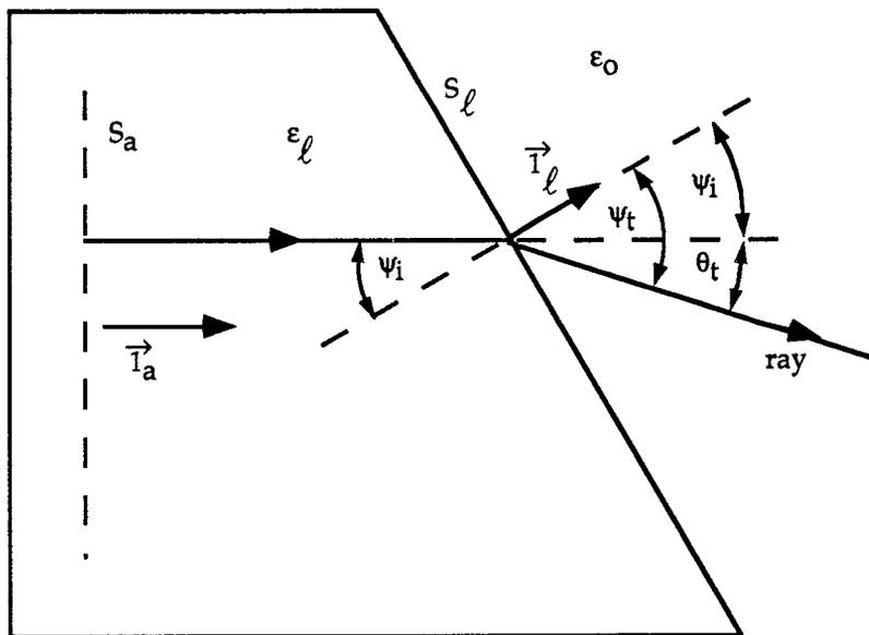
B. Oblique incidence on lens surface: rays straight
