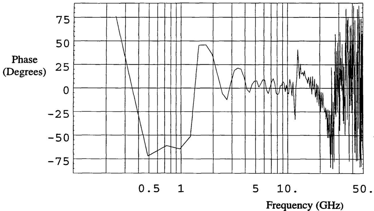
Figure 4.6. Frequency domain  $H(f)$ , just after taking the square root, magnitude (top) and phase (bottom). Note that the phase is essentially flat at the mid-band.
