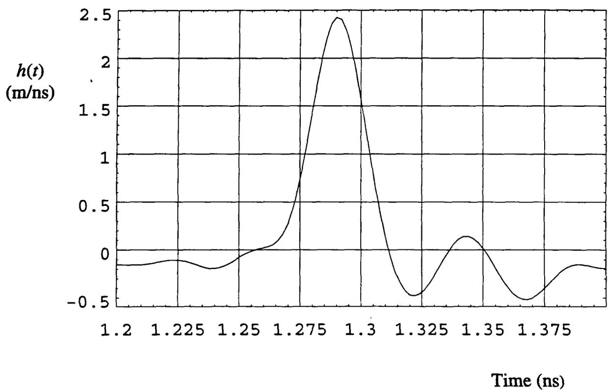
Figure 4.7 Boresight  $h(t)$ , entire waveform (top) and a closeup of the impulse (bottom).
