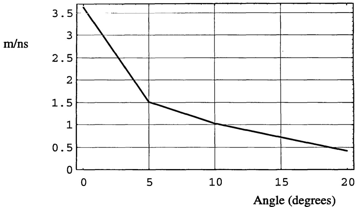
Figure 9.1. Gain of the 23 cm (9-inch) reflector IRA plotted as a function of angle off-boresight in the E-plane (top) and in the H-plane (bottom). Here gain is used in the peak  $h(t)$  sense, with perfect step excitation.
