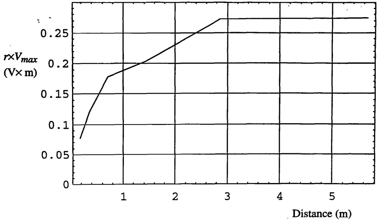
Figure 5.6. A check on the  $1/r$  dependence of the measurement. Based on this, measurements over 3 m are in the far field.
