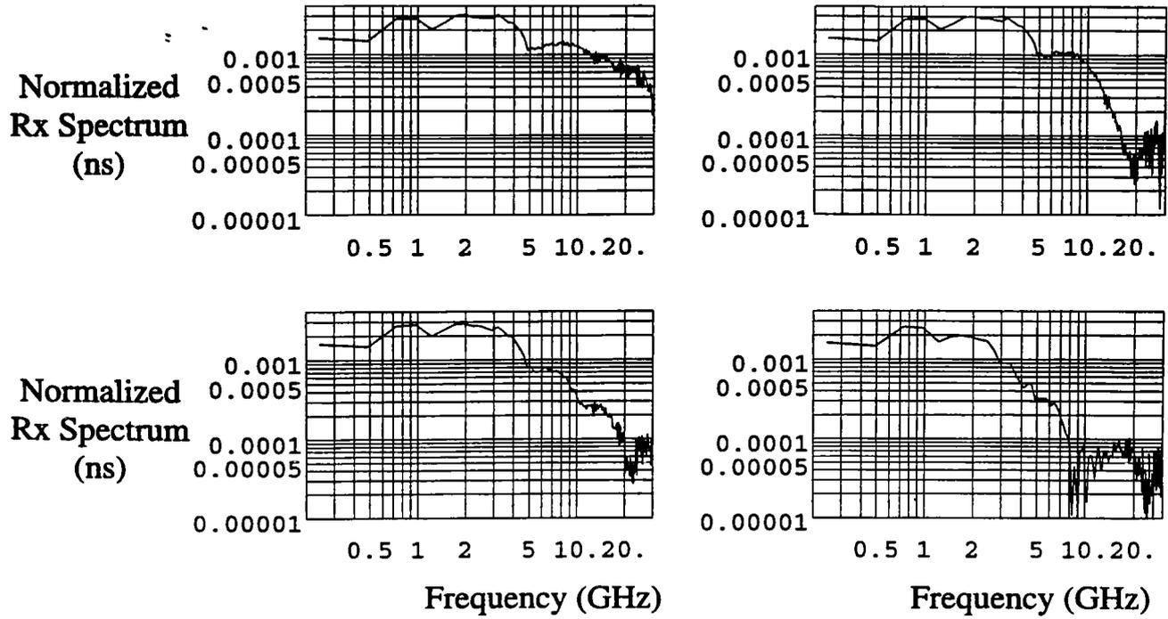
Figure 8.5 (b). H-Plane received voltage, after filtering and normalization, in the frequency domain. Waveforms are at 0, 5, 10, and 20 degrees off boresight.
