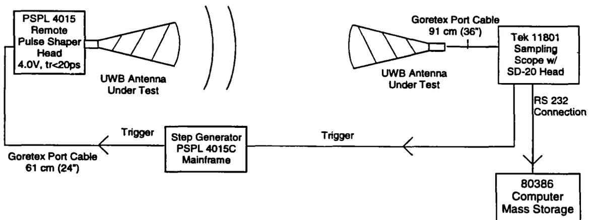
Figure 3.1. The experimental test configuration.
