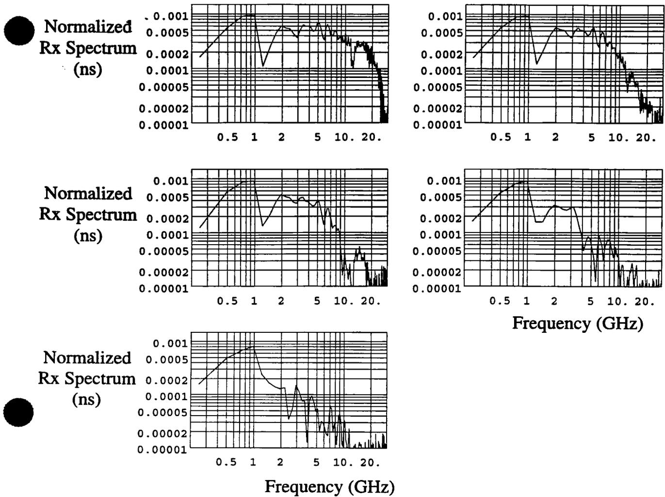
Figure 4.5 (a). E-Plane received voltage, after filtering and normalization, in the frequency domain. Waveforms are at 0, 5, 10, 20 and 40 degrees off boresight.
