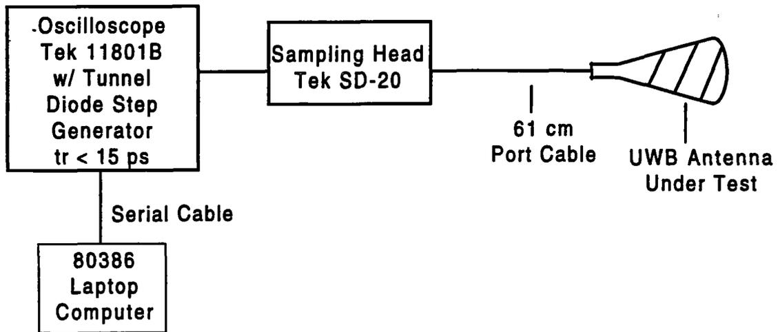
Figure 5.3. Experimental configuration for TDR measurements.
