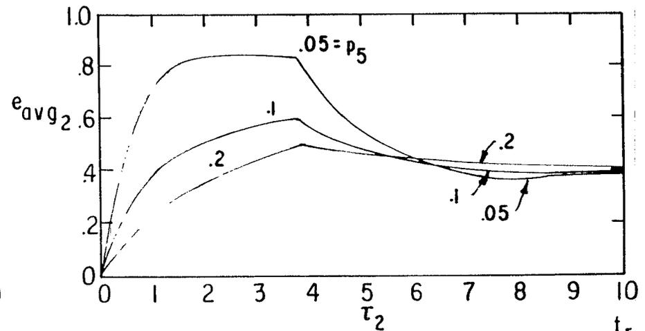
D.  $e_{avg_2}$  VS  $\tau_2$  WITH  $p_5$  AS A PARAMETER:  $\frac{t_{r1}}{t_2} = 1$
