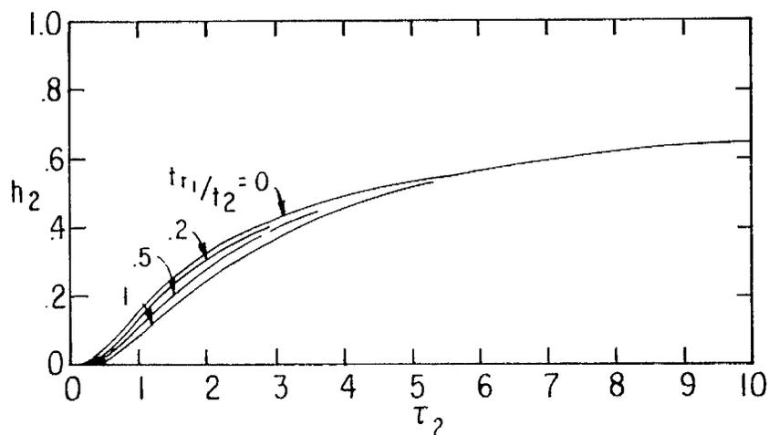
C.  $h_2$  VS  $\tau_2$  WITH  $t_{r1}/t_2$  AS A PARAMETER:  $\frac{\sigma_1}{\sigma_2} = 1$
