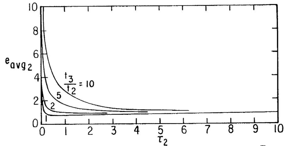
B.  $e_{avg2}$  VS  $\tau_2$  WITH  $t_3/t_2$  AS A PARAMETER:  $\frac{\sigma_1}{\sigma_2} = .1$
