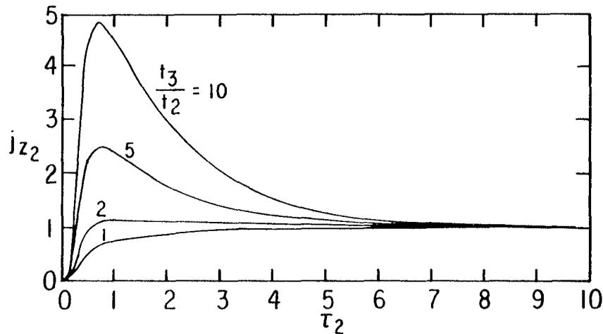
A.  $j_{z2}$  VS  $\tau_2$  WITH  $t_3/t_2$  AS A PARAMETER:  $\frac{\sigma_1}{\sigma_2} = 0$
