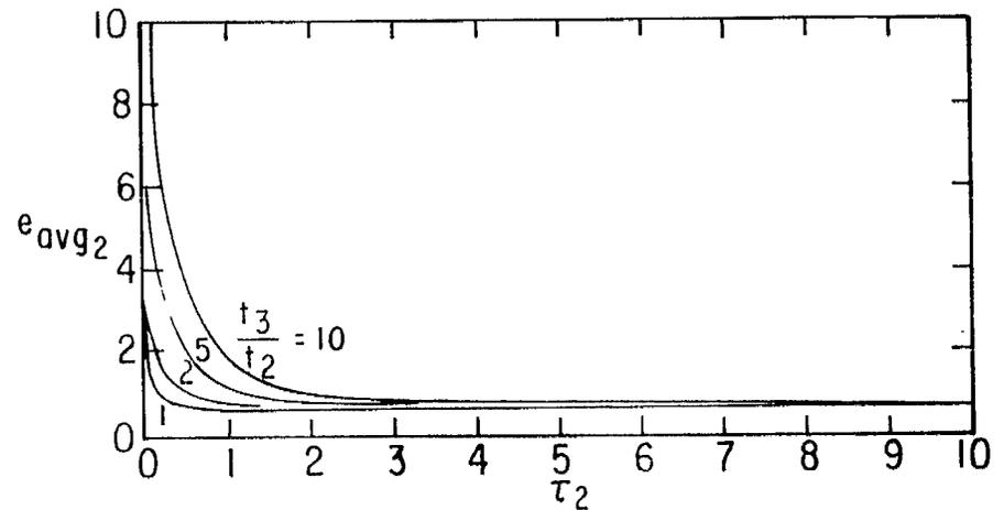
D.  $e_{avg2}$  VS  $\tau_2$  WITH  $t_3/t_2$  AS A PARAMETER:  $\frac{\sigma_1}{\sigma_2} = 10$
