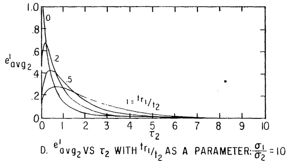
FIGURE 8. AVERAGE VERTICAL ELECTRIC PULSE SHAPE ON TRANSMISSION LINE:  $\epsilon_{r1} = 1$ ,  $\epsilon_{r2} = 10$ ,  $p_5 = 0$
