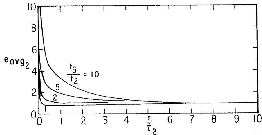
A.  $e_{avg2}$  VS  $\tau_2$  WITH  $t_3/t_2$  AS A PARAMETER:  $\frac{\sigma_1}{\sigma_2} = 0$
