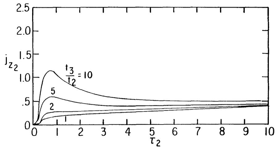
$j_{z2}$  VS  $\tau_2$  WITH  $t_3/t_2$  AS A PARAMETER:  $\frac{\sigma_1}{\sigma_2} = 10$
