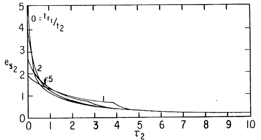
B.  $e_{s2}$  VS  $\tau_2$  WITH  $t_{r1}/t_2$  AS A PARAMETER:  $\frac{\sigma_1}{\sigma_2} = .1$
