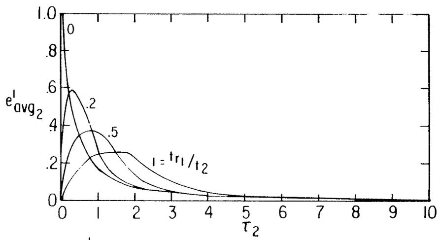
C.  $e'_{avg2}$  VS  $\tau_2$  WITH  $t_{r1}/t_2$  AS A PARAMETER:  $\frac{\sigma_1}{\sigma_2} = 1$
