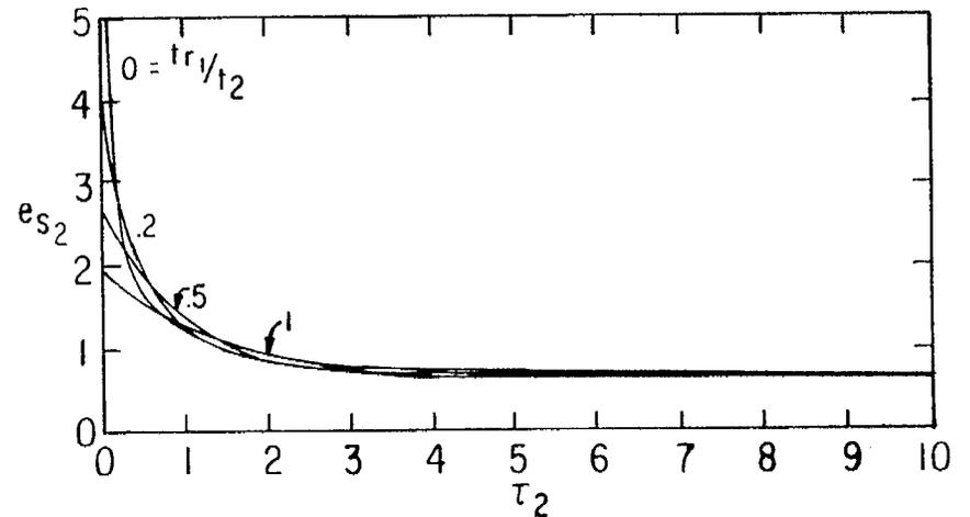
D.  $e_{s2}$  VS  $\tau_2$  WITH  $t_{r1}/t_2$  AS A PARAMETER:  $\frac{\sigma_1}{\sigma_2} = 10$
