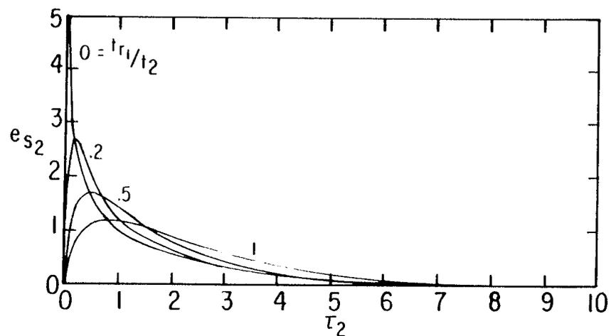
A.  $e_{s2}$  VS  $\tau_2$  WITH  $t_{r1}/t_2$  AS A PARAMETER:  $\frac{\sigma_1}{\sigma_2} = 0$
