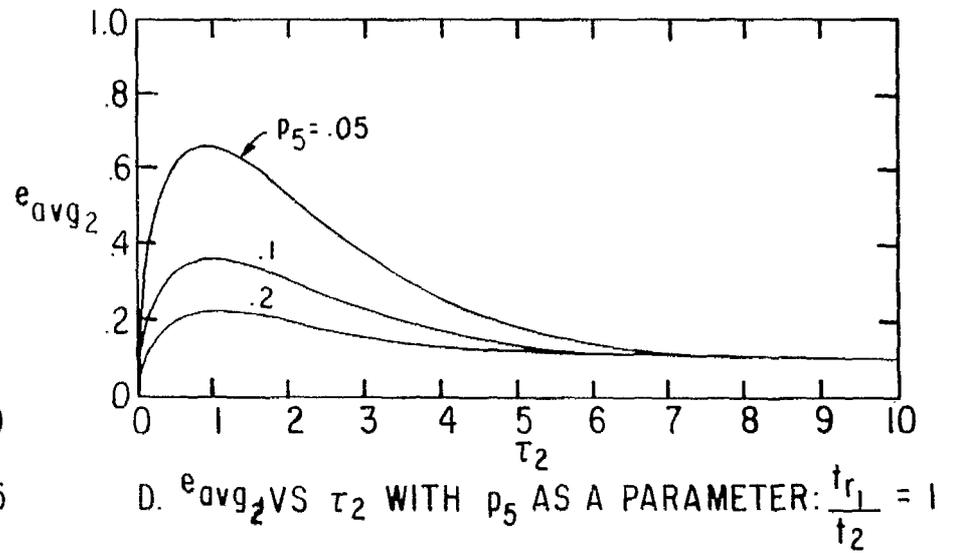
FIGURE 14. AVERAGE VERTICAL ELECTRIC FIELD PULSE SHAPE ON TRANSMISSION LINE:  $\frac{\sigma_1}{\sigma_2} = 0, \epsilon_{r1} = 1$
