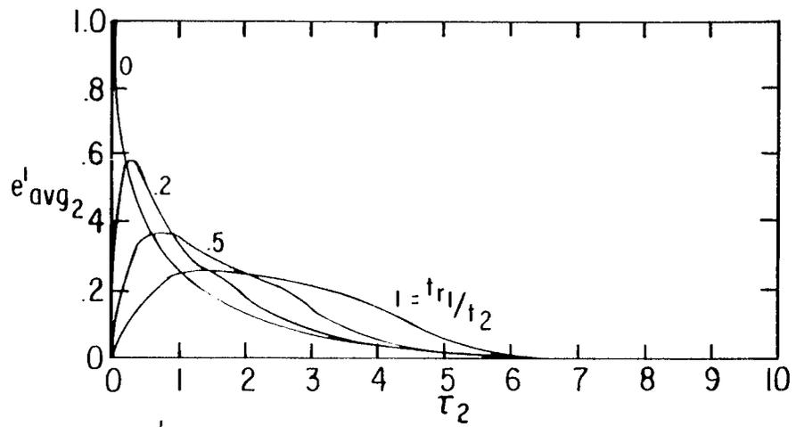
A.  $e'_{avg2}$  VS  $\tau_2$  WITH  $t_{r1}/t_2$  AS A PARAMETER:  $\frac{\sigma_1}{\sigma_2} = 0$
