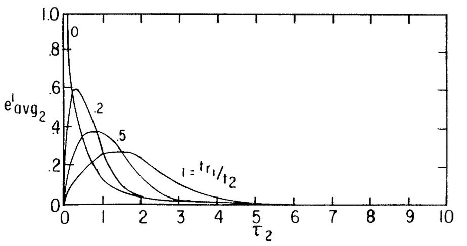
D.  $e'_{avg2}$  VS  $\tau_2$  WITH  $t_{r1}/t_2$  AS A PARAMETER:  $\frac{\sigma_1}{\sigma_2} = 10$
