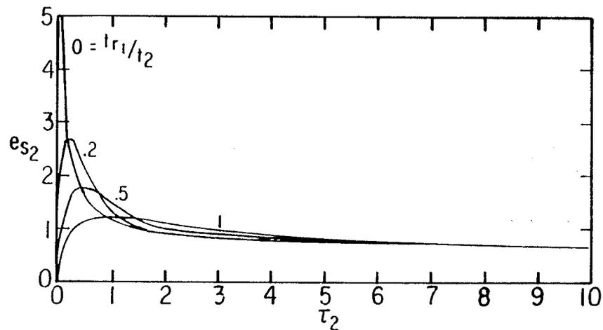
D.  $e_{s2}$  VS  $\tau_2$  WITH  $t_{r1}/t_2$  AS A PARAMETER:  $\frac{\sigma_1}{\sigma_2} = 10$
