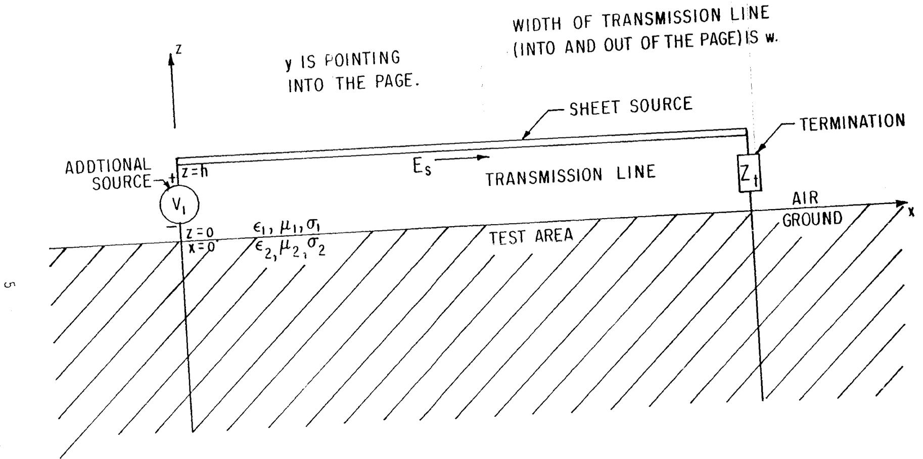
FIGURE 1 THE DISTRIBUTED - SOURCE, PLANAR, UNIFORM SURFACE TRANSMISSION LINE
