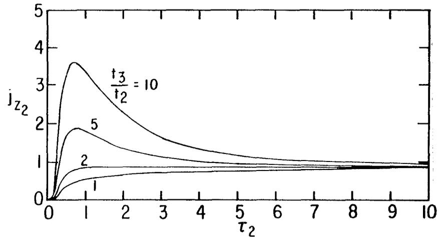
B.  $j_{z2}$  VS  $\tau_2$  WITH  $t_3/t_2$  AS A PARAMETER:  $\frac{\sigma_1}{\sigma_2} = .1$
