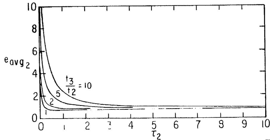
C.  $e_{avg2}$  VS  $\tau_2$  WITH  $t_3/t_2$  AS A PARAMETER:  $\frac{\sigma_1}{\sigma_2} = 1$
