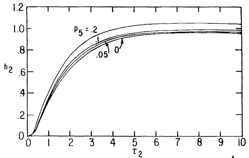
B.  $h_2$  VS  $\tau_2$  WITH  $p_5$  AS A PARAMETER:  $\frac{t_{r1}}{t_2} = .2$
