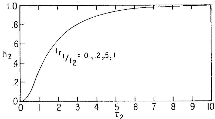
A.  $h_2$  VS  $\tau_2$  WITH  $t_{r1}/t_2$  AS A PARAMETER:  $\frac{\sigma_1}{\sigma_2} = 0$
