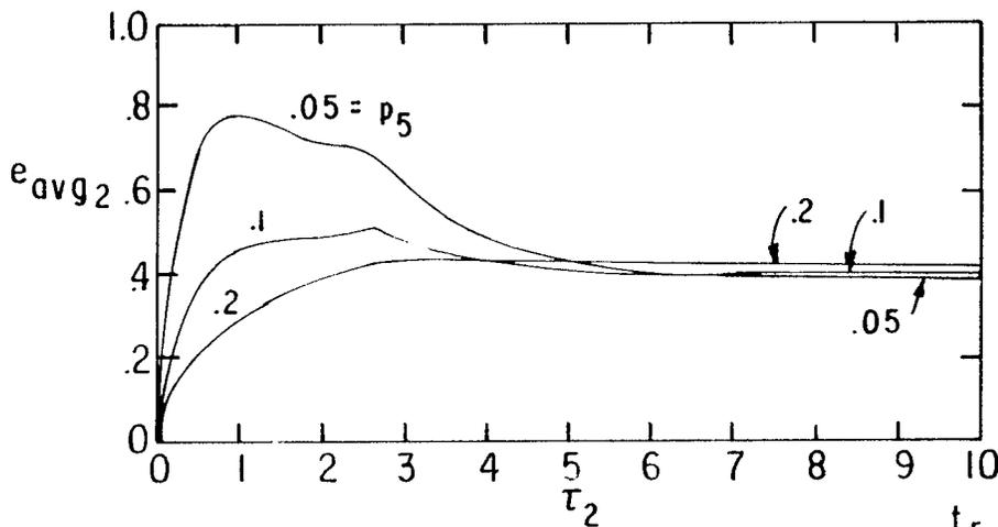
C.  $e_{avg_2}$  VS  $\tau_2$  WITH  $p_5$  AS A PARAMETER:  $\frac{t_{r1}}{t_2} = .5$
