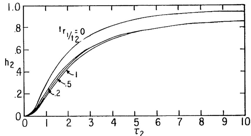
B.  $h_2$  VS  $\tau_2$  WITH  $t_{r1}/t_2$  AS A PARAMETER:  $\frac{\sigma_1}{\sigma_2} = .1$
