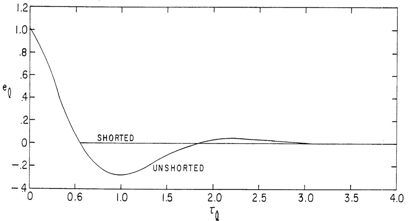
FIGURE 8. PULSE SHAPES FOR FINITE-LENGTH TRANSMISSION LINE WITH ONE CAPACITOR:  $\frac{t_0}{t_l} = .1$
