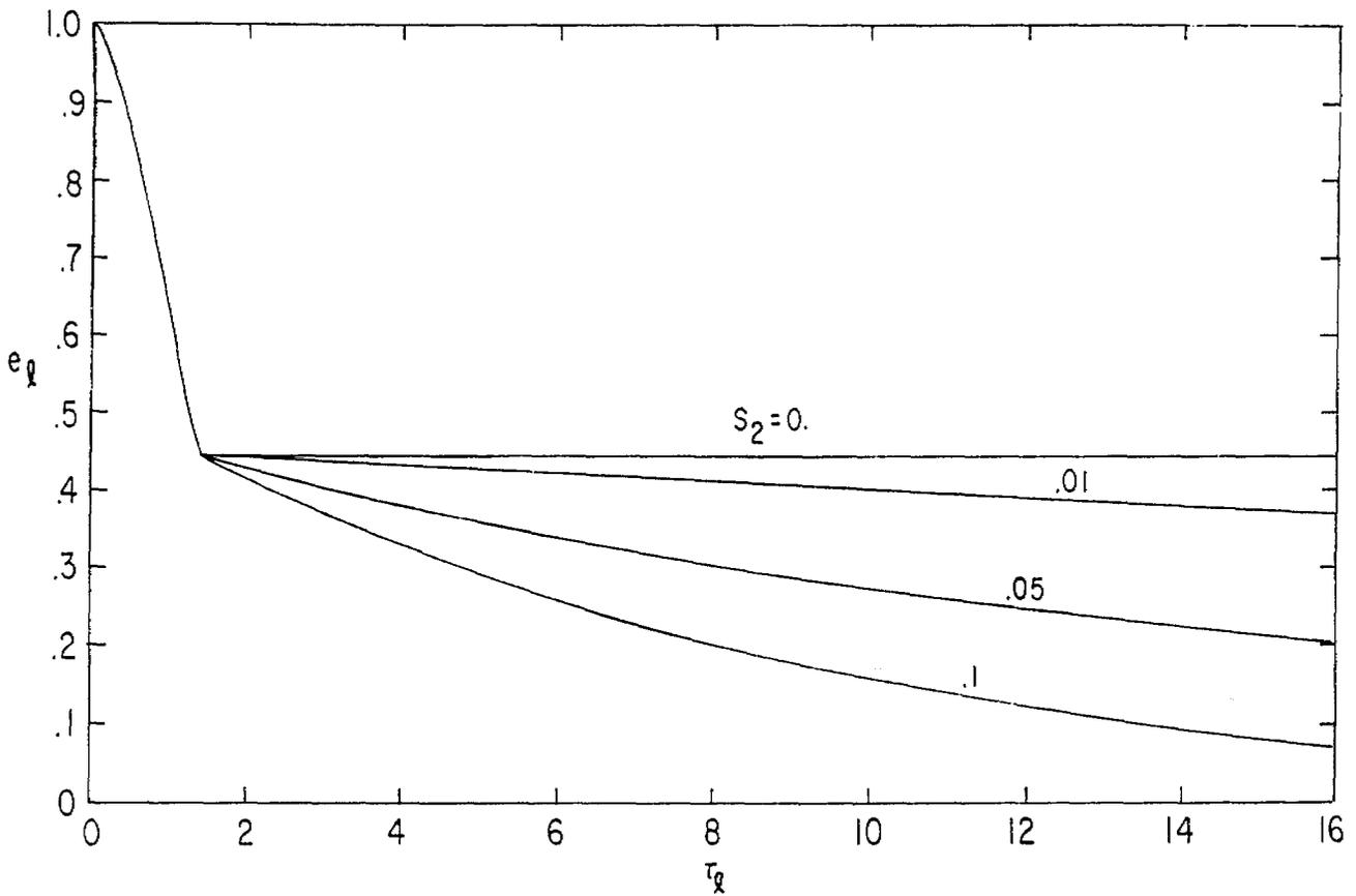
FIGURE 7. PULSE SHAPES FOR FINITE-LENGTH TRANSMISSION LINE WITH TWO CAPACITORS:  $\frac{t_0}{t_q} = 1.$ ,  $v_2 = .45$
