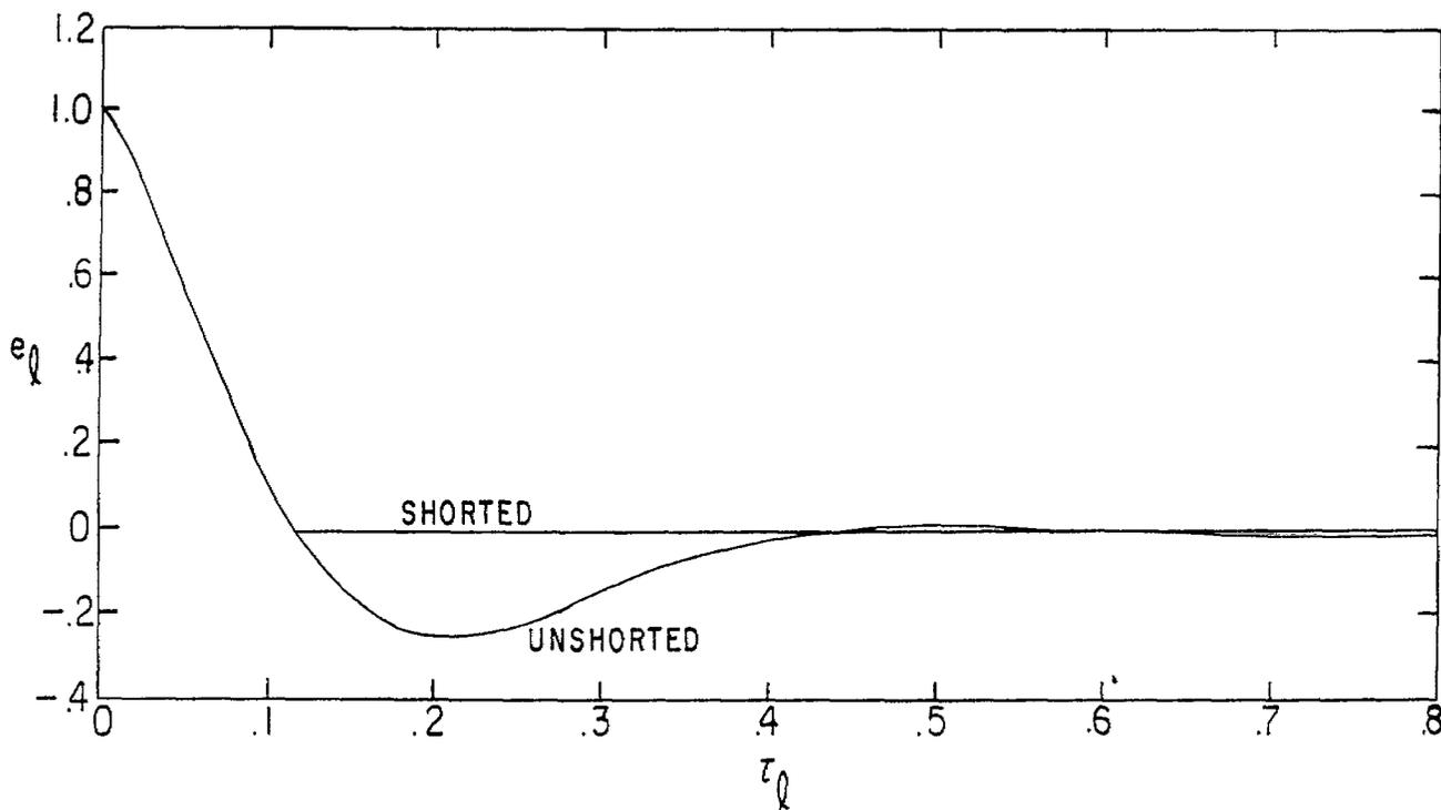
FIGURE II. PULSE SHAPES FOR FINITE-LENGTH TRANSMISSION LINE WITH ONE CAPACITOR:  $t_0/t_l = .01$
