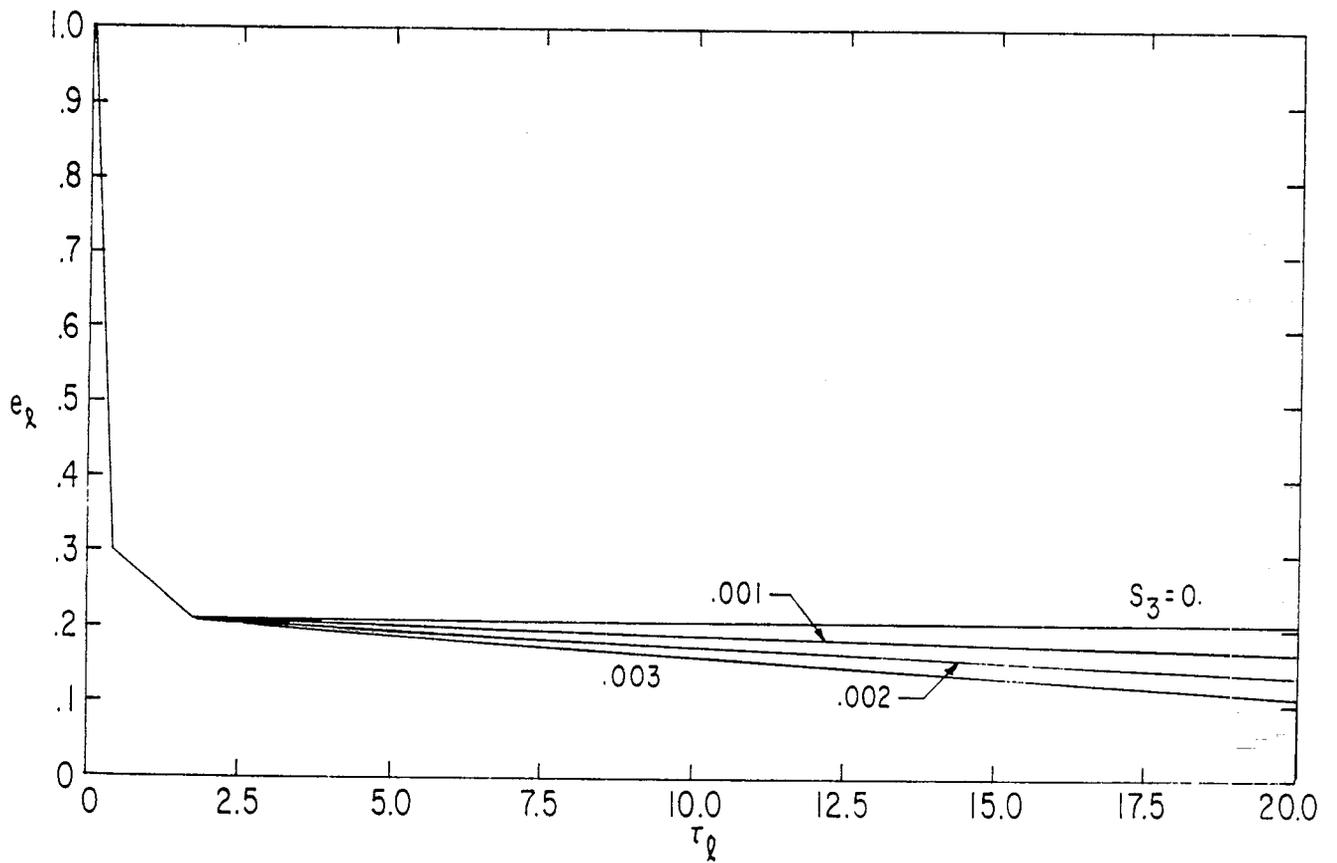
FIGURE 10. PULSE SHAPES FOR FINITE-LENGTH TRANSMISSION LINE WITH THREE CAPACITORS:  $\frac{\tau_0}{\tau_\lambda} = .1$ ,  $v_2 = .3$ ,  $S_2 = .03$ ,  $v_3 = .21$
