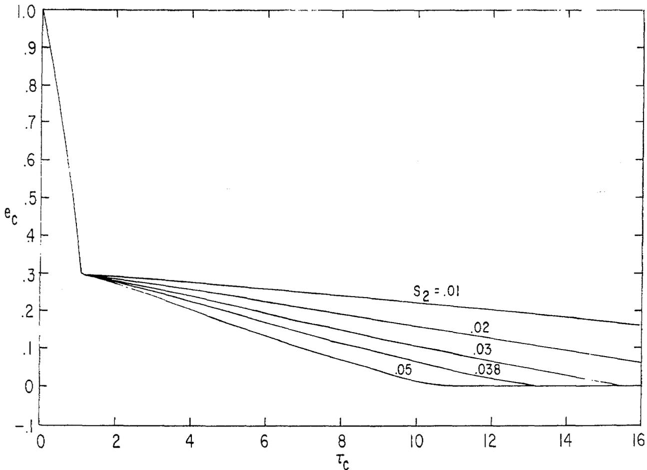
FIGURE 3. PULSE SHAPES FOR INFINITE-LENGTH TRANSMISSION LINE WITH TWO CAPACITORS:  $v_2 = .3$
