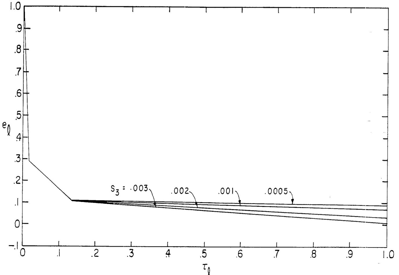
FIGURE 16. PULSE SHAPES FOR FINITE-LENGTH TRANSMISSION LINE WITH THREE CAPACITORS:  $t_0/t_0 = .001$ ,  $v_2 = .3$ ,  $S_2 = .034$ ,  $v_3 = .11$
