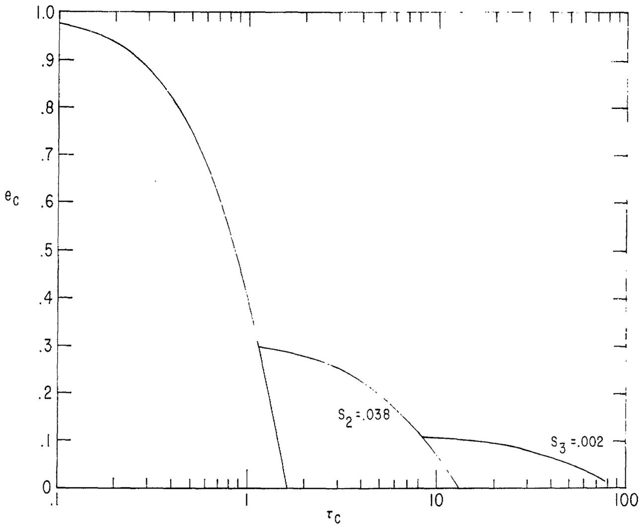
FIGURE 5. PULSE SHAPES FOR INFINITE-LENGTH TRANSMISSION LINE WITH VARYING NUMBER OF CAPACITORS
