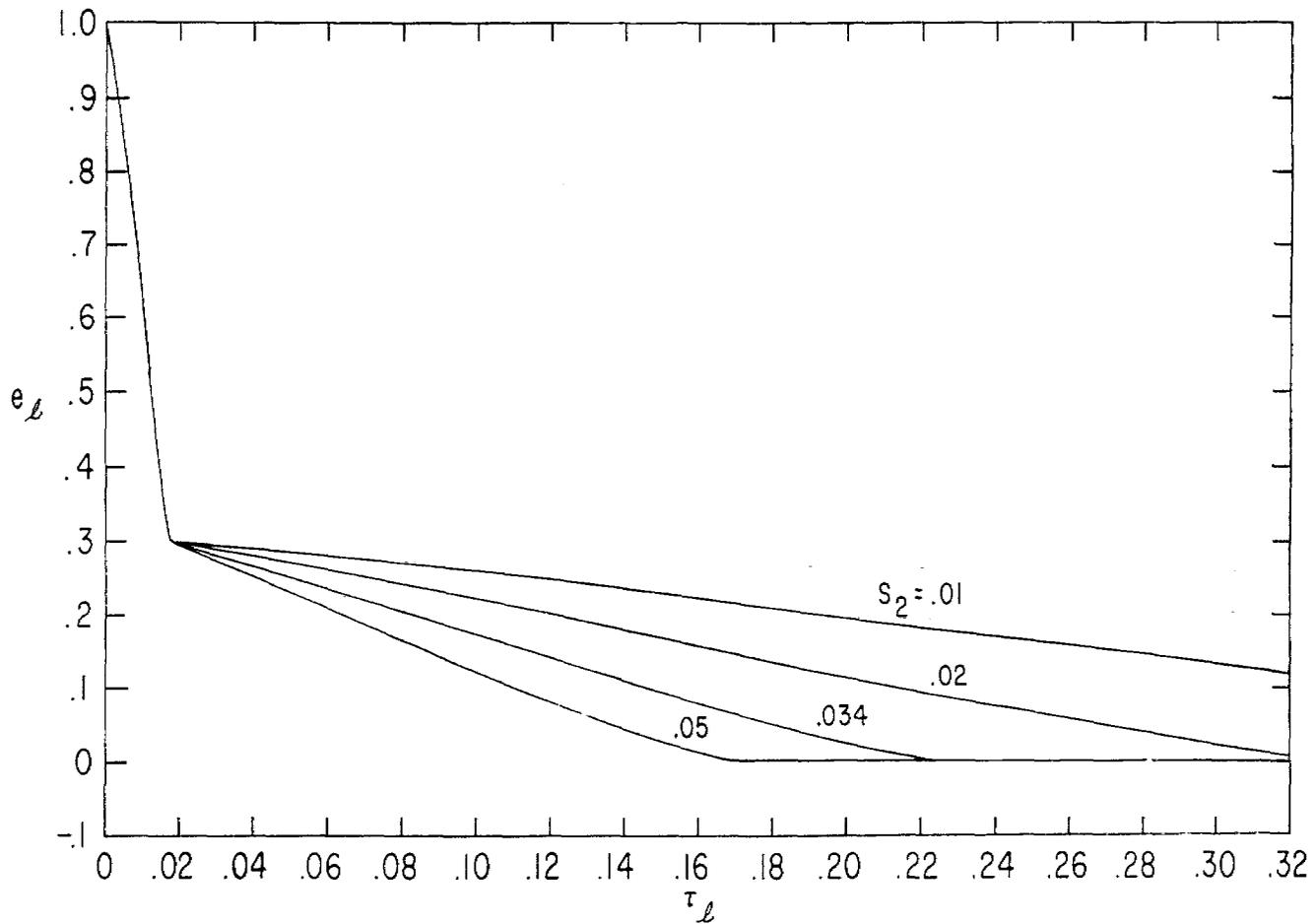
FIGURE 15. PULSE SHAPES FOR FINITE-LENGTH TRANSMISSION LINE WITH TWO CAPACITORS :  $\frac{t_0}{t_l} = .001$ ,  $v_2 = .3$
