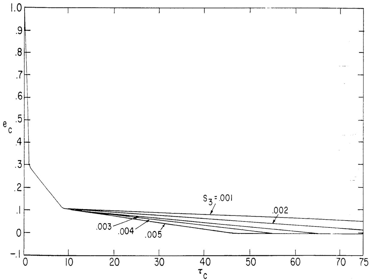
FIGURE 4. PULSE SHAPES FOR INFINITE-LENGTH TRANSMISSION LINE WITH THREE CAPACITORS:  $v_2 = .3$ ,  $S_2 = .038$ ,  $v_3 = .11$
