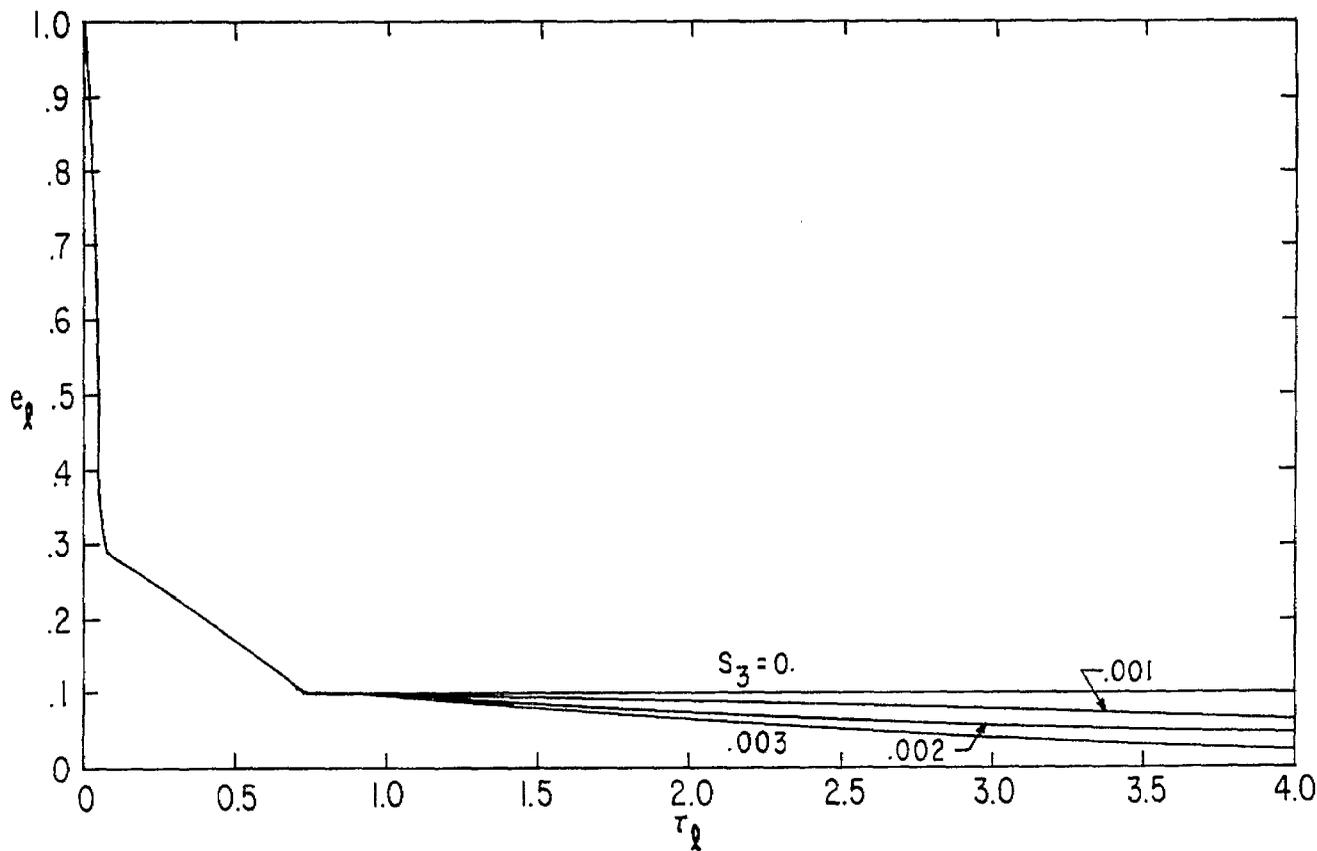
FIGURE 13. PULSE SHAPES FOR FINITE-LENGTH TRANSMISSION LINE WITH THREE CAPACITORS:  $\frac{\tau_0}{\tau_g} = .01$ ,  $v_2 = .3$ ,  $S_2 = .03$ ,  $v_3 = .1$
