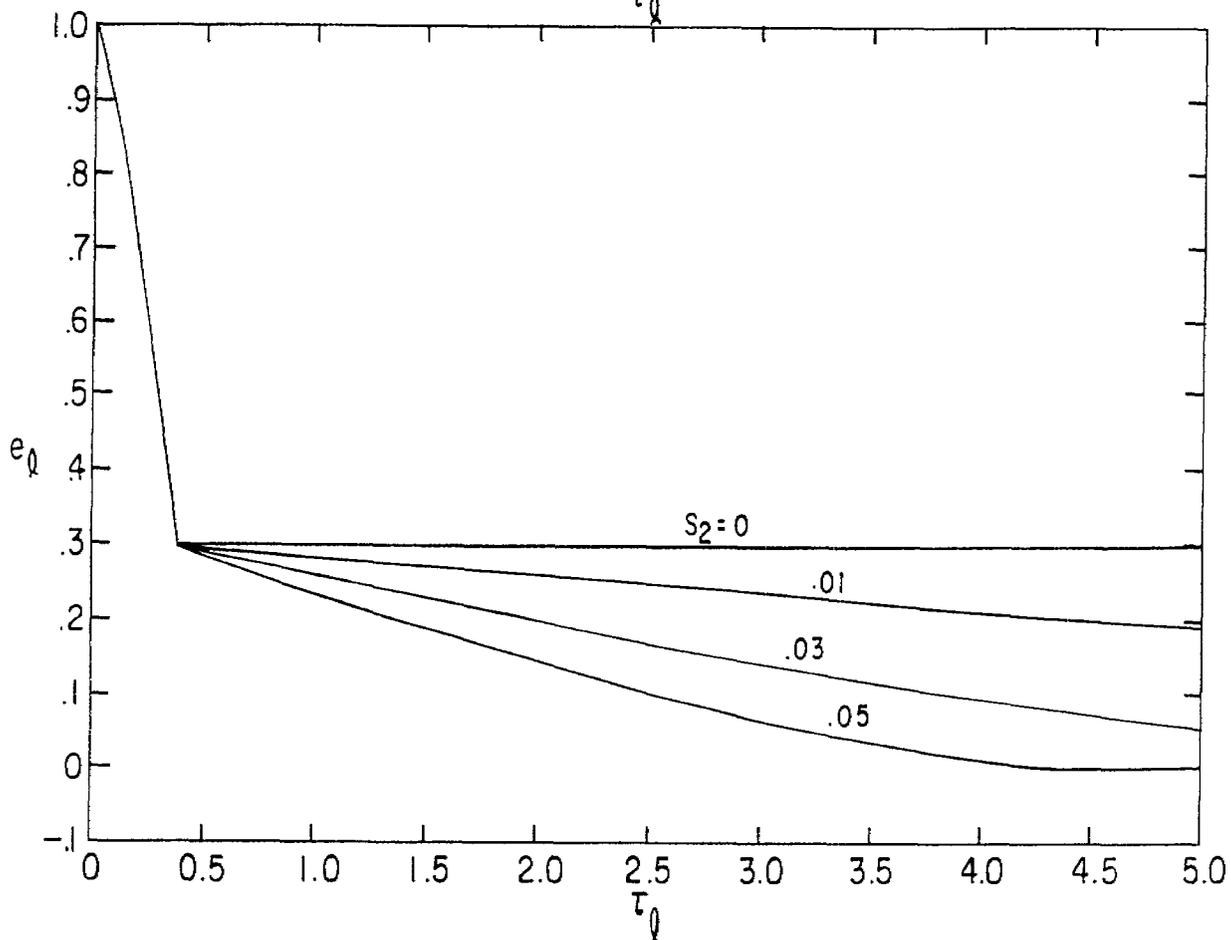
FIGURE 9. PULSE SHAPES FOR FINITE-LENGTH TRANSMISSION LINE WITH TWO CAPACITORS:  $t_0/t_1 = .1, v_2 = .3$
