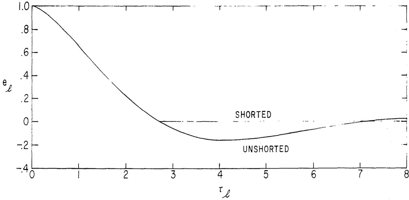
FIGURE 6. PULSE SHAPES FOR FINITE - LENGTH TRANSMISSION LINE WITH ONE CAPACITOR :  $\frac{t_0}{t_l} = 1$ .
